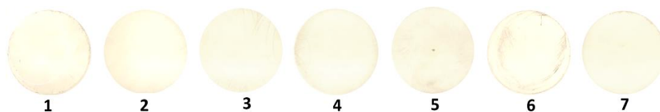
Fig. S2 Anhydride-based epoxy sample (TCES) was cut into 3mm thick discs.
