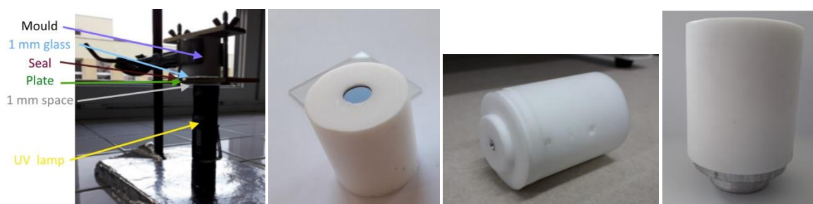
Fig. S3 The schema of the experimental arrangement of the photo-induced RICFP by UV light. In the first picture, the reaction systems were triggered by UV light, which was passed through the thin SiO 2 glass plate fixed at the bottom of the mould. Next three pictures represent the Teflon cylindrical mould with three different bottom parts, i.e. the glassy plate, the Teflon plate with an integrated metal part in the middle used for a soldering iron, and the Al spacer used for a heating plate.
