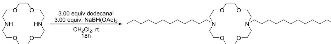
**Didodecyl diaza(18-crown-6) (LEC<sub>12</sub>).** To a stirred solution of 100.0 mg (0.38 mmol, 1.00 equiv.) 1,4,10,13-tetraoxa-7,16-diazacyclooctadecane in 3.80 mL  $CH_2Cl_2$  was added 0.25 mL (1.14 mmol,
