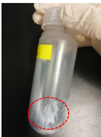
Fig. S7 The photo of damaged \text{Ti}_2\text{CT}_x MXene by oxidation.
