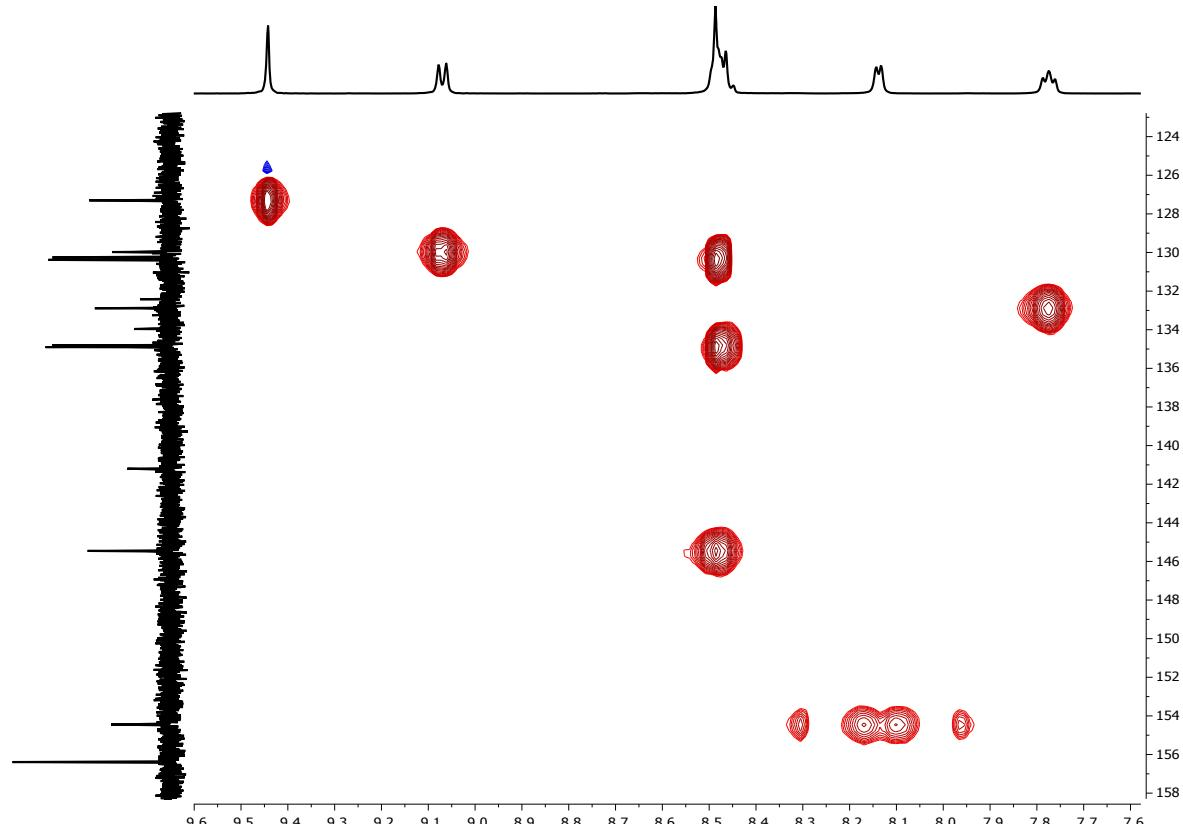
Fig. S8. HMQC (500 MHz  $^1\text{H}$ , 126 MHz  $^{13}\text{C}$ , TFA-d 298 K) spectrum of  $[\text{Rh}(\mathbf{1})_2]\text{Cl}_3$  prepared from  $\text{RhCl}_3 \cdot 3\text{H}_2\text{O}$ . Chemical shifts in  $\delta/\text{ppm}$ .
