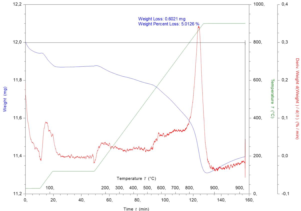
Fig. S25. TGA curve for NP-[Rh(1)<sub>2</sub>]<sup>3+</sup> prepared from RhCl<sub>3</sub>.3H<sub>2</sub>O: Weight against time and temperature (blue), derivative of weight change against time (red).
