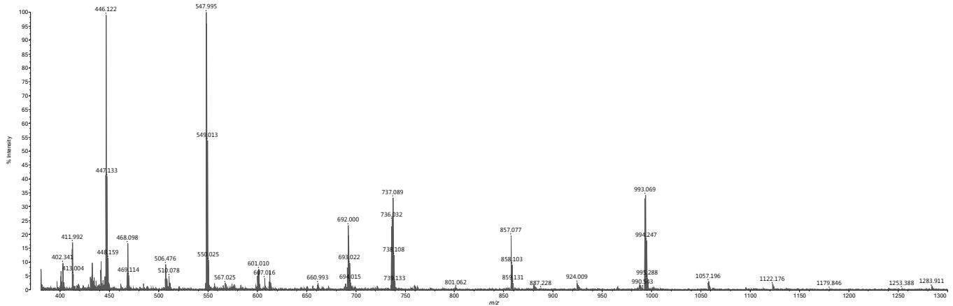
Fig. S35. MALDI mass spectrum (with CHCA matrix) of  $[\text{Rh}(\mathbf{5})_2]\text{[PF}_6\text{]}_3$
