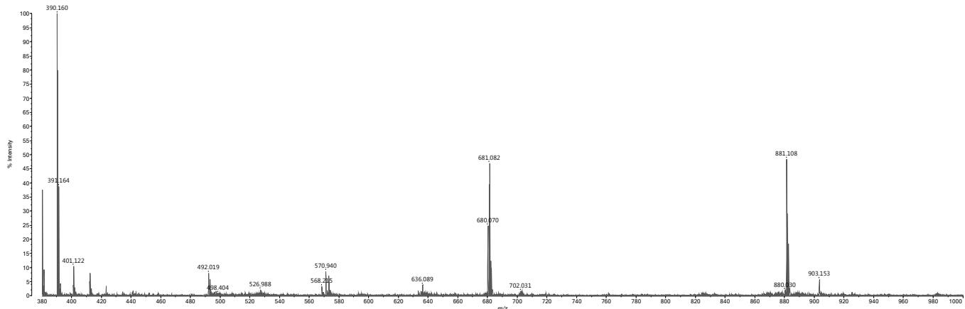
Fig. S4. MALDI mass spectrum (with CHCA matrix) of  $[\text{Rh}(\mathbf{1})_2]\text{Cl}_3$  prepared from  $\text{RhCl}_3 \cdot 3\text{H}_2\text{O}$ .
