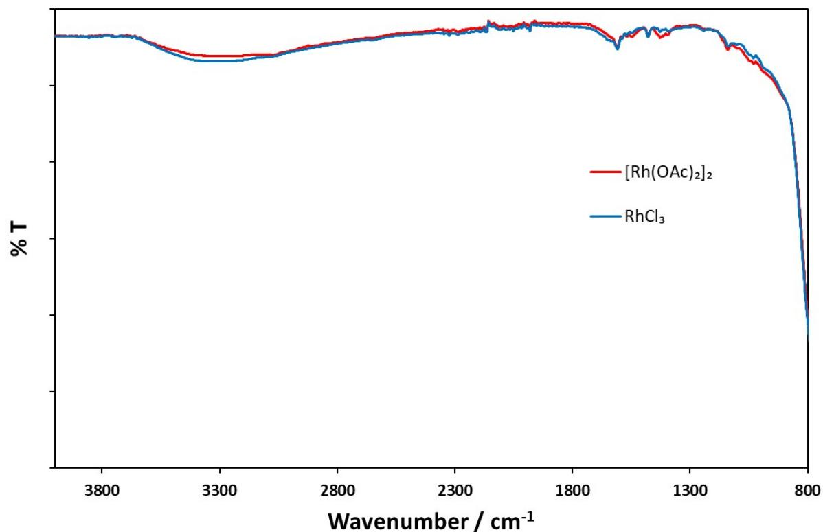
Fig. S22. Solid-state IR spectra of NP-[Rh(**1**)<sub>2</sub>]<sup>3+</sup>, prepared from [Rh<sub>2</sub>(μ-OAc)<sub>4</sub>(H<sub>2</sub>O)<sub>2</sub>] (red) or RhCl<sub>3</sub>·3H<sub>2</sub>O (blue) following the procedures in the Experimental Section.
