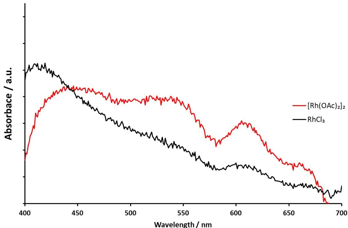
Fig. S23. Solid-state absorption spectra of NP-[Rh(**1**)<sub>2</sub>]<sup>3+</sup> prepared from [Rh<sub>2</sub>(μ-OAc)<sub>4</sub>(H<sub>2</sub>O)<sub>2</sub>] (red) or RhCl<sub>3</sub>·3H<sub>2</sub>O (black); The spectra are background-corrected using an NP reference.
