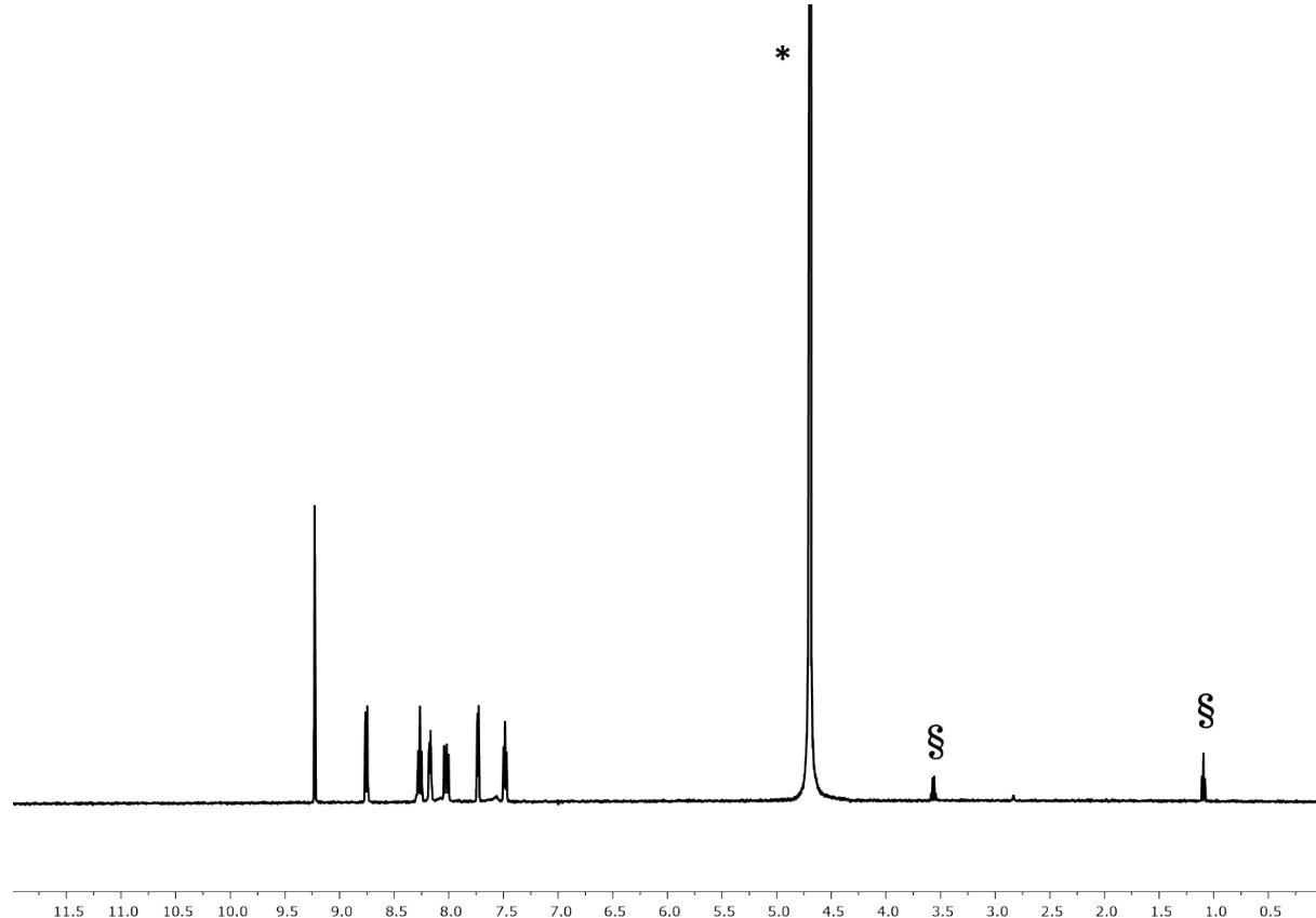
Fig. S2.  $^1\text{H}$  NMR (500 MHz,  $\text{D}_2\text{O}$ , 298 K) spectrum of  $[\text{Rh}(\mathbf{1})_2]\text{Cl}_3$  prepared from  $[\text{Rh}_2(\mu\text{-OAc})_4(\text{H}_2\text{O})_2]$ , \* = HOD, § = residual EtOH. Chemical shifts in  $\delta/\text{ppm}$ .
