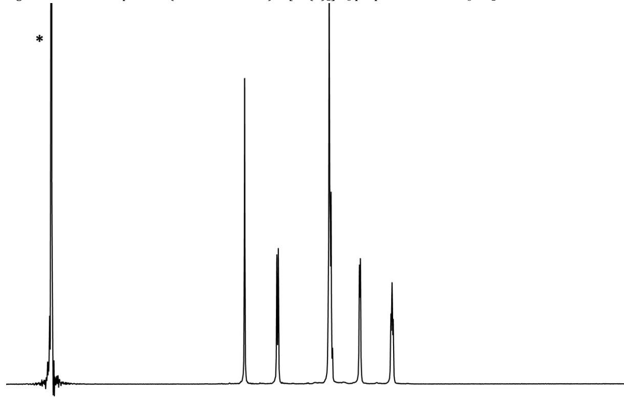
Fig. S5.  $^1\text{H}$  NMR (500 MHz, TFA-d 298 K) spectrum of  $[\text{Rh}(\mathbf{1})_2]\text{Cl}_3$  prepared from  $\text{RhCl}_3 \cdot 3\text{H}_2\text{O}$ , \* = HOD. Chemical shifts in  $\delta/\text{ppm}$ .
