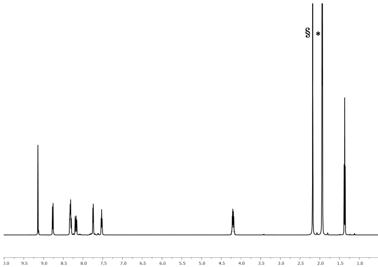
Fig. S14. <sup>1</sup>H NMR (500 MHz,  $\text{CD}_3\text{CN}$ , 298 K) spectrum of  $[\text{Rh}(\mathbf{5})_2]\text{[PF}_6\text{]}_3$ , \* =  $\text{CHD}_2\text{CN}$ , § = HOD. Chemical shifts in  $\delta/\text{ppm}$ .
