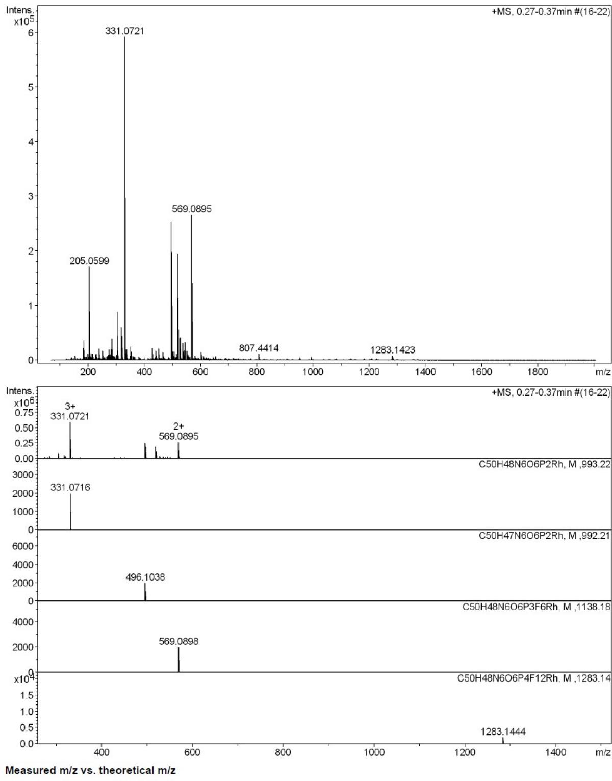
Fig. S33. High resolution electrospray mass spectrum of  $[\text{Rh}(\text{5})_2][\text{PF}_6]_3$  (MeCN, positive mode). Calculated spectra are shown in the lower four traces.
