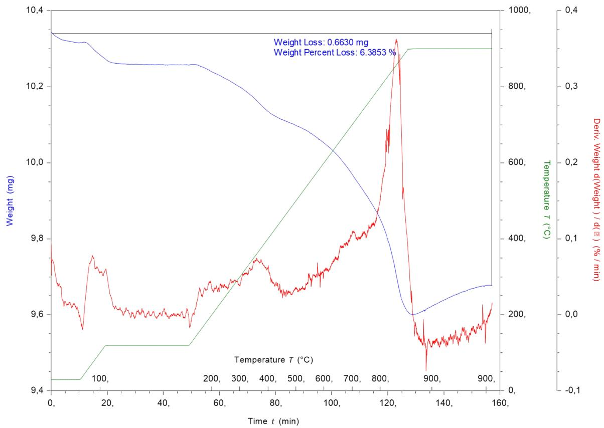
Fig. S24. TGA curve for NP-[Rh(1)<sub>2</sub>]<sup>3+</sup> prepared from [Rh<sub>2</sub>(μ-OAc)<sub>4</sub>(H<sub>2</sub>O)<sub>2</sub>]: Weight against time and temperature (blue), derivative of weight change against time (red).
