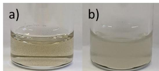
Fig. S3. a)  $[\text{Rh}(\mathbf{1})_2]\text{Cl}_3$  dissolved in concentrated  $\text{HNO}_3$  b)  $[\text{Rh}(\mathbf{1})_2]\text{Cl}_3$  dissolved in concentrated  $\text{HNO}_3$  after adding a drop of silver nitrate showing precipitation of  $\text{AgCl}$ .
