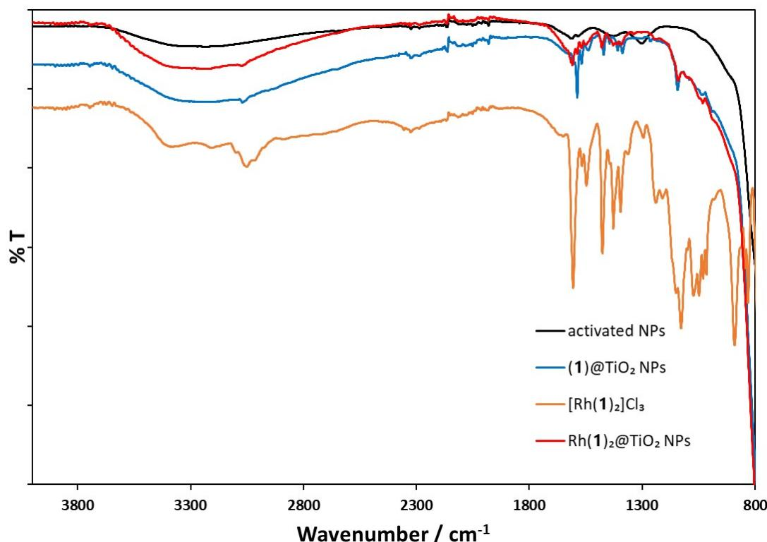
Fig. S29. Solid-state IR spectra of activated NPs (black),  $(\mathbf{1})@\text{TiO}_2$  NPs (blue),  $[\text{Rh}(\mathbf{1})_2]\text{Cl}_3$  (orange) and  $\text{Rh}(\mathbf{1})_2@\text{TiO}_2$  NPs (red) following the procedures in the Experimental Section.
