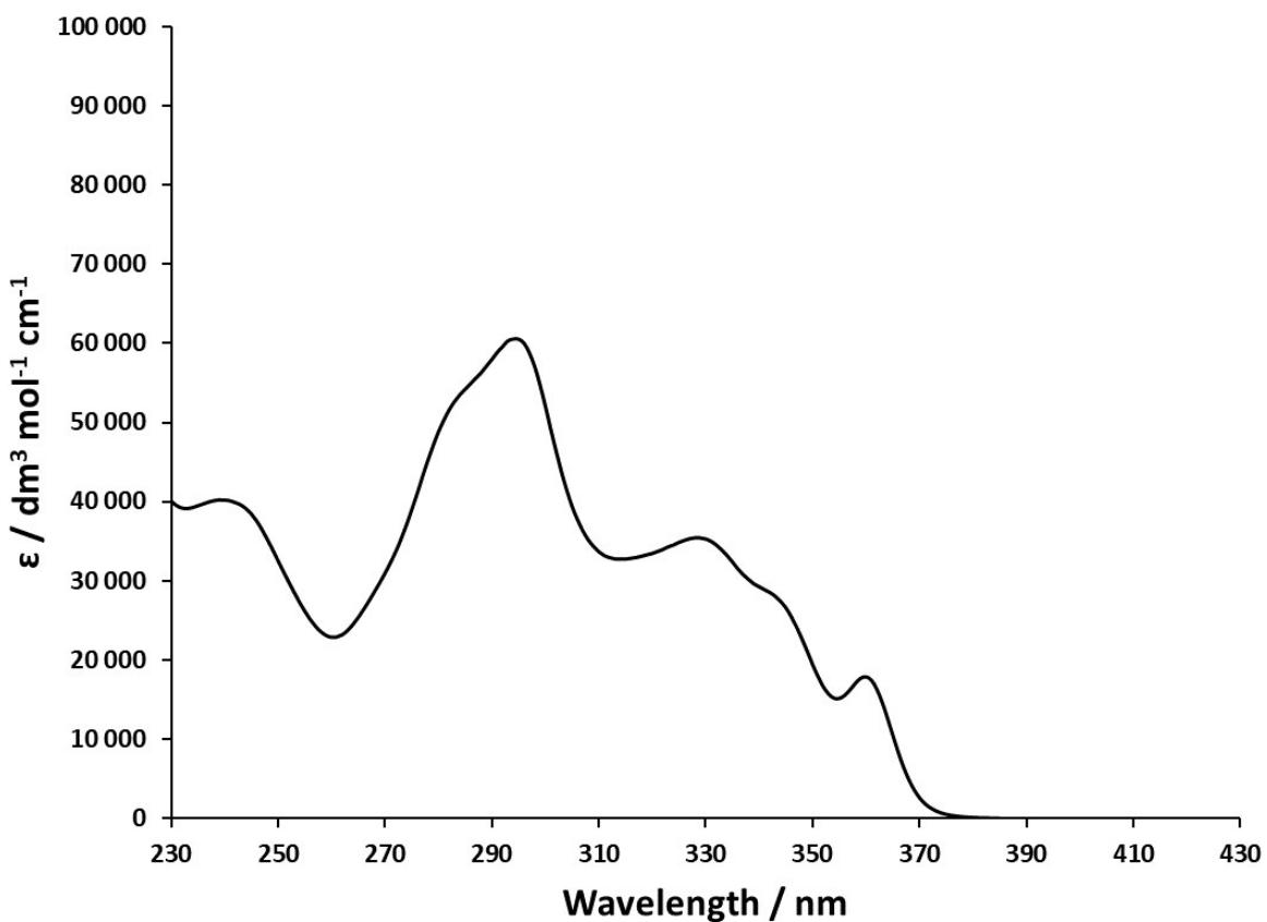
Fig. S20. Solution absorption spectra of  $[\text{Rh}(5)_2]\text{[PF}_6\text{]}_3$  ( $2.25 \times 10^{-5} \text{ mol dm}^{-3}$ ) in MeCN.
