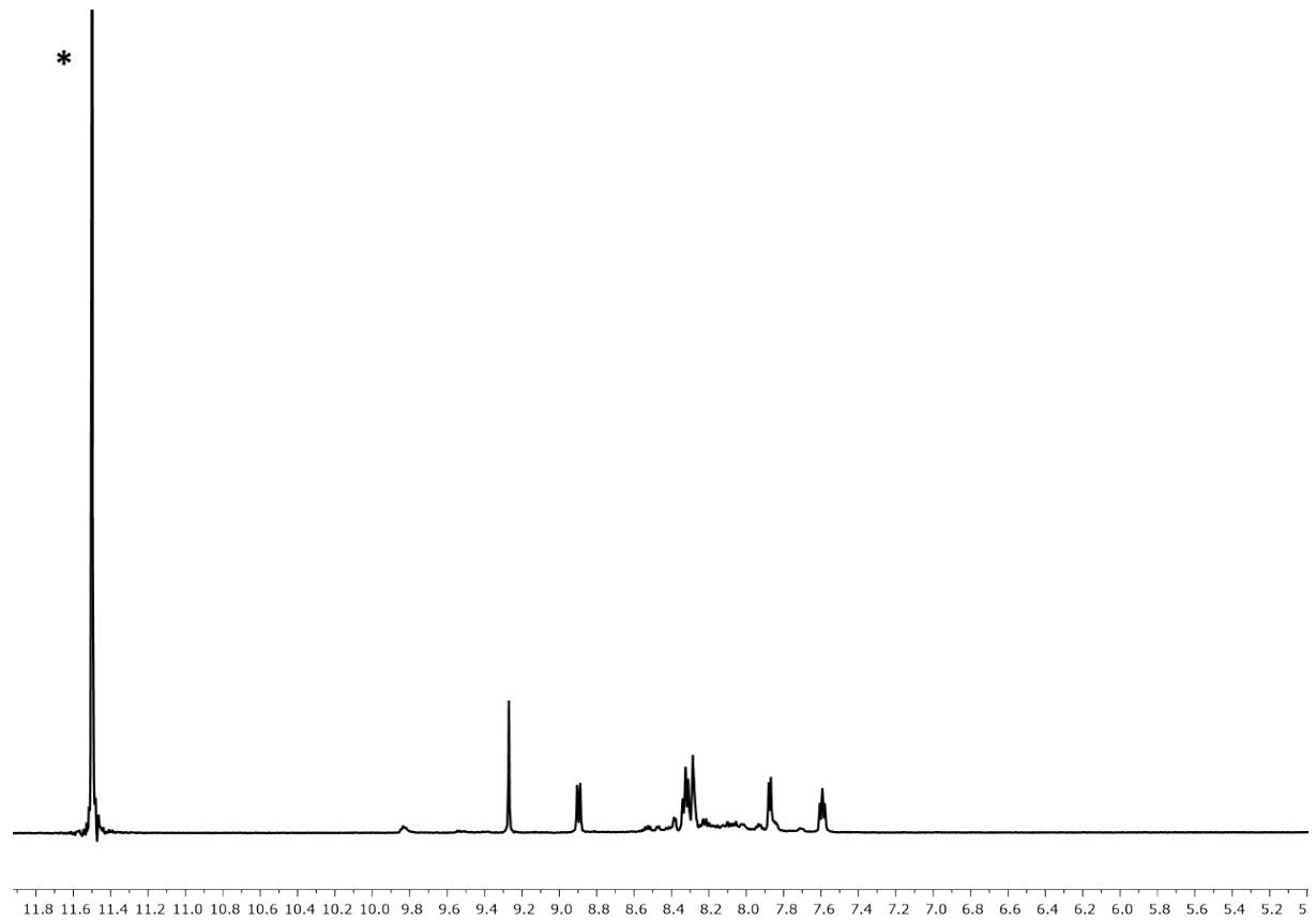
Fig. S10.  $^1\text{H}$  NMR (500 MHz, TFA-d, 298 K) spectrum of  $[\text{Rh}(\mathbf{1})_2]\text{Cl}_3$  prepared from  $[\text{Rh}_2(\mu\text{-OAc})_4(\text{H}_2\text{O})_2]$ , \* =  $\text{CF}_3\text{CO}_2\text{H}$ . Chemical shifts in  $\delta/\text{ppm}$ .
