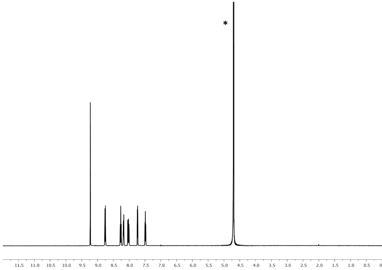
Fig. S36.  $^1\text{H}$  NMR (500 MHz,  $\text{D}_2\text{O}$ , 298 K) spectrum of  $[\text{Rh}(\mathbf{1})_2]\text{Cl}_3$  prepared from  $\text{RhCl}_3 \cdot 3\text{H}_2\text{O}$ , \* = HOD. Chemical shifts in  $\delta/\text{ppm}$ .
