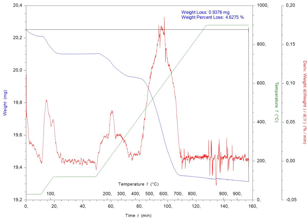
Fig. S31. TGA curve of (1)@TiO<sub>2</sub> NPs: Weight against time and temperature (blue), derivative of weight change against time (red).
