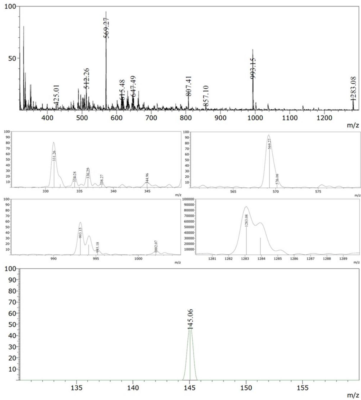
Fig. S32. Electrospray mass spectrum of  $[\text{Rh}(5)_2][\text{PF}_6]_3$  (MeCN). Positive mode in black, negative mode in green.
