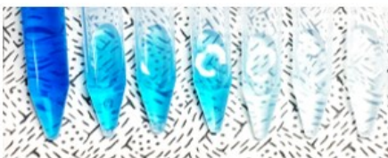
Fig. S2. Photographs of MB solutions acquired at specific contact times after the addition of MB adsorbents SCG-Na, SCG-NaU, SCG-K and SCG-KU, from left to right: 20 min, 40 min, 60 min, 80 min, 120 min, 140 min, and 180 min (initial MB concentration: 200 mg/L, adsorbent dosage: 300 mg/L).
