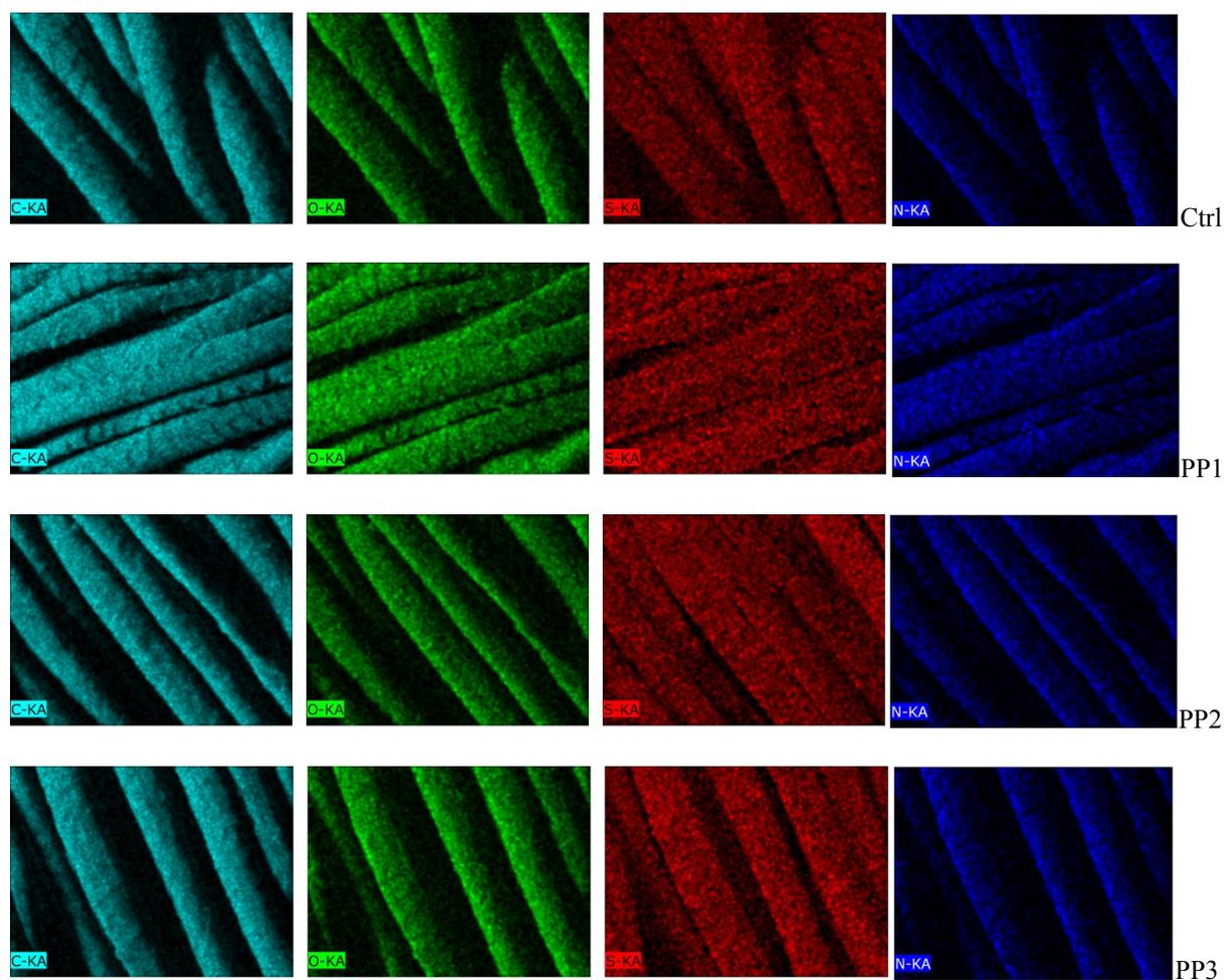
**Fig. S4.** Elemental distribution of C, O, N, and S in untreated (a) and wool fabrics treated with 5% owf PP-1, PP-2, and PP-3.
