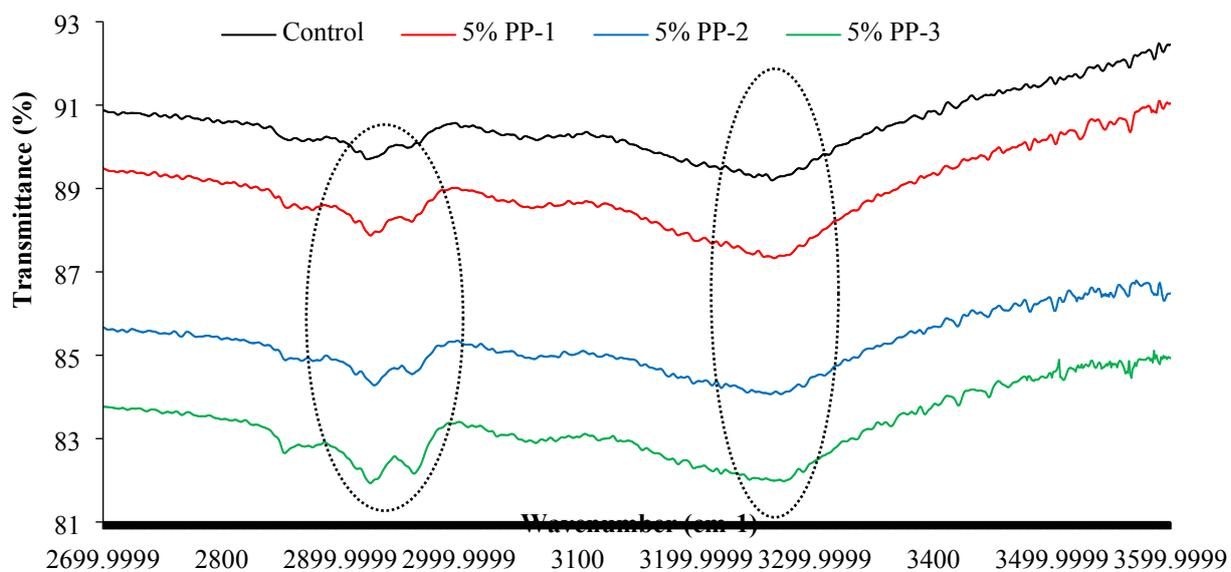
**Fig. S3.** ATR-FTIR spectra of wool fabric treated with various PPs at 5% owf at pH 5.
