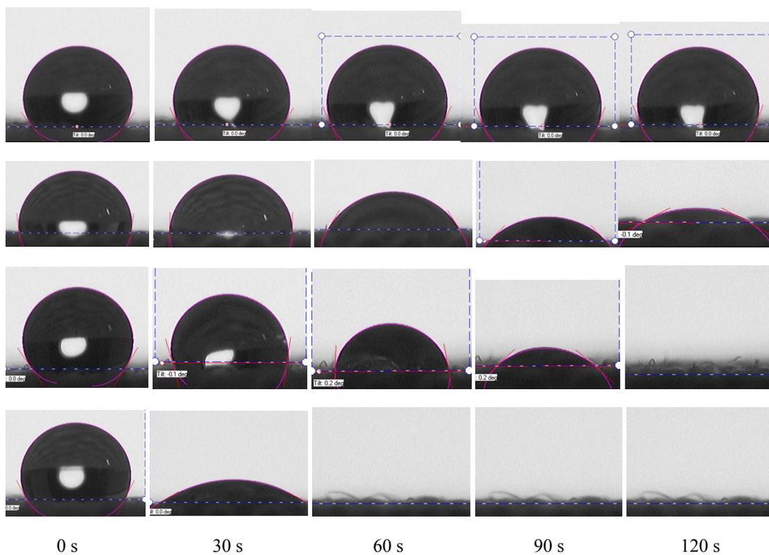
**Fig. S2.** Optical images of shape of droplets of water at various times.
