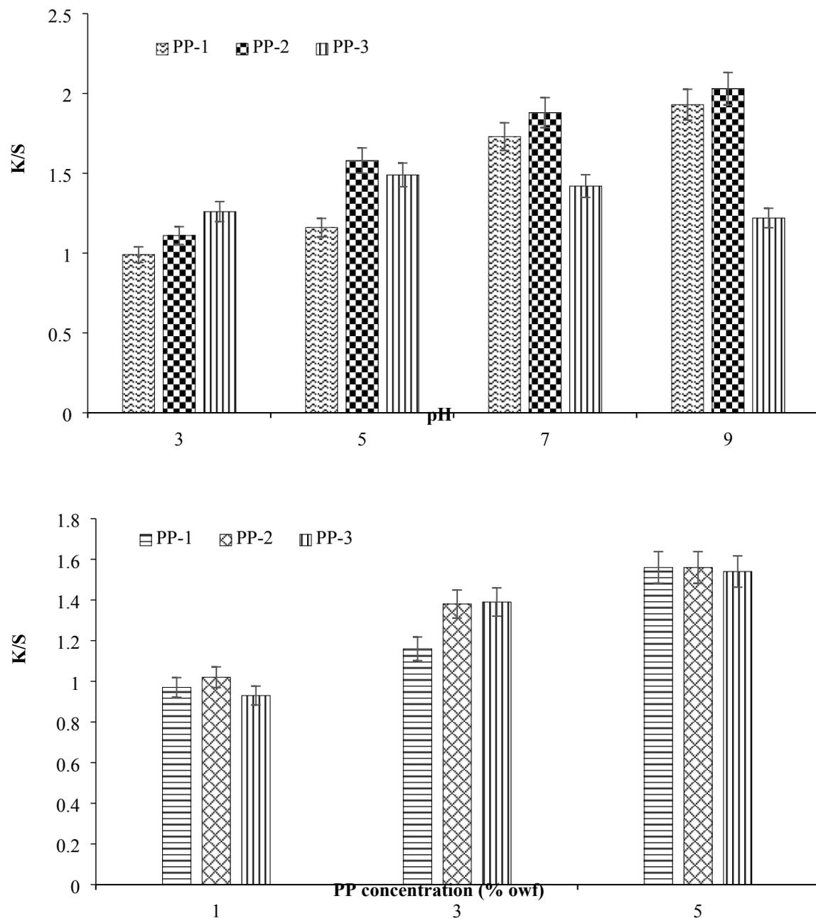
**Fig. S1.** Effect of treatment pH (top) and PP concentrations bottom) on the absorption of wool fabric treated with PP-1, PP-2, and PP-3.
