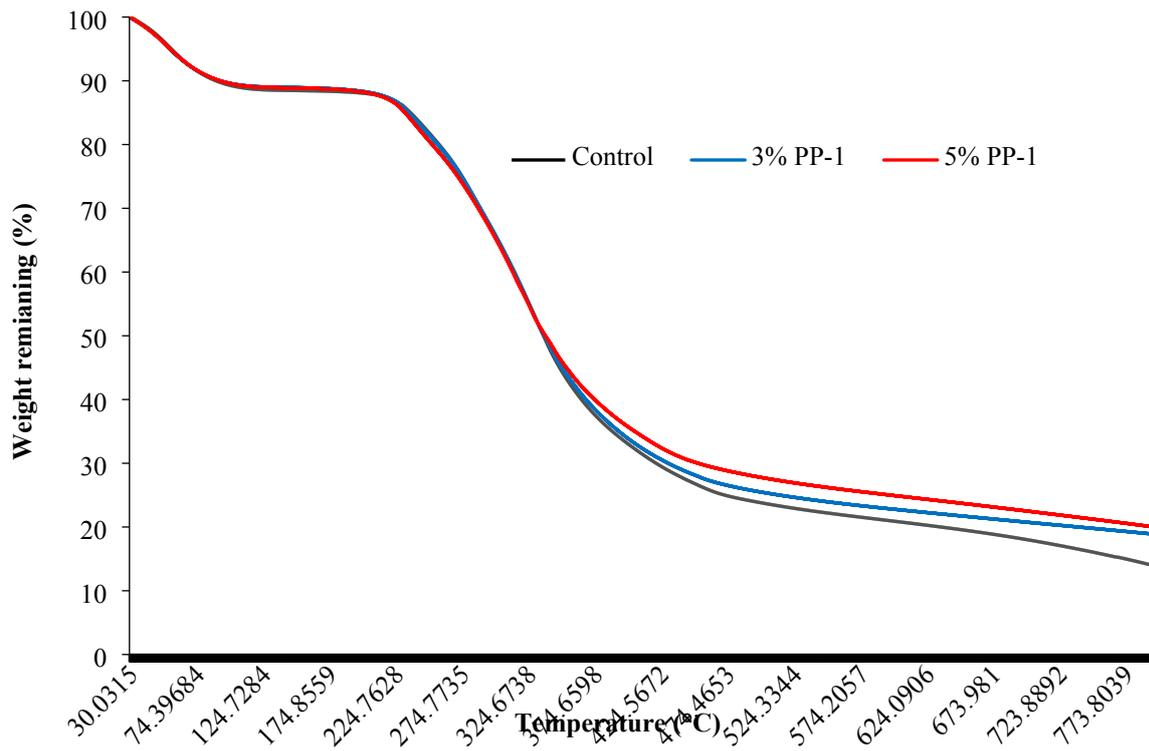
**Fig. S5.** Weight loss of wool fabric treated with PP-1 over room temperature to 800 °C under nitrogen.
