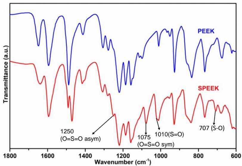
Fig.S1 ATR- FTIR spectra of PEEK and SPEEK.
