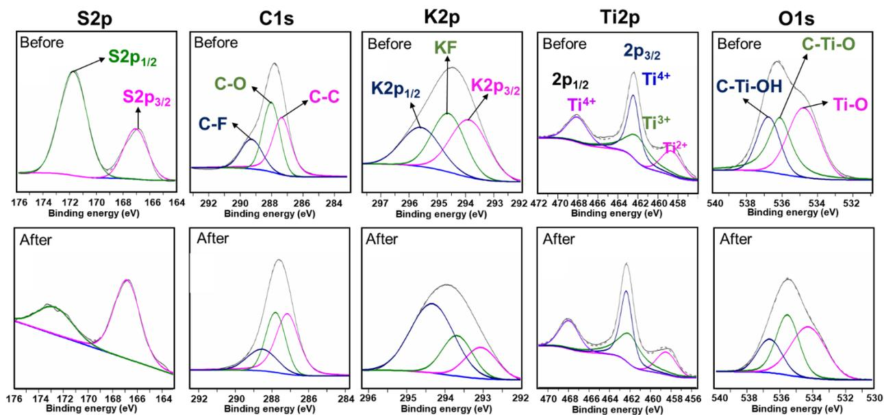
Fig.S6 Deconvolution of 12%MKT-NW/C- SPEEK hybrid composite PEM before and after the H<sub>2</sub> evolution testing for 5h.
