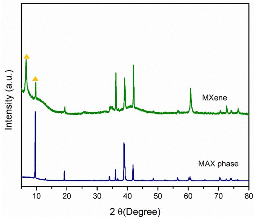
Fig. S2 WXR D patterns of MAX phase and MXene.
