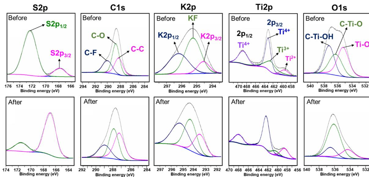
Fig.S5 Deconvolution of 5%MKT-NW/C- SPEEK hybrid composite PEM before and after the H<sub>2</sub> evolution testing for 5h.
