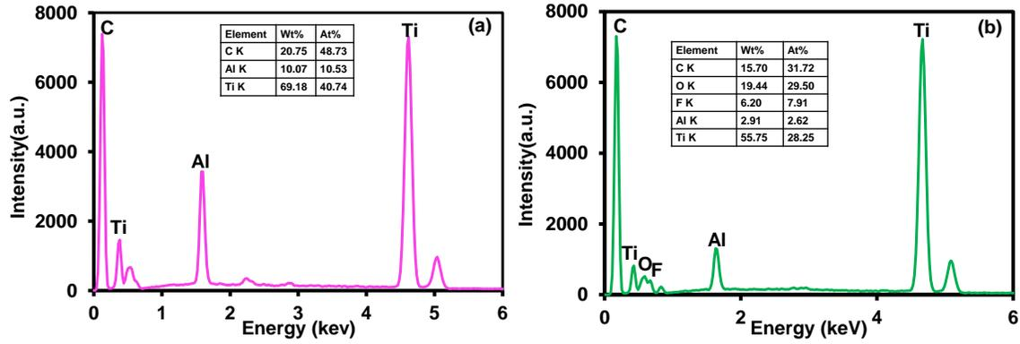
Fig.S3 EDS mapping of (a) MAX phase and (b) MXene.
