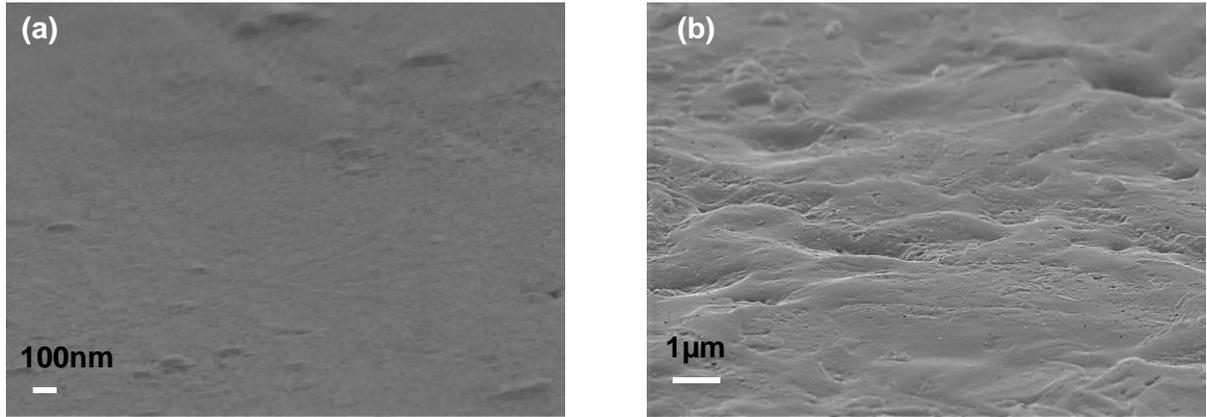
Fig.S4 FE- SEM images of surface morphology of (a) C- SPEEK and (b) 12%MKT-NW/C- SPEEK hybrid composite PEM.
