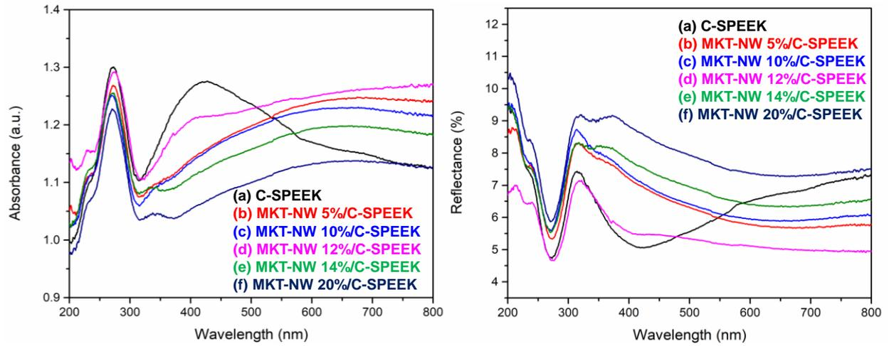
**Fig.S7** Absorption spectra and diffuse reflectance spectra of (a) C-SPEEK, and MKT- NW/C-SPEEK composite films contain 5 – 20%wt of MKT-NW (b) – (f).
