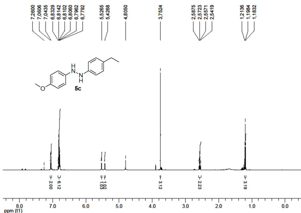
**4-Ethyl-4'-methoxyhydrazobene (5c):  $^{13}\text{C-NMR}$  (125 MHz,  $\text{CDCl}_3$ )**
