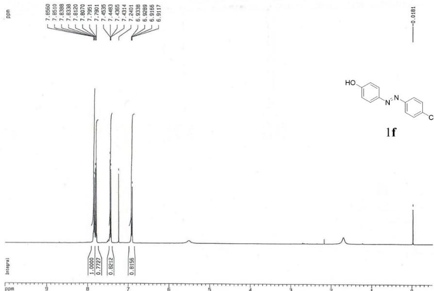
**(E)-4-((4-chlorophenyl)diazenyl)phenol (1f):  $^{13}\text{C-NMR}$  (100 MHz,  $\text{CDCl}_3$ )**
