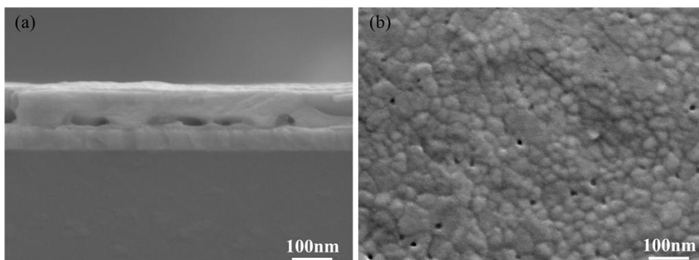
Fig S7 SEM (a) cross-view and (b) surface with  $\text{CsPb}_{0.75}\text{Sn}_{0.25}\text{I}_3$
