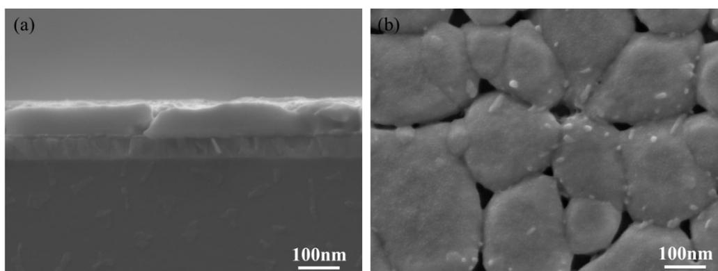
Fig S5 SEM (a) cross-view and (b) surface with  $\text{CsPb}_{0.25}\text{Sn}_{0.75}\text{I}_3$
