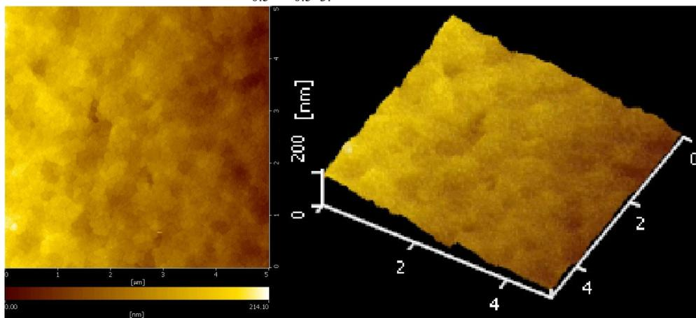
Fig S2. AFM top view and 3D topography images with  $\text{CsPb}_{0.5}\text{Sn}_{0.5}\text{I}_3$
