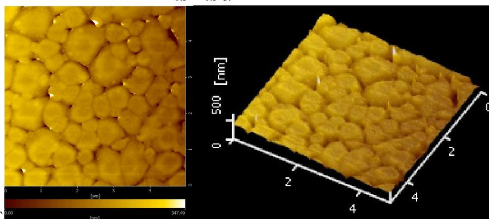
Fig S3. AFM top view and 3D topography images with  $\text{CsPb}_{0.25}\text{Sn}_{0.75}\text{I}_3$
