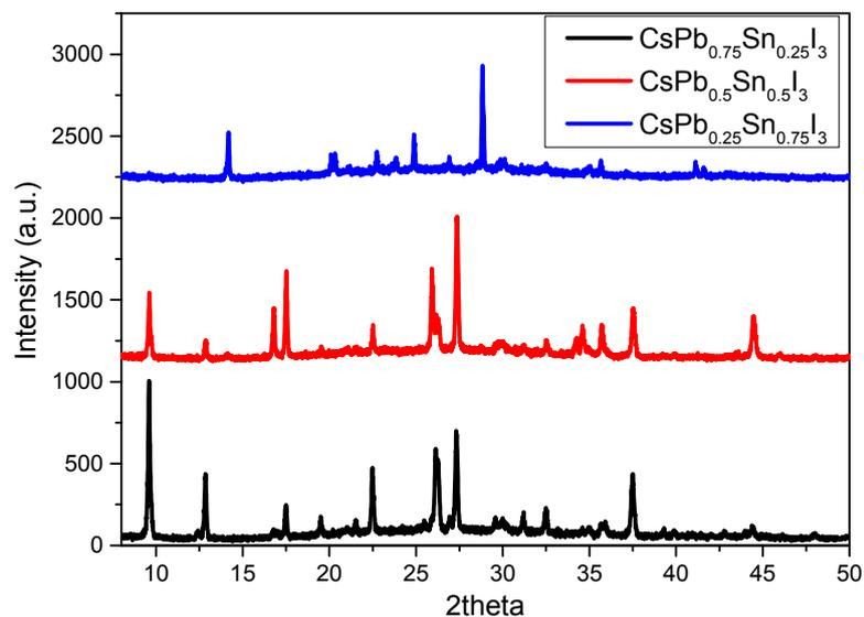
Fig S4. XRD of  $\text{CsPb}_{0.75}\text{Sn}_{0.25}\text{I}_3$ ,  $\text{CsPb}_{0.5}\text{Sn}_{0.5}\text{I}_3$  and  $\text{CsPb}_{0.25}\text{Sn}_{0.75}\text{I}_3$
