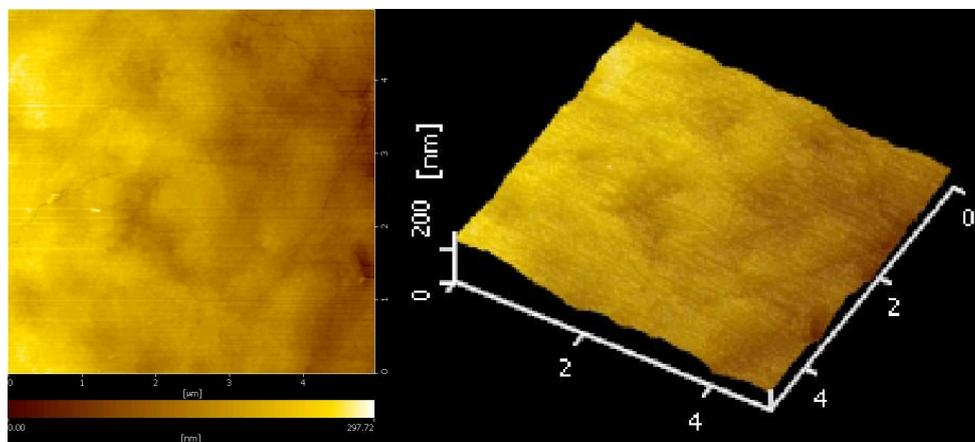
Fig S1. AFM top view and 3D topography images with  $\text{CsPb}_{0.75}\text{Sn}_{0.25}\text{I}_3$
