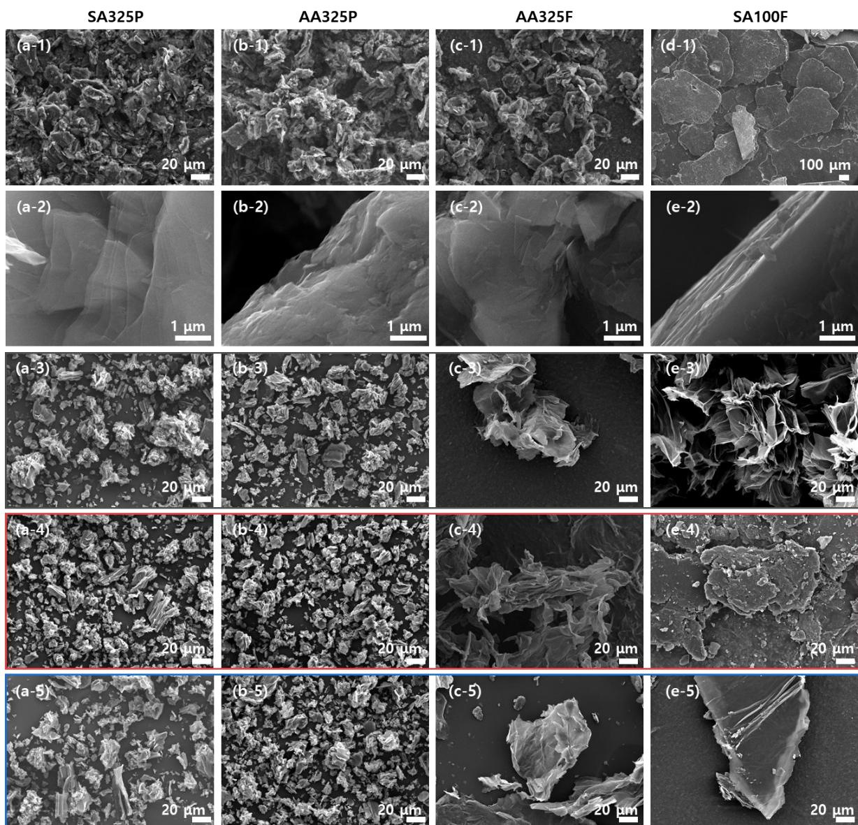
**Fig. S2.** SEM image of graphite source (a-d) and GO by different oxidation method. (1-2) Graphite with different magnification of x500 and x20,000. (3-5) Low magnification SEM image (x500) of GO from HGO, HGO+, and IGO, respectively.
