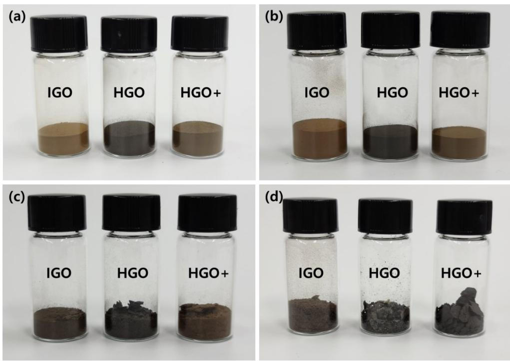
**Fig. S1.** Digital images of GO powders. Three different oxidation methods (IGO, HGO, and HGO+, respectively) are applied to graphite sources; (a) SA325P, (b) AA325P, (c) AA325F, and (d) SA100F.
