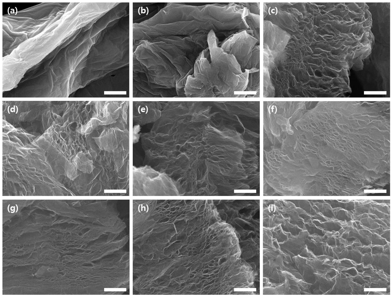
**Fig. S4.** High magnification SEM image of (a) GO, and (b-i) TEGO powders by annealing temperature 100, 200, 300, 400, 500, 600, and 700 °C, respectively.
