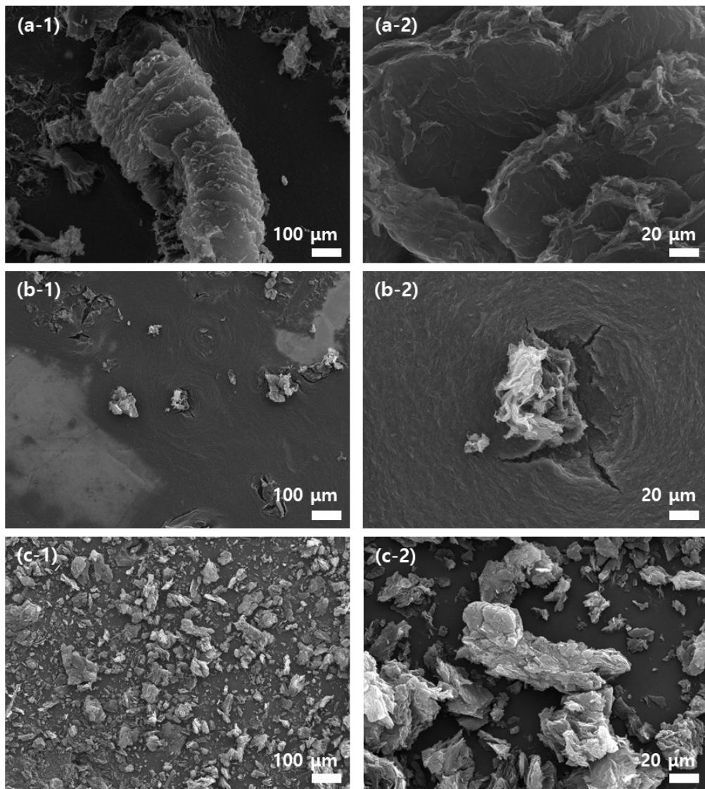
**Fig. S3.** SEM image of thermally expanded graphene oxide (TEGO) from SA100F with (a) HGO, (b) HGO+, and (c) IGO with different magnifications: (1-2) x500 and x10,000, respectively.
