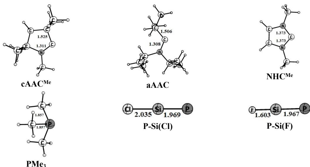
**Figure S0.** Optimized geometries of ligands cAAC<sup>Me</sup>, aAAC, NHC<sup>Me</sup>, PMe<sub>3</sub>, and P-Si(Cl/F) at BP86(D3BJ)/def2-TZVPP level.
