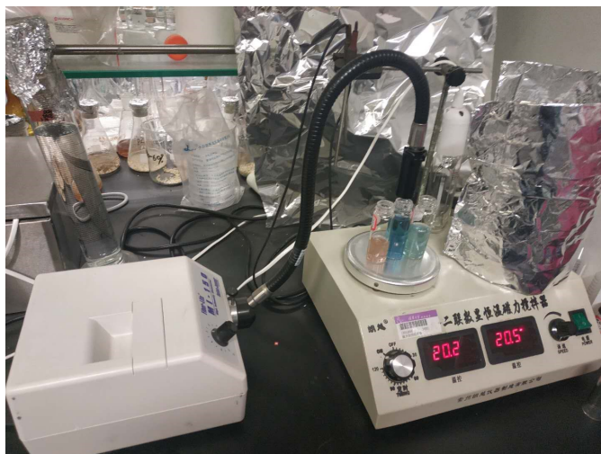
Figure S1. Anisotropic Silver nanoparticles fabrication setup employed to produce three different shapes of AgNP (triangular, cubes and rods)
