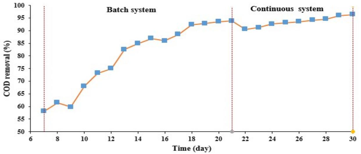
**Fig S1.** Efficiency of MBBR biological reactor in COD removal during the early stages of reactor adaptation
