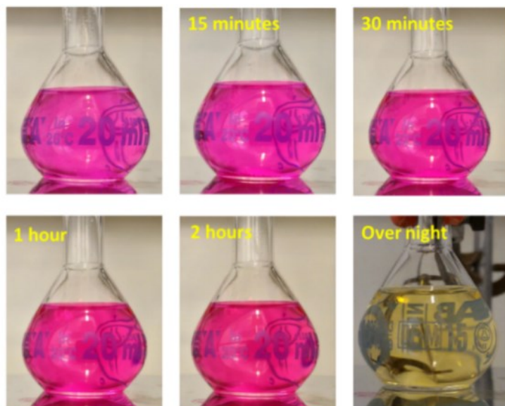
Figure S1 : Color evolution for the binary mixture DDT+bptz (in absence of Au).
