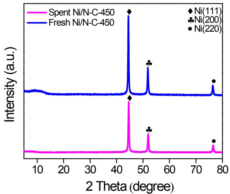
Fig. S5 XRD patterns of fresh and spent Ni/N-C-450 catalyst.
