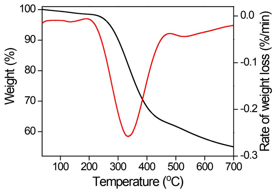
**Fig. S1** TG and DTG curves of Ni-MOF.
