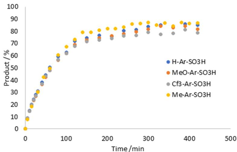
**Figure S1.** Reaction profiles using different *para*-substituted aryl sulfonic acids, *p*-Z-C<sub>6</sub>H<sub>4</sub>SO<sub>3</sub>H (monitored by HPLC). Reaction conditions: 4-methylacetanilide (0.75 mmol), *n*-butyl acrylate (0.75 mmol), Pd(OAc)<sub>2</sub> (5 mol%, 0.0375 mmol), aryl sulfonic acid (0.75 mmol, 1 equivalent), AcOH (3 mL), BQ (0.75 mmol), 30 °C.
