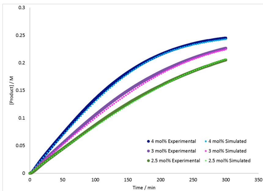
**Figure S7.** Experimental and simulated data for different catalyst loadings (2.5-4 mol%). Initial concentrations: 4'-methylacetanilide = 0.3 M, butyl acrylate **2** = 0.25 M, BQ = 0.25 M, TsOH = 0.125 M.
