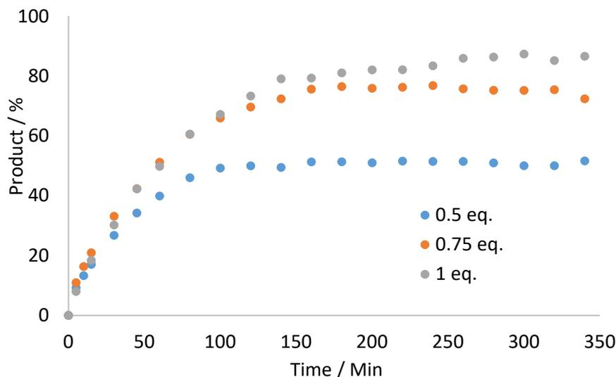
**Figure S3.** Reaction profiles using different amounts of acrylate (0.5-1 equivalents): 4-methylacetanilide (0.75 mmol), Pd(OAc)<sub>2</sub> (5 mol%, 0.0375 mmol), aryl sulfonic acid (0.75 mmol, 1 equivalent), AcOH (3 mL), BQ (0.75 mmol), 30 °C. The initial rates show that the reaction is zero order in acrylate. Note: these experiments were conducted using sub-stoichiometric amount of the alkene to prevent formation of di-substituted compound.
