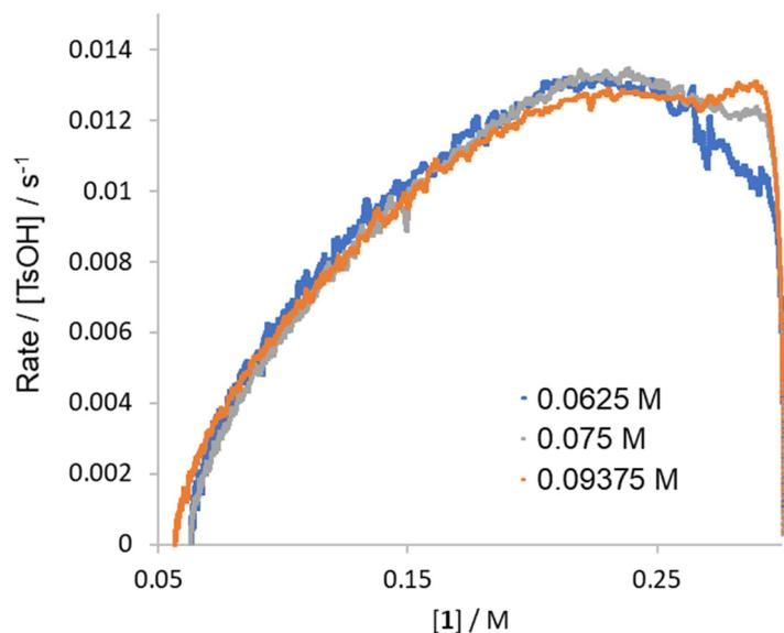
**Figure S4.** Plot of reaction rate/[TsOH] vs [1], between 2.5-37.5 mol% (0.0625-0.09375 M) of TsOH.
