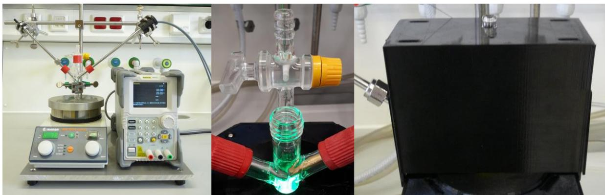
**Fig. S2:** Integration of compatible immersion probes in the photoreactor (left and middle). Light cover for Raman application (right).
