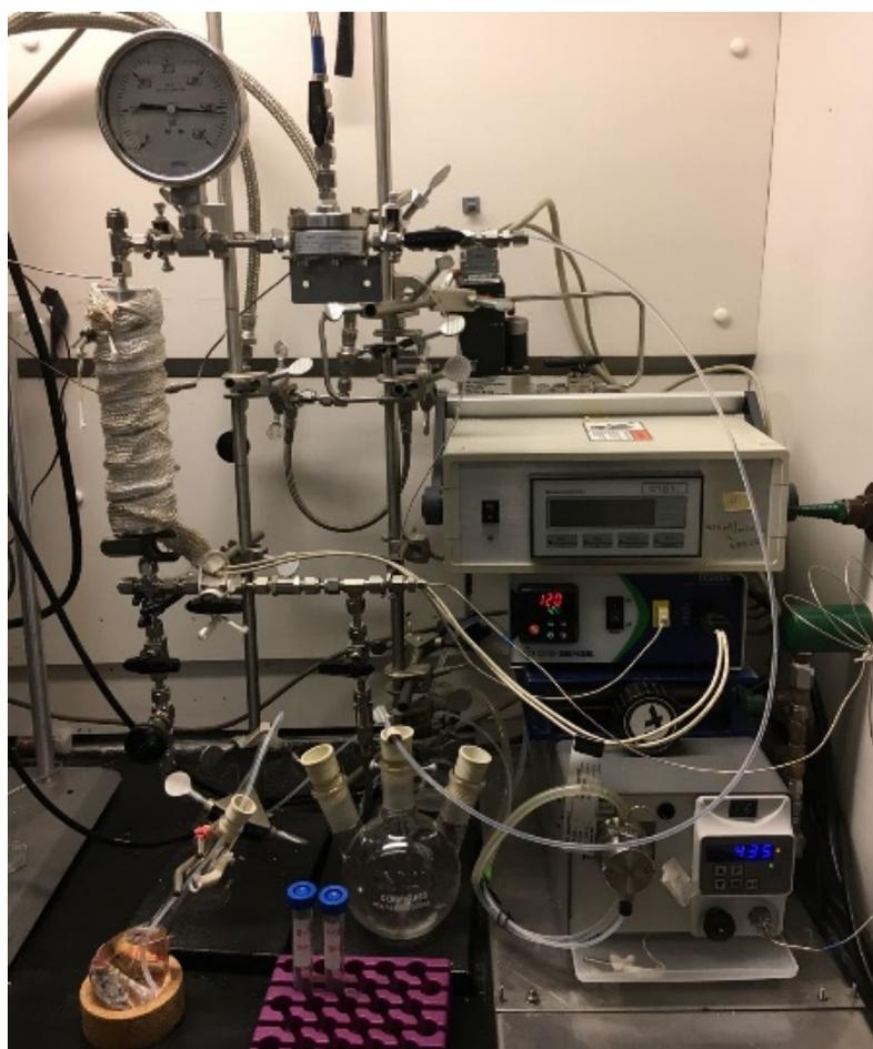
**Scheme S1.** Schematic (top) and photograph (bottom) of continuous flow reactor.
