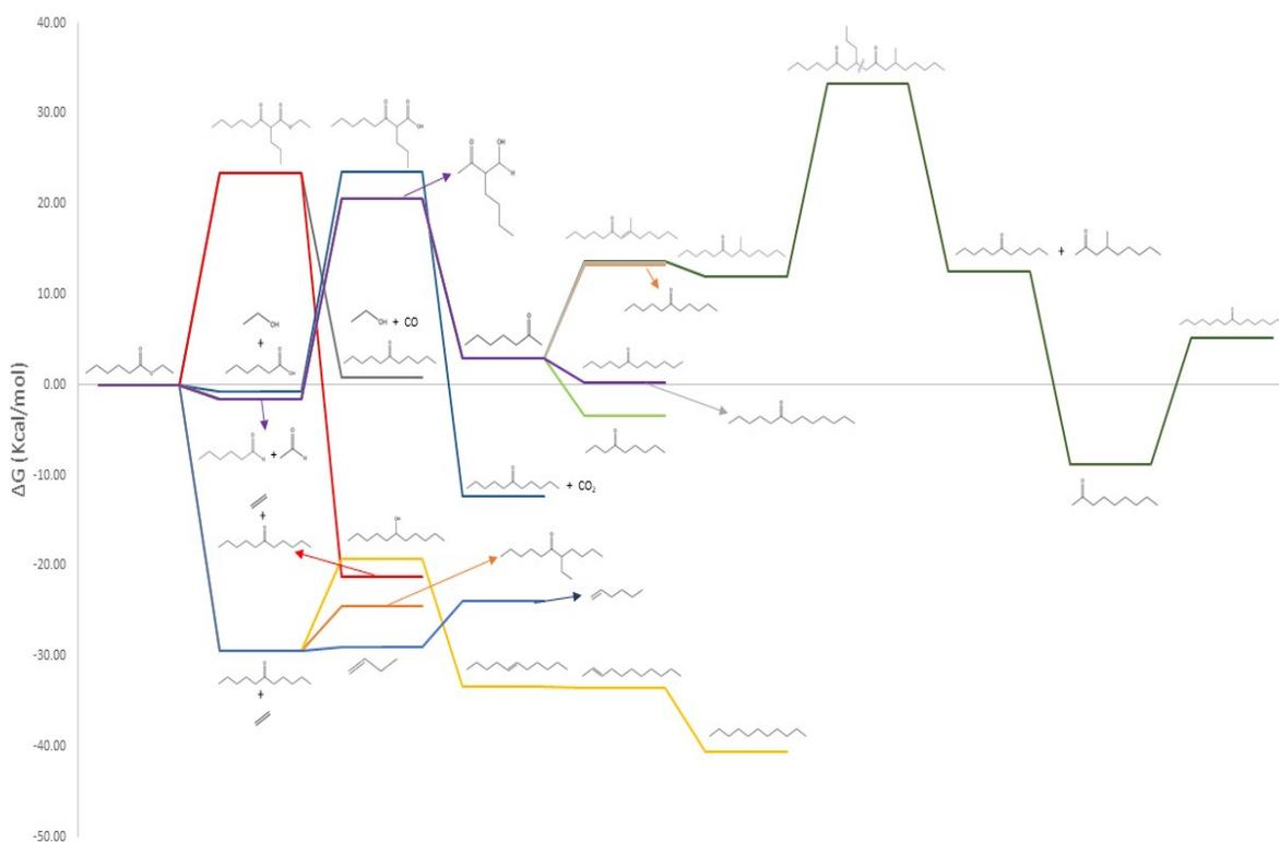
Figure S1. Standard changes of Gibbs free energy (Kcal/mol) for the reactions at 623 K.
