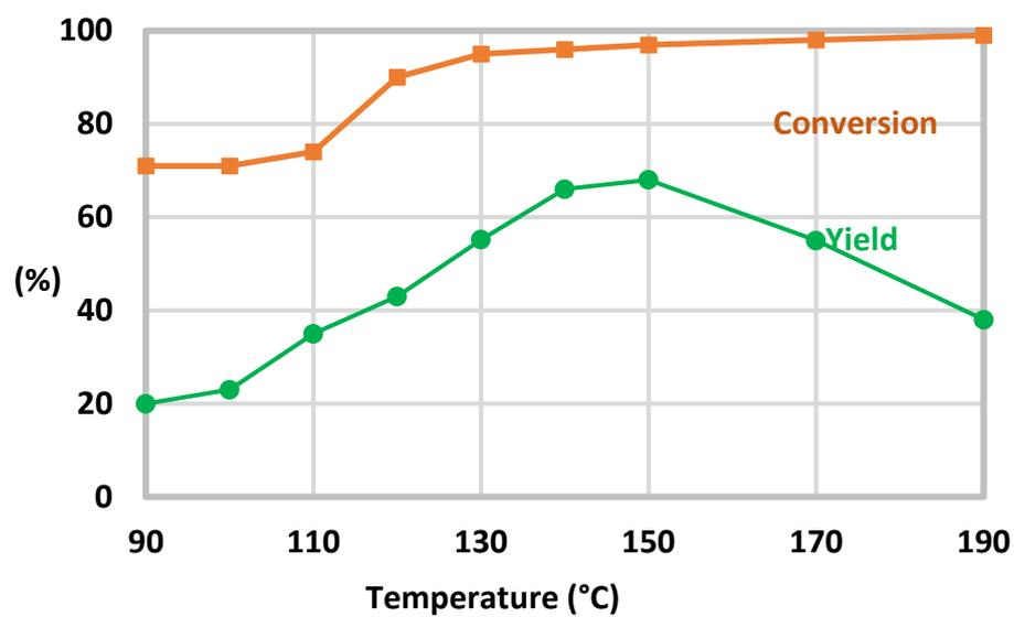
**Figure S9:** Reaction results by temperature change at 0.5M in Methanol, nifedipine (●, green), conversion (■, orange).
