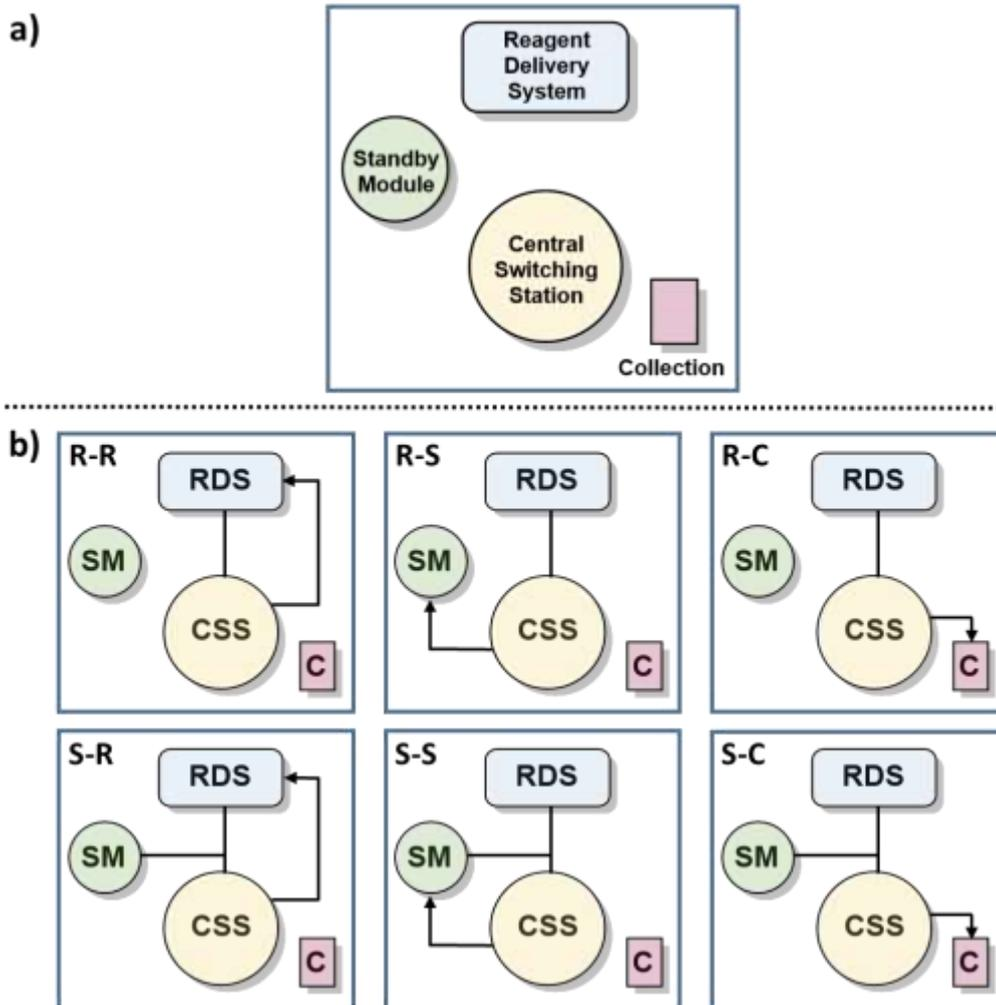
**Figure S3:** a) The radial synthesizer's main sections: reagent delivery system (RDS), central switching station (CSS), standby module (SM) and collection vessels (C). b) Six pathways of solution flow through the instrument are described by the starting location of the reagents and their destination. For example, **R-C** refers to a solution starting in the RDS and ending in the Collection vessel.
