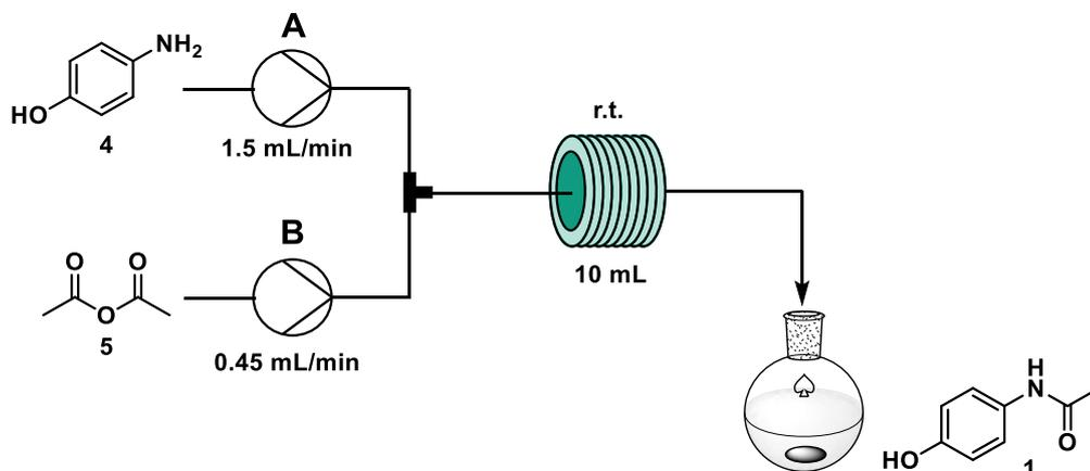
**Figure S5:** Continuous flow synthesis of paracetamol followed by batch crystallization.
