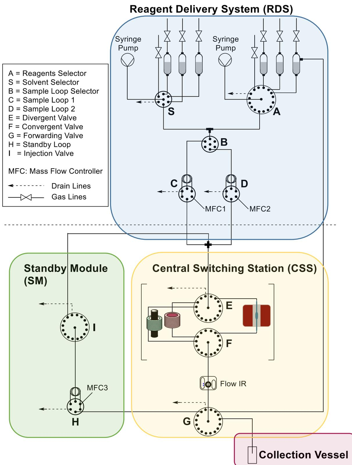
**Figure S2:** The Radial Synthesizer is composed of three main blocks: the reagents delivery system (RDS), the central switching station (CSS) and the standby module (SM).
