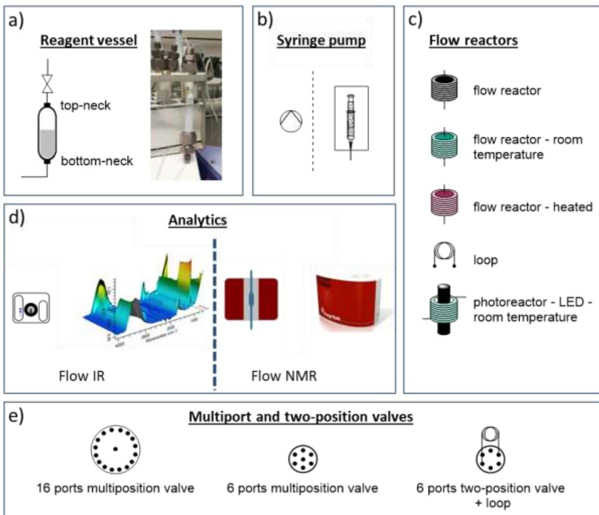
Figure S1: Components of the radial synthesizer.
