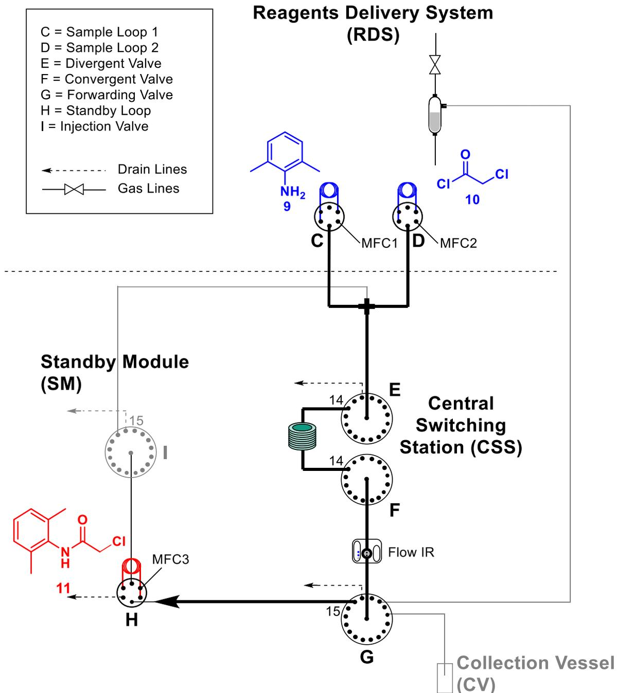
Figure S10: First step of the radial synthesis of Lidocaine (Li-1) performed using the R-S pathway.
