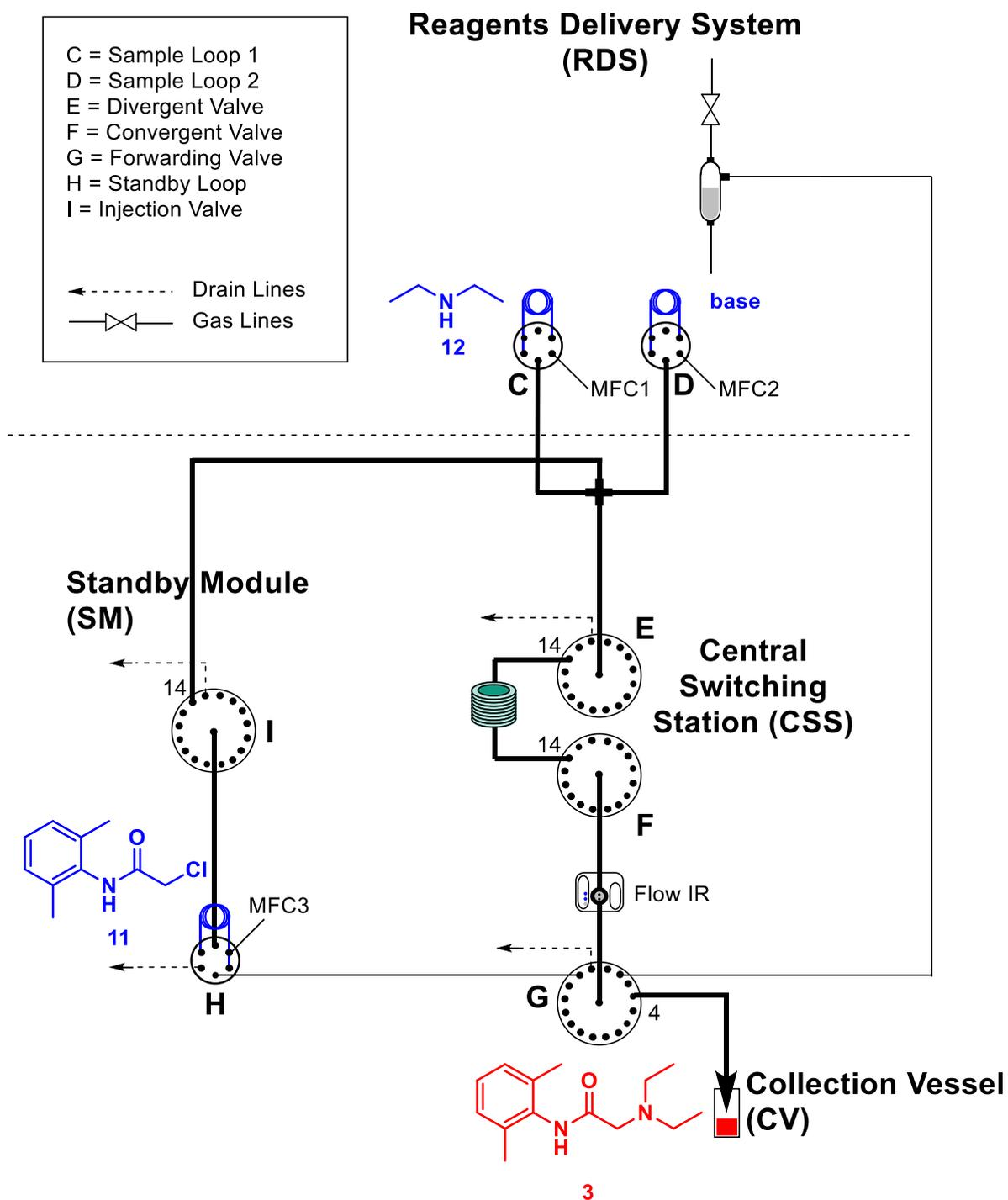
**Figure S11:** Second step of the radial synthesis of Lidocaine (Li-2) performed using the S-C pathway.
