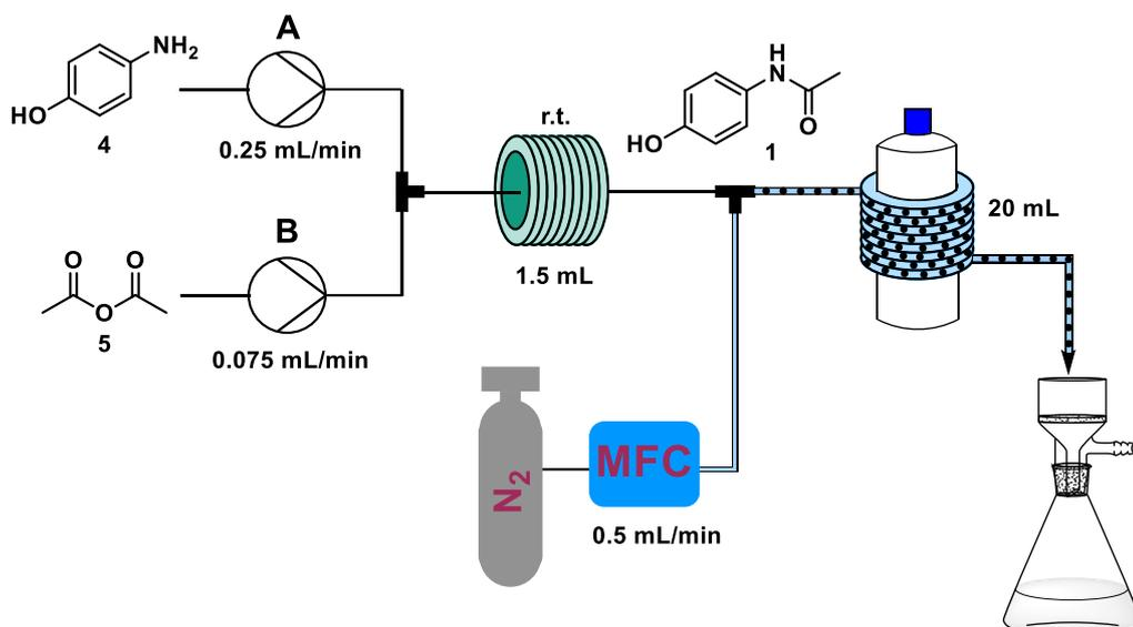
**Figure S6:** Continuous flow synthesis of paracetamol followed by flow crystallization and filtration.
