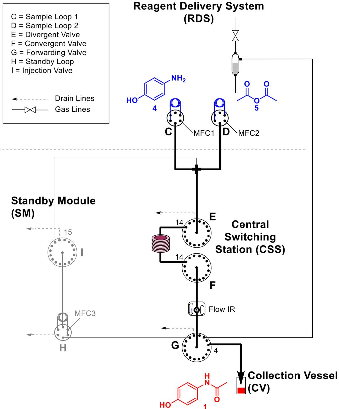
**Figure S4:** The synthesis of paracetamol was optimized using the R-C pathway in the radial synthesizer. Reagents are delivered by the RDS, pass through a heated or room temperature coil and the product is collected in a non-pressurized collection vessel (CV).
