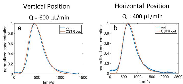
**Figure S3:** RTD profiles of the high-temperature CSTR cascade when the orientation is (a) vertical and (b) horizontal. Blue line is the experimental RTD profile and the red line represents the profile based on the ideal CSTRs in series model.
