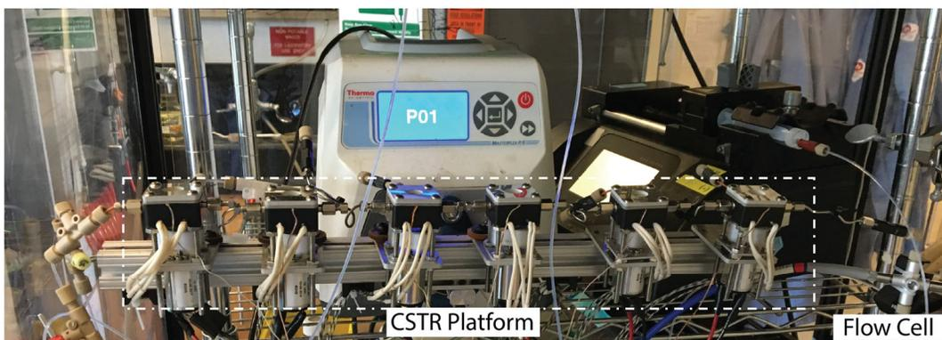
**Figure S1:** Image of the high-temperature continuous stirred-tank reactors for the synthesis of InP/ZnS QDs
