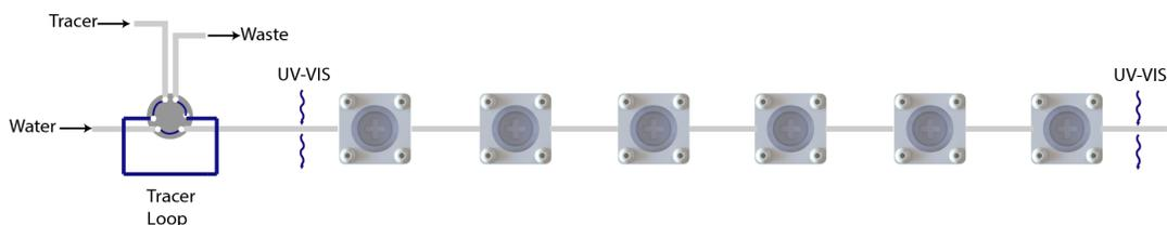
**Figure S2:** Scheme of the residence time distribution measurements using in-line UV-Vis to record concentration profiles at the inlet and outlet.
