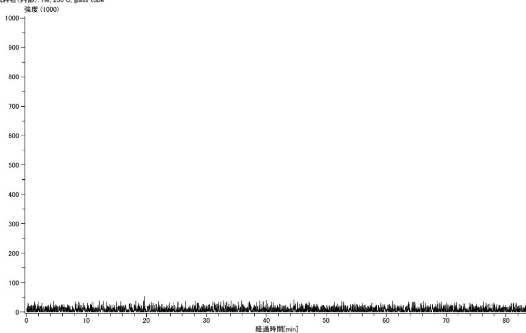
Figure S5. SIC of 1-d 4 (corresponding to decomposed internal standard 2-d 4 , no detection of peak indicates 2-d 4 is stable both under reaction conditions and on DART ionization)
