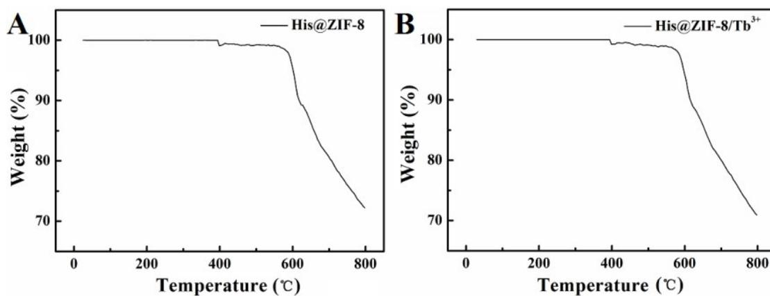
Fig. S1 TGA curve of the synthesized His@ZIF-8 (A) and His@ZIF-8/Tb<sup>3+</sup> (B).
