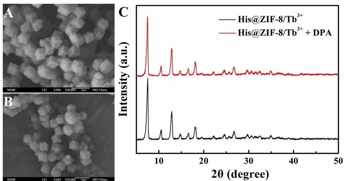
**Fig. S8** SEM images of His@ZIF-8/Tb<sup>3+</sup> before (A) and after (B) reacting with DPA aqueous solution (1 mmol L<sup>-1</sup>) for 3 min. (C) XRD patterns of His@ZIF-8/Tb<sup>3+</sup> before and after reacting with DPA aqueous solution (1 mmol L<sup>-1</sup>) for 3 min.
