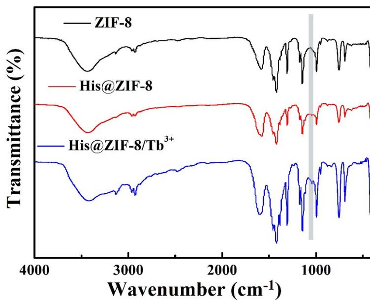
Fig. S2 FT-IR spectra of ZIF-8, His@ZIF-8 and His@ZIF-8/Tb<sup>3+</sup>.
