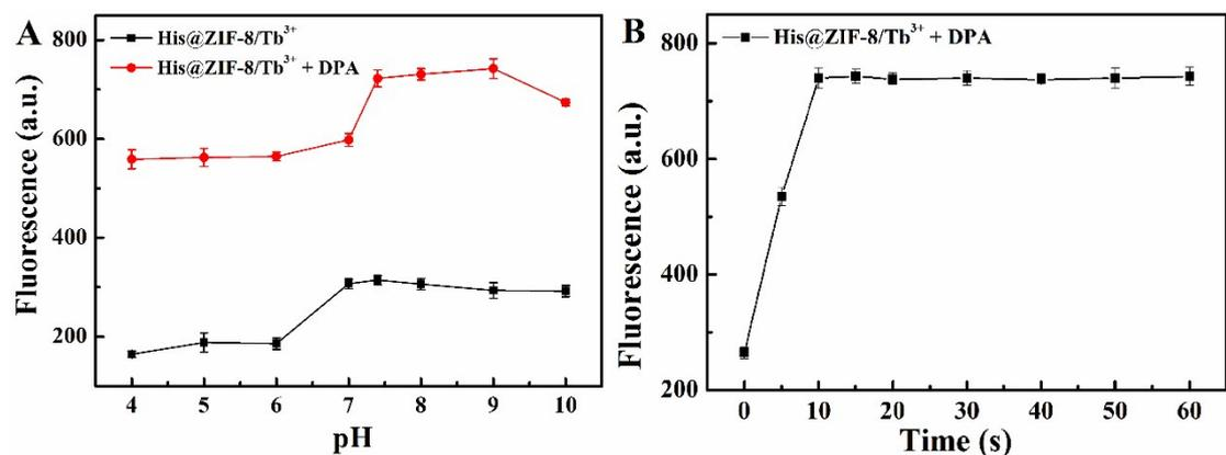
**Fig. S6** (A) Effects of pH values on fluorescence intensity of His@ZIF-8/Tb<sup>3+</sup> with DPA (red line) and without DPA (black line). (B) Effects of reaction time on fluorescence intensity of His@ZIF-8/Tb<sup>3+</sup> with DPA (1  $\mu\text{mol L}^{-1}$ ); HEPES buffer: 20  $\text{mmol L}^{-1}$ , pH 7.4.
