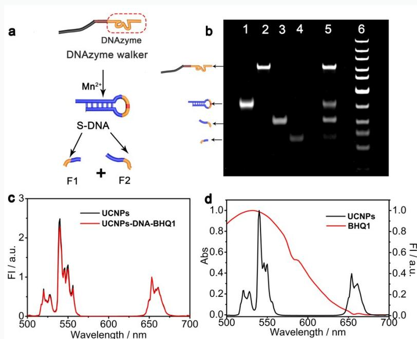
**Fig. S2** (a) Schematic illustration and (b) Gel electrophoresis assay characterization of DNAzyme catalytic cleavage reaction. Lane 1: S-DNA, lane 2: DNAzyme walker, lane3: F2, lane4: F1, lane5: mixture of S-DNA and DNAzyme walker, lane6: 300-bp DNA ladder markers. (c) Normalized upconversion luminescence spectra of UCNPs and UCNPs-DNA-BHQ1 (d) Normalized fluorescence emission spectra of UCNPs under 980 nm excitation and normalized absorption spectra of BHQ1.
