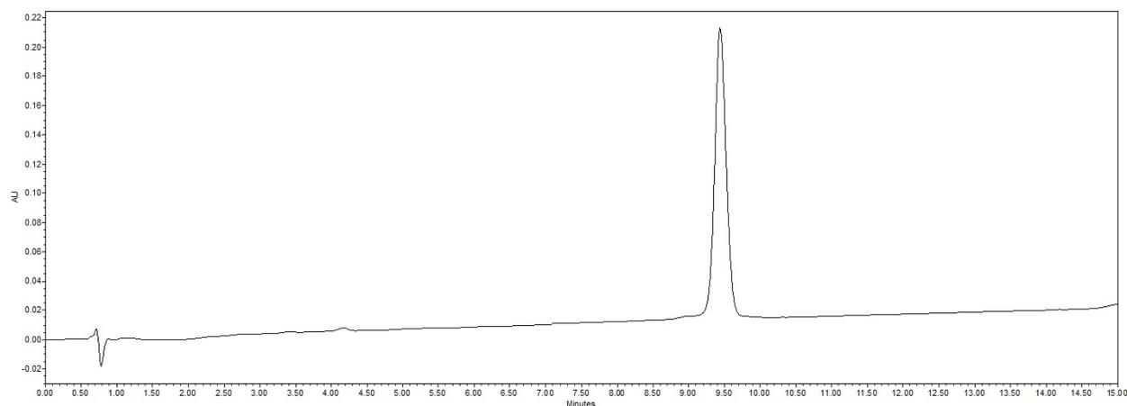
**Fig. S3** Analytical RP-HPLC trace of **S3**:  $t_R$  = 9.44 min ( $\lambda$ =214 nm, 0–30% B over 15 min).
