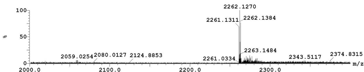
**Fig. S30** HRMS (ESI<sup>+</sup>-TOF) of **17**:  $m/z$  calcd. for  $[\text{M}+\text{H}]^+$  2261.1400 (monoisotopic), found 2261.1311.
