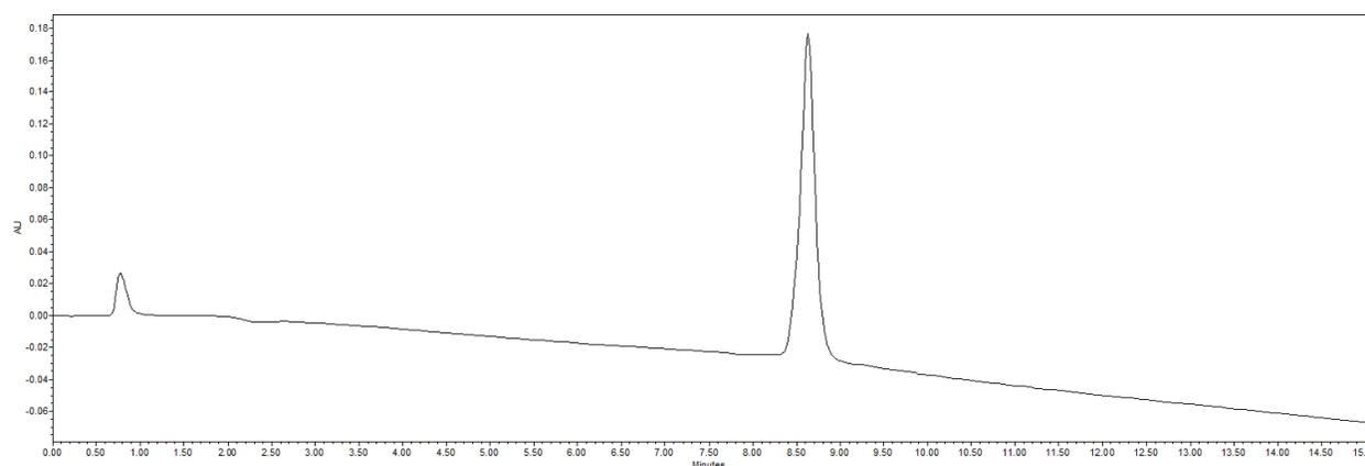
**Fig. S11** Analytical RP-HPLC trace of **5**: t<sub>R</sub> = 8.67 min (λ<sub>max</sub> = 214 nm, 0–40% B over 15 min).
