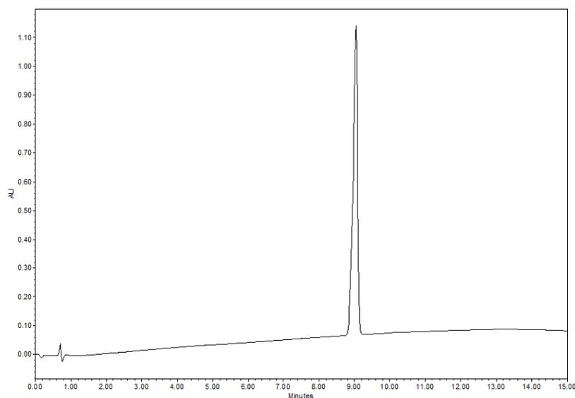
**Fig. S31** Analytical RP-HPLC trace of **S8**.  $t_R = 9.04$  min ( $\lambda_{\text{max}} = 214$  nm, 5–100% B over 15 min).
