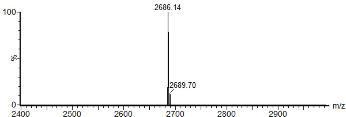
**Fig. S26** LRMS (ESI<sup>+</sup>-MS) spectrum of **S6**:  $m/z$  calcd. for  $[M+6H]^{6+}$  2686.1 (monoisotopic), found 2686.1.
