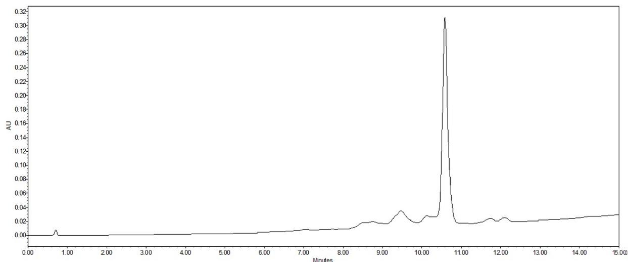
**Fig. S177** Analytical RP-HPLC trace of **12**:  $t_{\text{R}} = 10.59$  min ( $\lambda_{\text{max}} = 214$  nm, 5–100% B over 15 min)
