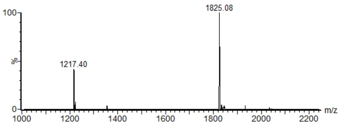
**Fig. S22** LRMS (ESI<sup>+</sup>-MS) spectrum of **S5**:  $m/z$  calcd. for  $[M+2H]^{2+}$  1824.9 (average), found 1825.1; calcd. for  $[M+3H]^{3+}$  1216.9, found 1217.4.
