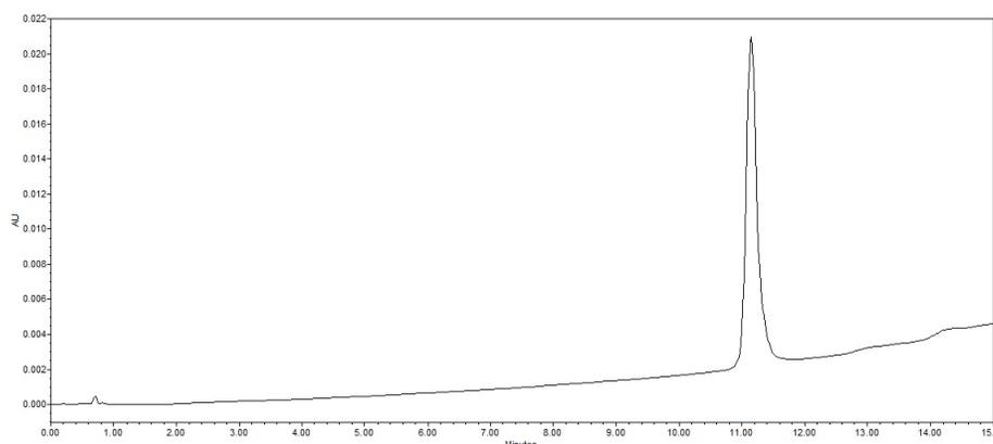
**Fig. S41** Analytical RP-HPLC trace of **S10**:  $t_R = 11.15$  min ( $\lambda_{max} = 214$  nm, 0–40% B over 15 min).
