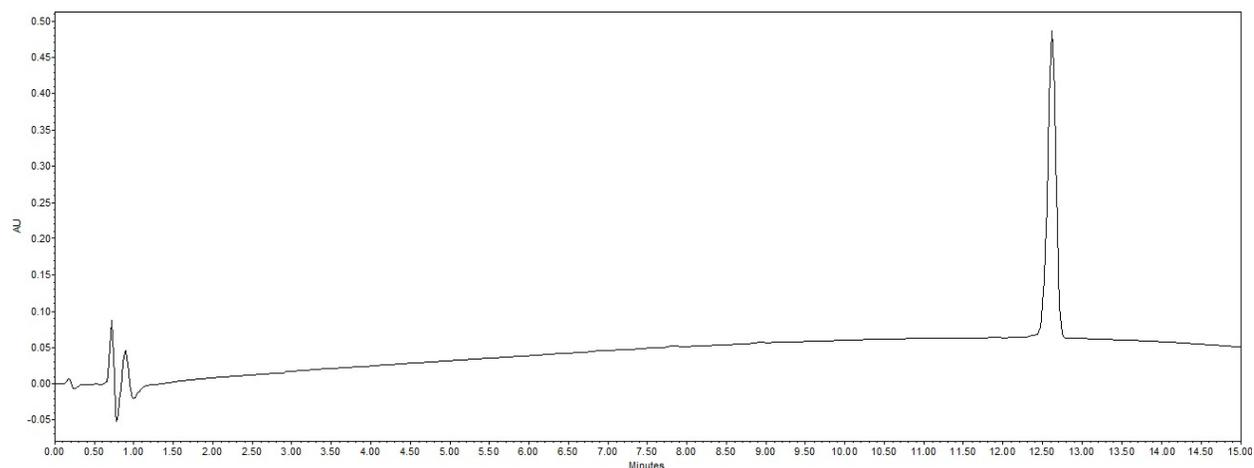
**Fig. S155** Analytical RP-HPLC trace of **11**:  $t_R = 12.62$  min ( $\lambda_{\text{max}} = 214$  nm, 5–100% B over 15 min)
