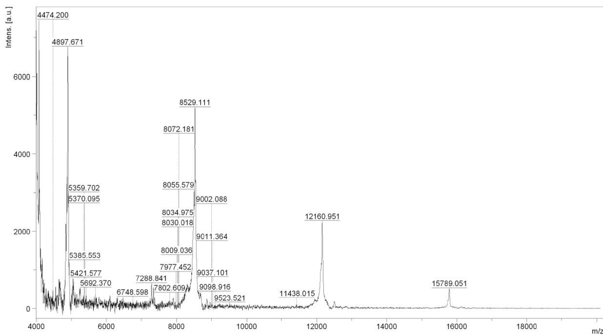
**Fig. S204** LRMS (MALDI-TOF) spectrum of **14**:  $m/z$  calcd. for  $[M+Na]^+$  15786.5 (average), found 15789.1.
