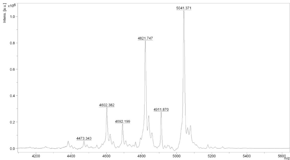
**Fig. S40** LRMS (MALDI-TOF) spectrum of **20**:  $m/z$  calcd. for  $[M+H]^+$  5040.5 (average), found 5041.4.
