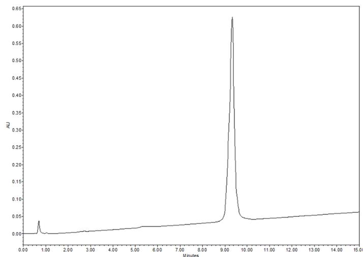
**Fig. S35** Analytical RP-HPLC trace of **19**:  $t_R = 9.33$  min ( $\lambda_{\max} = 214$  nm, 5–40% B over 15 min)
