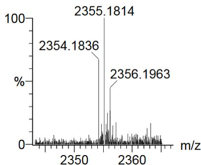
**Fig. S10** HRMS (ESI<sup>+</sup>-TOF) of **3**:  $m/z$  calcd. for  $[\text{M}+\text{H}]^+$  2354.1826 (monoisotopic), found 2354.1836.
