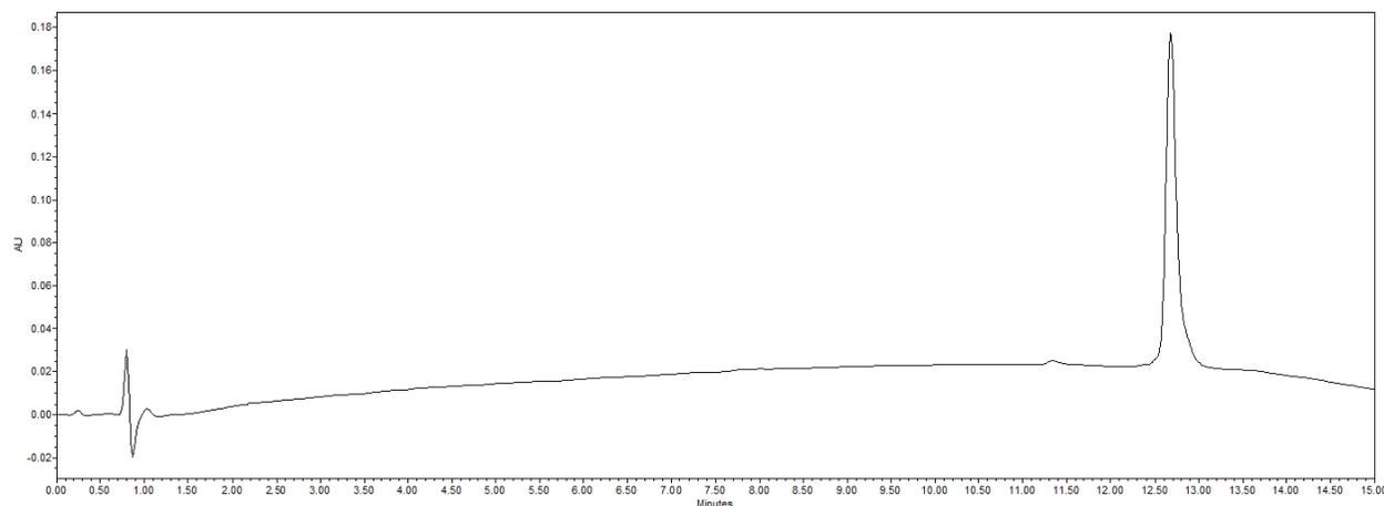
**Fig. S5** Analytical RP-HPLC trace of **1**:  $t_{\text{R}} = 12.67$  min ( $\lambda_{\text{max}} = 214$  nm, 5–100% B over 15 min).
