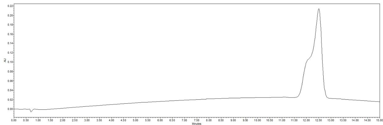
**Fig. S193** Analytical RP-HPLC trace of **14**:  $t_R = 12.51$  min ( $\lambda_{max} = 214$  nm, 50–100% B over 15 min).
