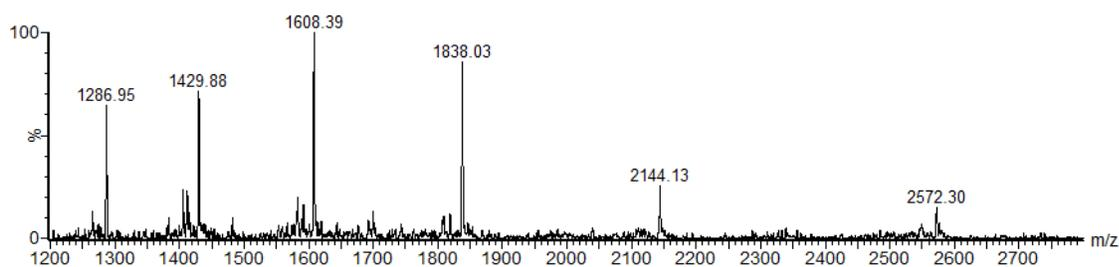
**Fig. S44** LRMS (ESI<sup>+</sup>-MS) spectrum of **21/23**:  $m/z$  calcd. for  $[\text{M}+5\text{H}]^{5+}$  2572.1 (average), found 2572.3; calcd. for  $[\text{M}+6\text{H}]^{6+}$  2143.6, found 2144.1; calcd. for  $[\text{M}+7\text{H}]^{7+}$  1837.5, found 1838.0; calcd. for  $[\text{M}+8\text{H}]^{8+}$  1607.9, found 1608.4; calcd. for  $[\text{M}+9\text{H}]^{9+}$  1429.4, found 1429.9; calcd. for  $[\text{M}+10\text{H}]^{10+}$  1286.6, found 1287.0.
