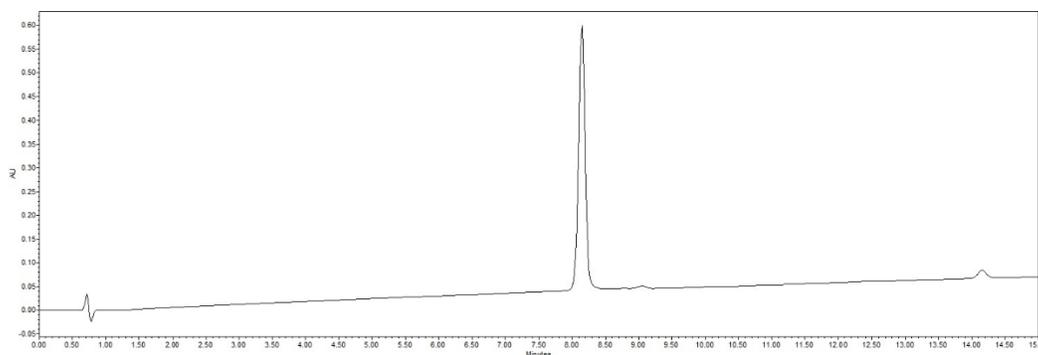
**Fig. S37** Analytical RP-HPLC trace of **S9**:  $t_R = 8.15$  min ( $\lambda_{max} = 214$  nm, 5–60% B over 15 min).
