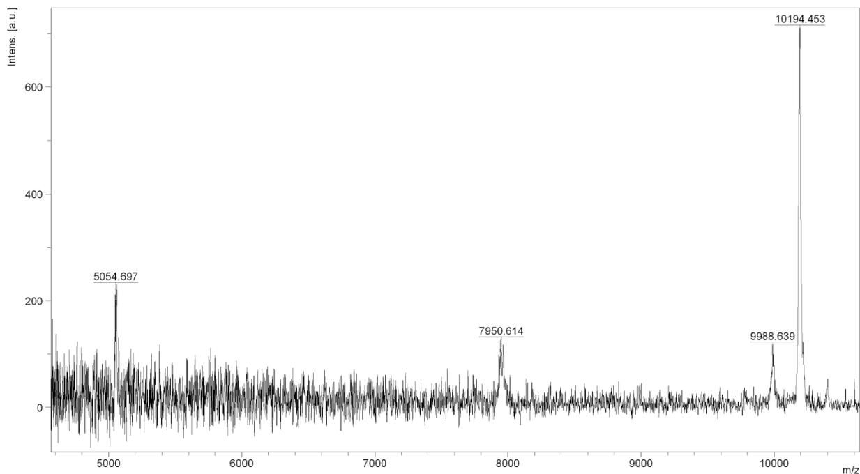
**Fig. S12** LRMS (MALDI-TOF) spectrum of **5**:  $m/z$  calcd. for  $[M+H]^+$  10190.9 (average), found 10194.5.
