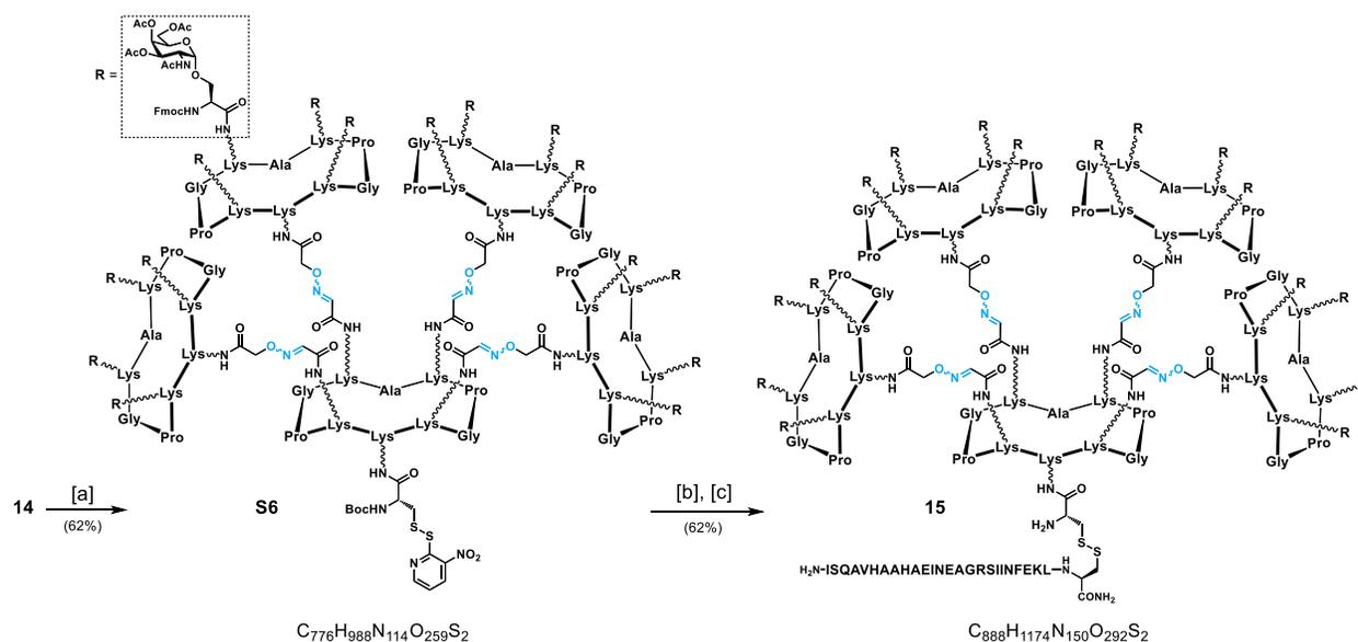
**Scheme S7** Synthesis of hexadecavalent glycodendrimer **15**. Reagents and conditions: [a] Boc-Cys(NPys)-NHS<sup>7</sup> (1.5 equiv), DIPEA (2.15 equiv), DMF, r.t., 30 min, 62% yield; [b] TFA/CH<sub>2</sub>Cl<sub>2</sub> (1:1), r.t., 30 min; [c] Peptide **10** (1.1 equiv), DMF/NaOAc buffer (pH 4.5, 40 mM) (2:1), r.t., 30 min, 62% yield (over two steps)
