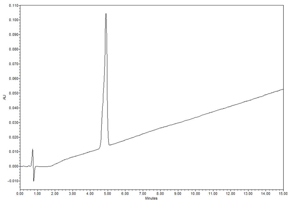
**Fig. S29** Analytical RP-HPLC trace of **17**:  $t_{\text{R}} = 4.09$  min ( $\lambda_{\text{max}} = 214$  nm, 0–40% B over 15 min).
