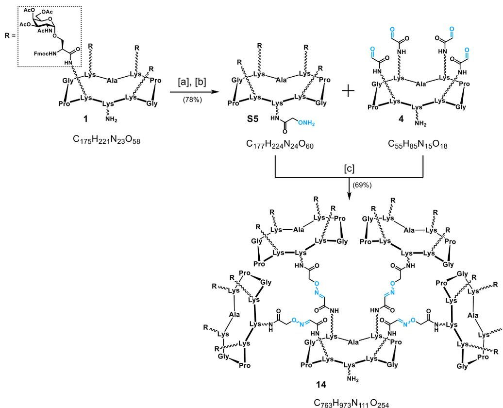
**Scheme S6** Synthesis of hexadecaivalent glycodendrimer **14**. Reagents and conditions: [a] Boc-Aoa-NHS<sup>4</sup> (1.2 equiv), DIPEA (1.5 equiv), DMF, r.t., 30 min; [b] TFA/NH<sub>2</sub>OH/CH<sub>2</sub>Cl<sub>2</sub> (50:2:48), r.t., 30 min, 78% yield (over two steps); [c] S5 (6.0 equiv), 4 (1.0 equiv), 0.1% TFA in H<sub>2</sub>O/CH<sub>3</sub>CN (1:9), 37 °C, 60 min, 69% yield.
