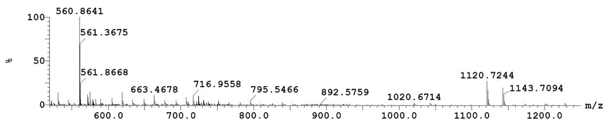
**Fig. S4** HRMS (ESI<sup>+</sup>-TOF) spectrum of **S3**:  $m/z$  calcd. for [M+H]<sup>+</sup> 1120.7206 (monoisotopic), found 1120.7244.
