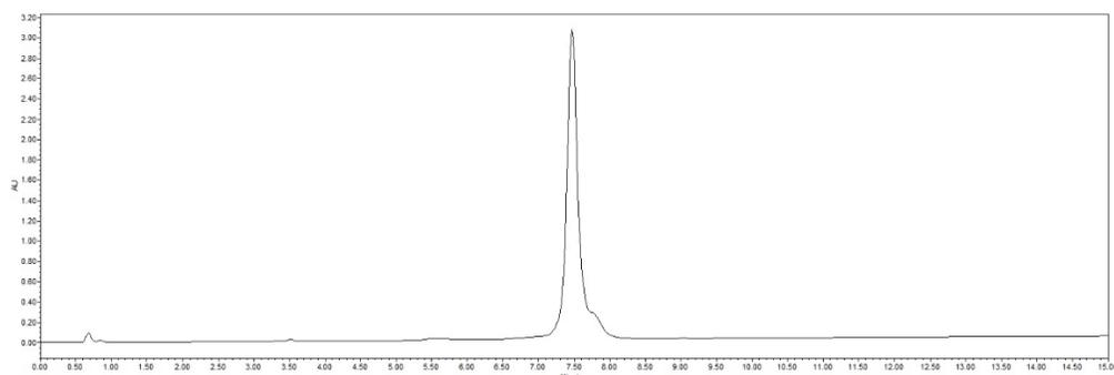
**Fig. S43** Analytical RP-HPLC trace of **21/23**:  $t_R = 7.47$  min ( $\lambda_{\text{max}} = 214$  nm, 5–60% B over 15 min).
