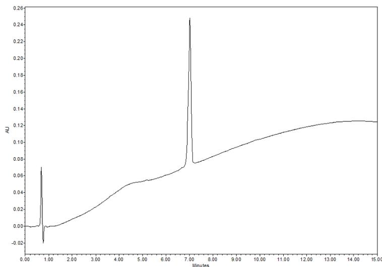
**Fig. S33** Analytical RP-HPLC trace of **18**:  $t_R = 7.03$  min ( $\lambda_{max} = 214$  nm, 5–100% B over 15 min).
