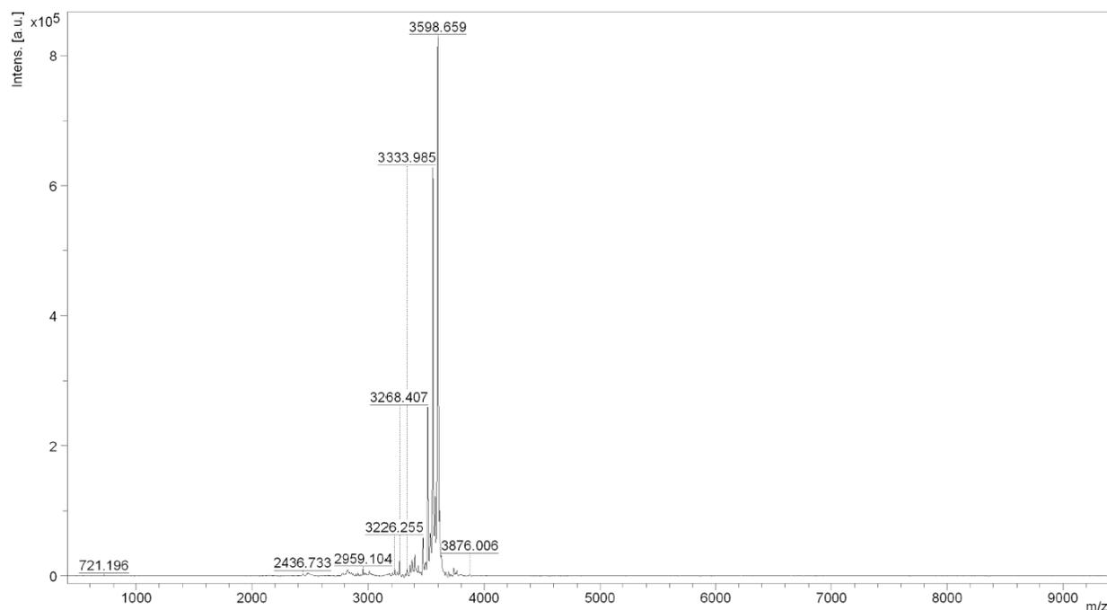
**Fig. S6** LRMS (MALDI-TOF) spectrum of glycodendrimer **1**:  $m/z$  calcd. for  $[M+Na]^+$  3597.7 (average), found 3598.7.
