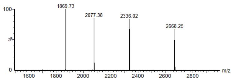
**Fig. S28** LRMS (ESI<sup>+</sup>-MS) spectrum of **15**:  $m/z$  calcd. for  $[M+7H]^{7+}$  2670.8 (average), found 2668.3; calcd. for  $[M+8H]^{8+}$  2336.6, found 2336.0; calcd. for  $[M+9H]^{9+}$  2077.1, found 2077.4; calcd. for  $[M+10H]^{10+}$  1869.5, found 1869.7.
