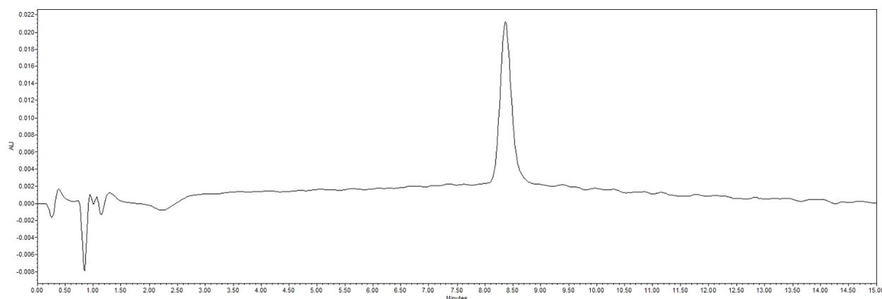
**Fig. S9** Analytical RP-HPLC trace of **3**:  $t_R = 8.37$  min ( $\lambda_{\text{max}} = 214$  nm, 0–40% B over 15 min).
