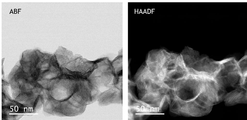
**Fig. S1 4.** ABF and HAADF images of the pristine NiFe-LDH-Seb at intermediate magnifications.
