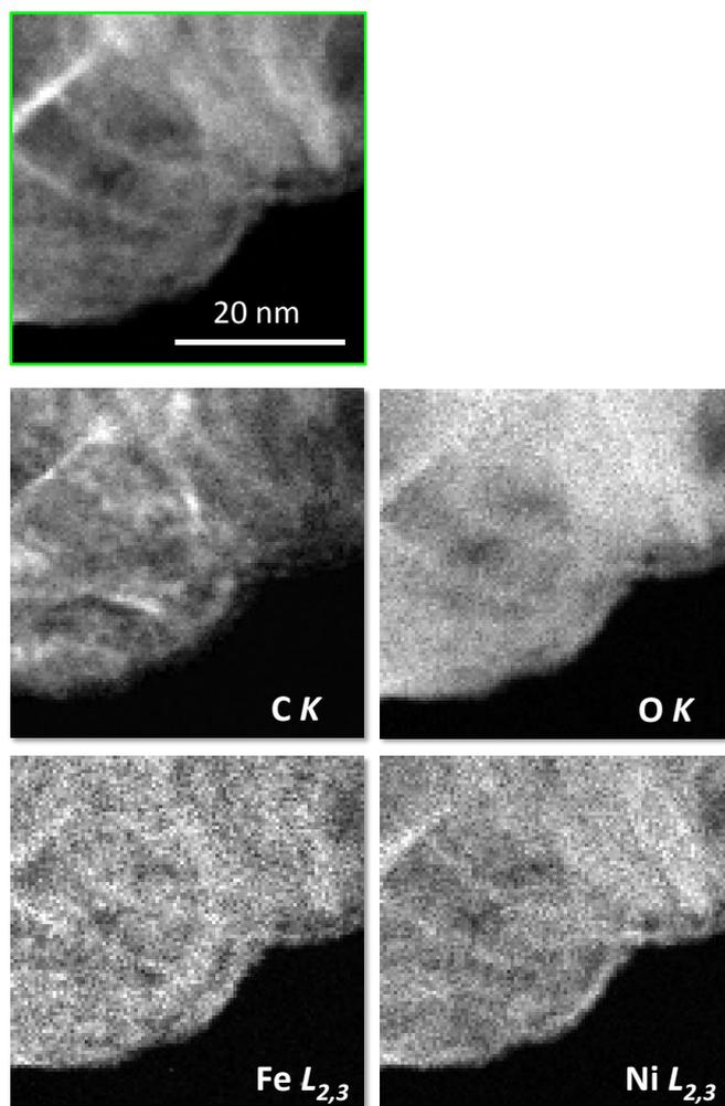
**Fig. SI 7** Electron energy-loss (EELS) compositional maps of the pristine NiFe-LDH-Seb at RT.
