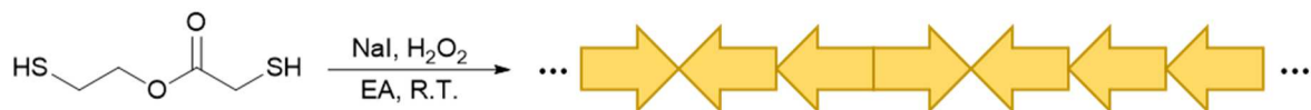
Figure S14. Scheme for the polycondensation of 2-mercaptoethyl-2-mercaptoacetate producing a polymer with randomly oriented repeating units. (0.3 M in ethyl acetate, 0.02 equiv. of NaI, 3 equiv. of H_2O_2 .)
