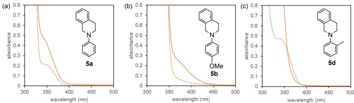
**Fig. S4** The absorption spectra of *N*-aryltetrahydroisoquinolines (**5a**, **5b**, and **5d**,  $1.0 \cdot 10^{-2}$  M, hashed line) and those in the presence of  $B(C_6F_5)_3$  ( $1.0 \cdot 10^{-2}$  M, solid line) in MeCN.
