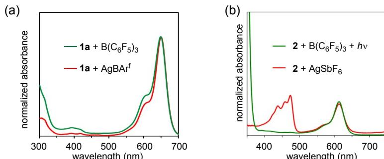
**Fig S3** (a) The absorption spectrum of  $B(C_6F_5)_3$  and **1a** after 1 h of stirring (green) in comparison with that of a mixture of  $AgBAr^f$  and **1a** (red). (b) The absorption spectrum of  $B(C_6F_5)_3$  and **2** after 405 nm LED irradiation for 3 h (green) in comparison with that of  $AgSbF_6$  and **2** after 2 h of stirring (red).
