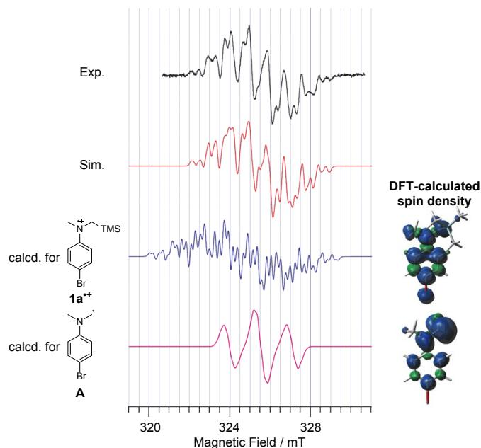
**Fig. S6** ESR spectra of the mixture of B(C<sub>6</sub>F<sub>5</sub>)<sub>3</sub> and **1a** in CH<sub>2</sub>Cl<sub>2</sub>, simulated spectrum (see Table S1 for the ESR parameters for the simulation), DFT-calculated spectrum for **1a<sup>•+</sup>**, and DFT-calculated spectrum of radical **A** with visualized spin density of **1a<sup>•+</sup>** and **A** (isovalue = 0.001). See also VI computational studies section for the details of DFT calculations.
