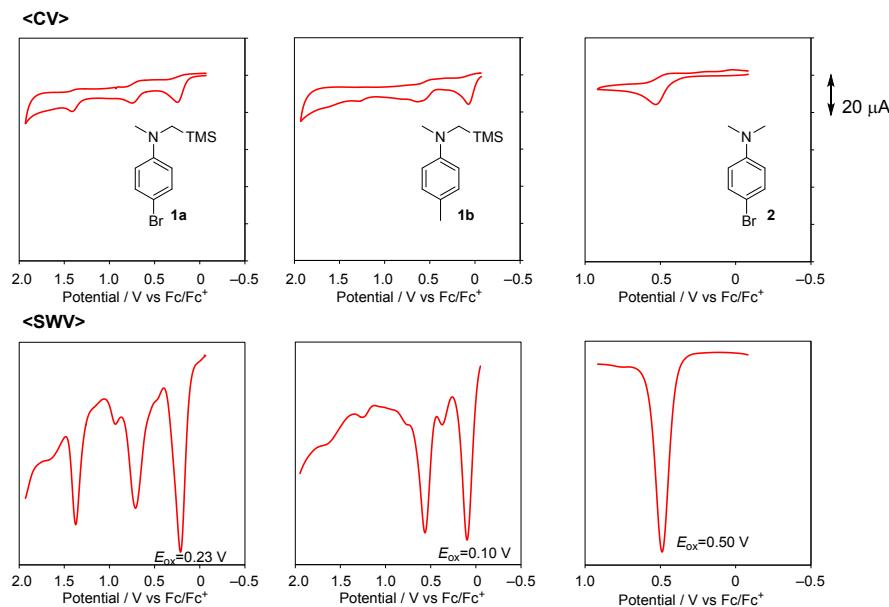
**Fig. S8** Cyclic voltammogram (upper) and square wave voltammogram (bottom) of **1a**, **1b**, and **2**.
