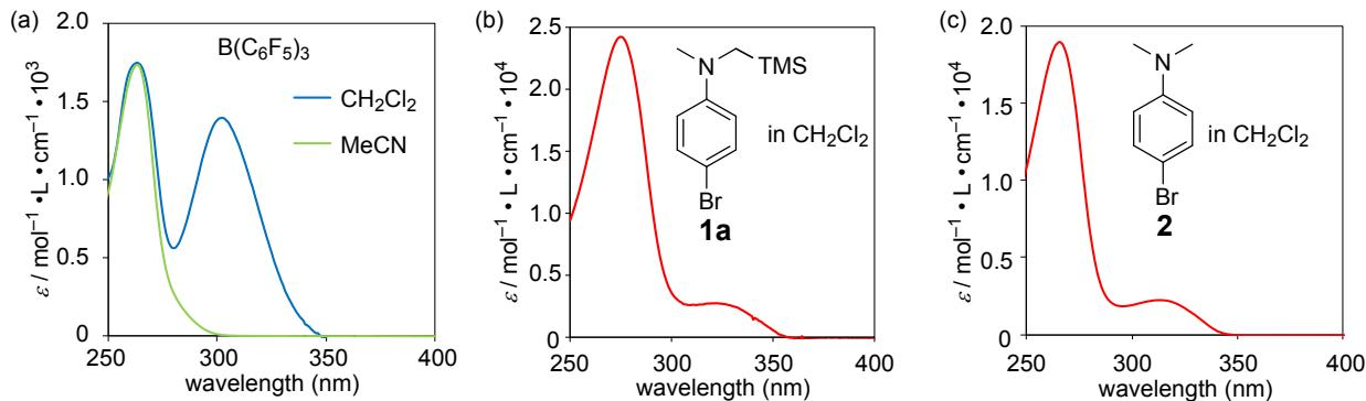
**Fig. S2** UV-vis absorption spectra of (a)  $B(C_6F_5)_3$  in  $CH_2Cl_2$  (blue) and MeCN (green); (b) **1a** in  $CH_2Cl_2$ ; (c) **2** in  $CH_2Cl_2$ . The difference in the absorption spectra of  $B(C_6F_5)_3$  recorded in MeCN and  $CH_2Cl_2$  is probably due to the coordination of MeCN to  $B(C_6F_5)_3$  as detected by <sup>11</sup>B NMR spectroscopy (see Fig. S20).
