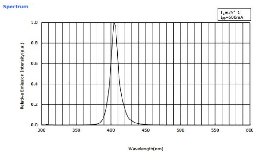
**Fig. S1** Emission spectrum of 405 nm LED element (provided from CCS inc).
