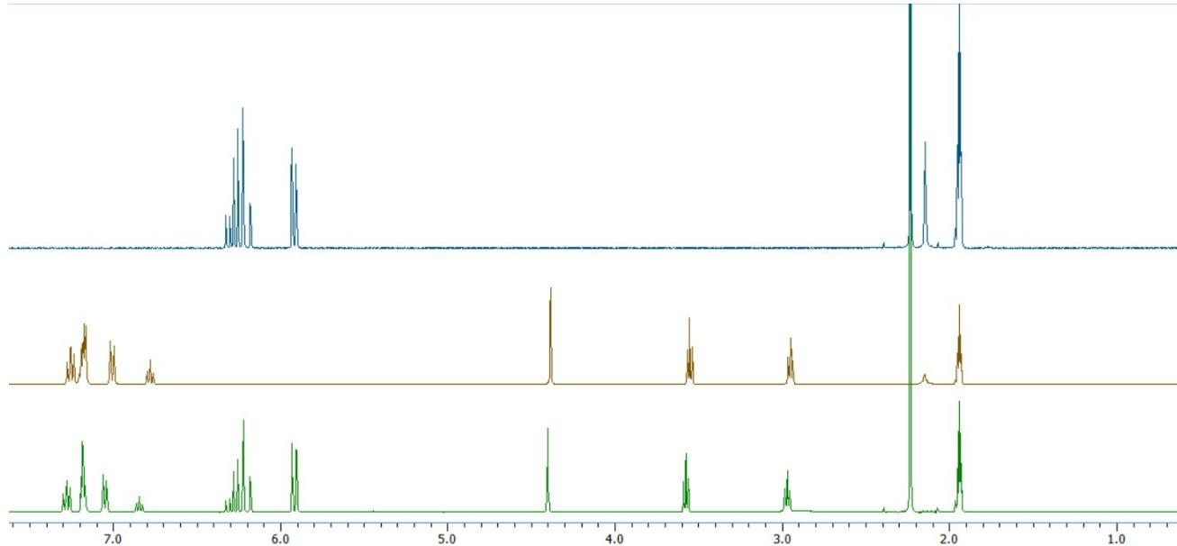
**Fig. S19** <sup>1</sup>H NMR spectra of methyl vinyl ketone **3a** (blue), **5a** (brown), and the reaction mixture (green) in the concentration reported in Table 2 (**3a**: 0.3 M, **5a**: 0.1 M, and B(C<sub>6</sub>F<sub>5</sub>)<sub>3</sub>: 0.01 M) (400 MHz, CD<sub>3</sub>CN).
