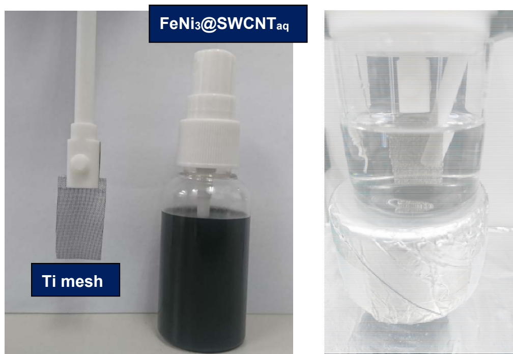
Fig. S14 \text{FeNi}_3\text{@SWCNT} ink loaded in a sprayer can homogeneously spray catalysts onto any conducting substrates for OER application.
