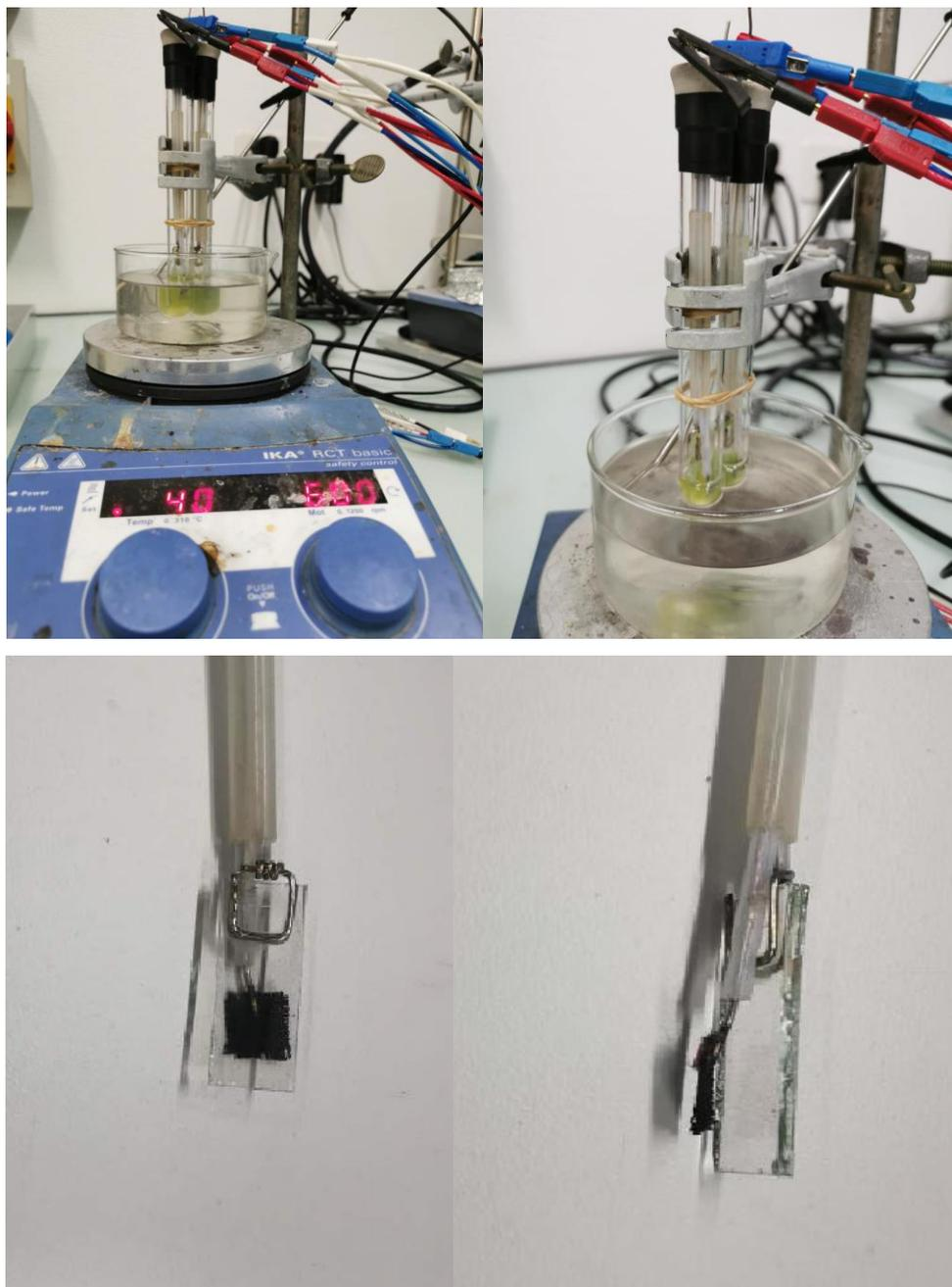
**Figure S1.** Undivided cell for the electrochemical reaction
