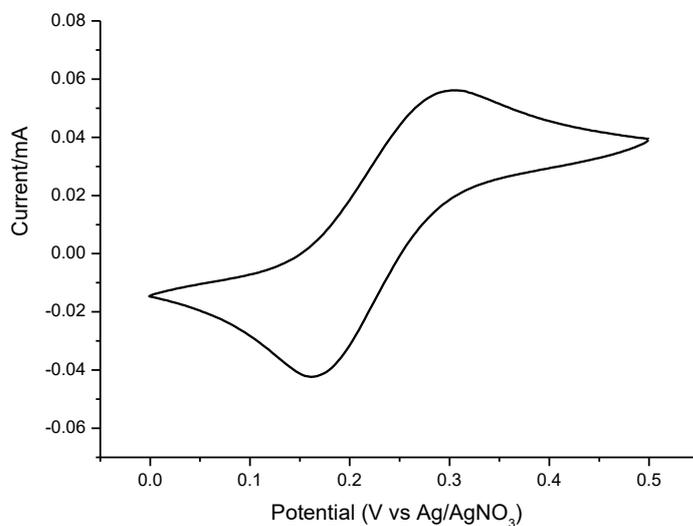
**Figure S2:** CV curve of ferrocene ( $5 \times 10^{-3}$  M) in THF/CH<sub>3</sub>CN (4:1, 2 mL) containing [LutH]ClO<sub>4</sub> (0.1 M) and lutidine (0.8 mmol). Glassy carbon electrode was used as a working electrode with a Ag/AgNO<sub>3</sub> reference electrode and a Pt counter electrode. Scan rate: 50 mV/s.
