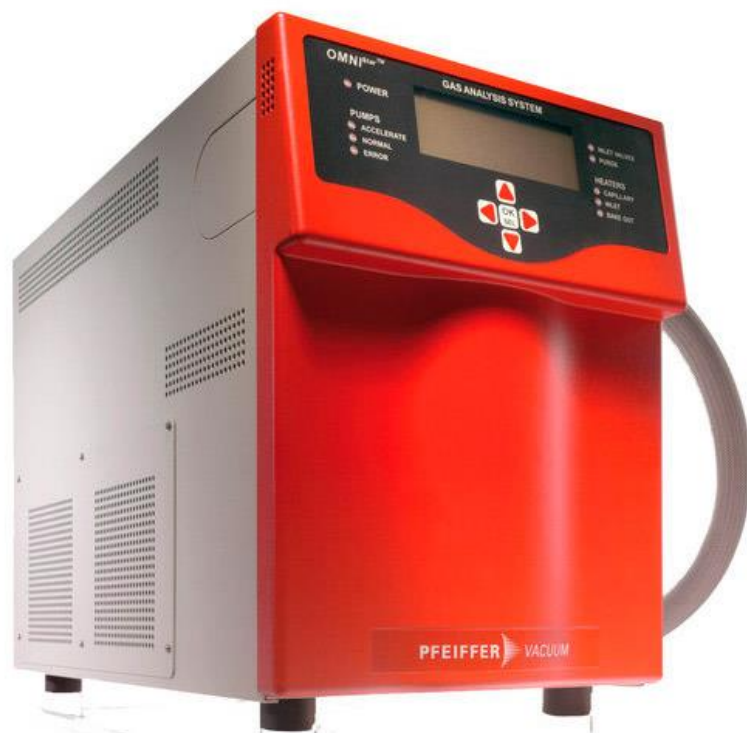
Figure S13. Photograph of OmniStar™ Gas Analysis System GSD 320 (Pfeiffer) quadrupole mass spectrometer apparatus used for the analysis of gases based on following their masses.
