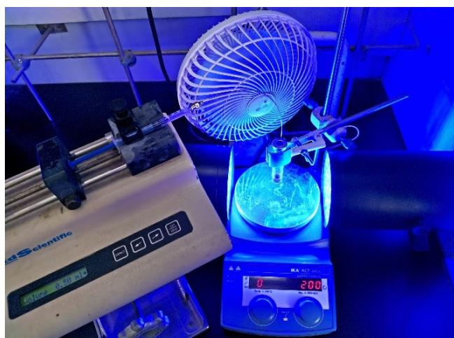
**Supplementary Figure 1.** Experimental setup for photocatalytic oxyarylation of olefins.
