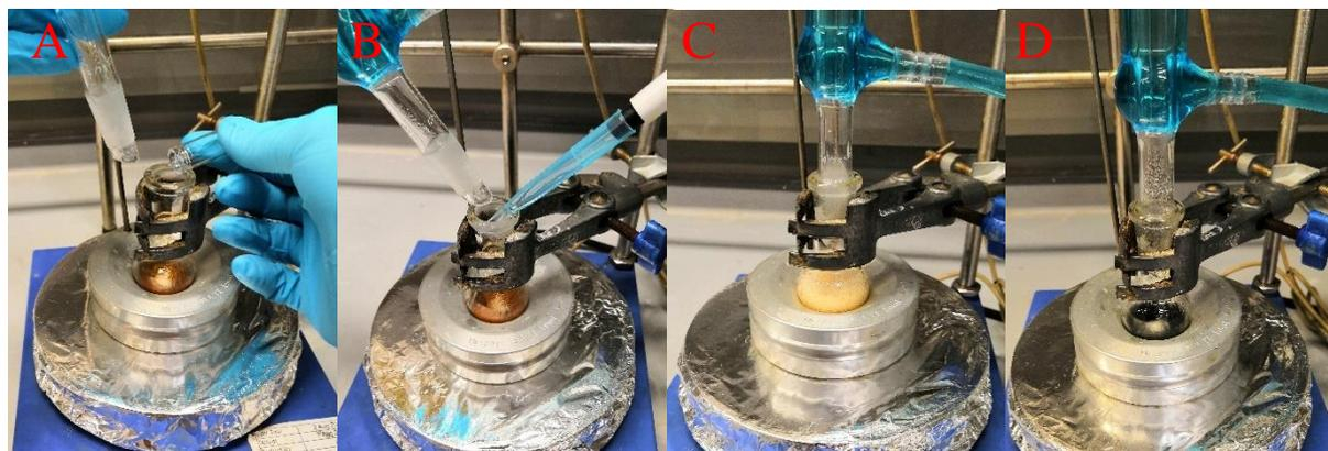
**Figure S2.** a) Addition of zinc acetate to the reaction mixture by temporary removal of the condenser. b) Addition of further phenylsilane to the reaction mixture. c) Resulting  $H_2$  evolution after addition of zinc acetate and phenylsilane. d) Characteristic colour change to black signalling the end-point of the reaction after 2 h / 6 h stirring at reflux.
