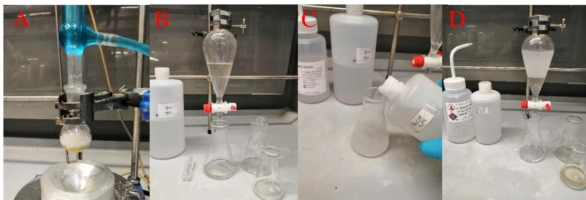
**Figure S3.** a) Reaction mixture after the addition of HCl / acetic acid (1 mL of a 3 M aqueous solution) to quench the reaction. b) Extraction of the product with HCl / acetic acid (3 M aqueous solution). c) Addition of NaOH (6 M aqueous solution) to the combined aqueous layers until pH12 was reached. d) Re-extraction of the product using  $\text{CH}_2\text{Cl}_2$ . The discarded organic layer can be seen on the right hand side.
