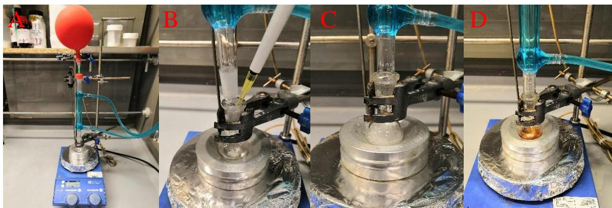
**Figure S1.** a) A typical reductive amination reaction set up using standard laboratory glassware and an argon balloon. b) Addition of phenylsilane to the solution of carboxylic acid in toluene by temporary removal of condenser. c)  $H_2$  evolution after the dropwise addition of amine to the reaction mixture. d) Amidation phase of the reaction after stirring at reflux for 16 h.
