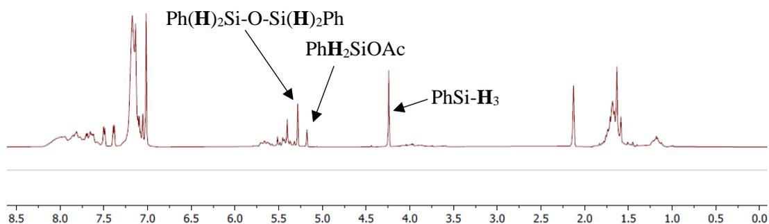
**Figure S7.**  $^1\text{H}$  NMR spectrum crude phenylsilyl acetate **39**.
