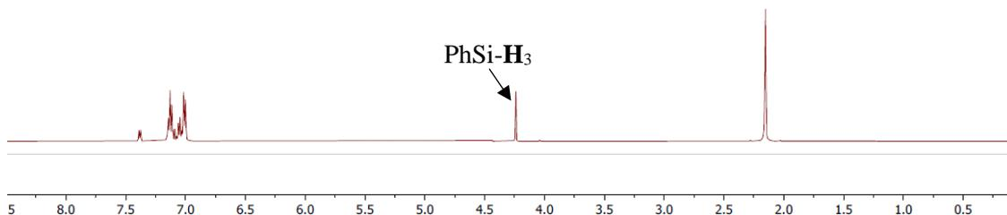
**Figure S6.**  $^1\text{H}$  NMR spectrum of the zinc acetate and phenylsilane crude reaction mixture.
