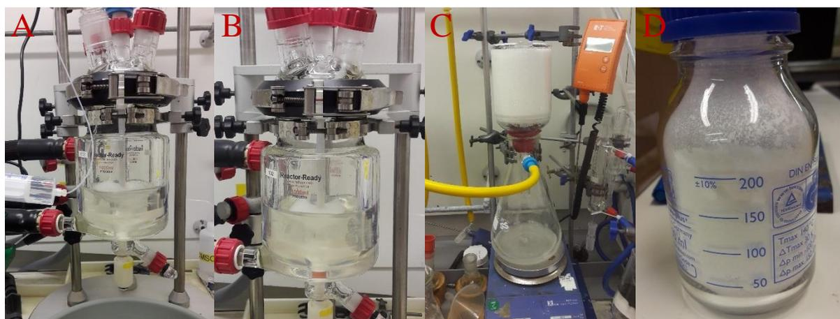
**Figure S5.** a) Reaction set-up using jacketed reaction vessel. Hydrogen effervescence visible from the slow addition of silane (2 mL/min) during the amidation phase of the reaction. b) After zinc acetate and further silane addition for the reduction phase of the reaction. c) Filtration of the hydrochloride salt. d) Product after filtration and drying.
