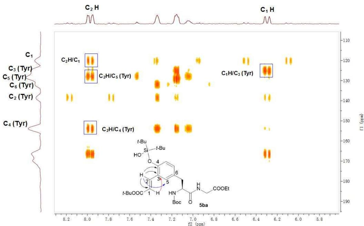
Figure S8. Determination of the olefination site on Tyr residue in product **5ba** by HMBC.
