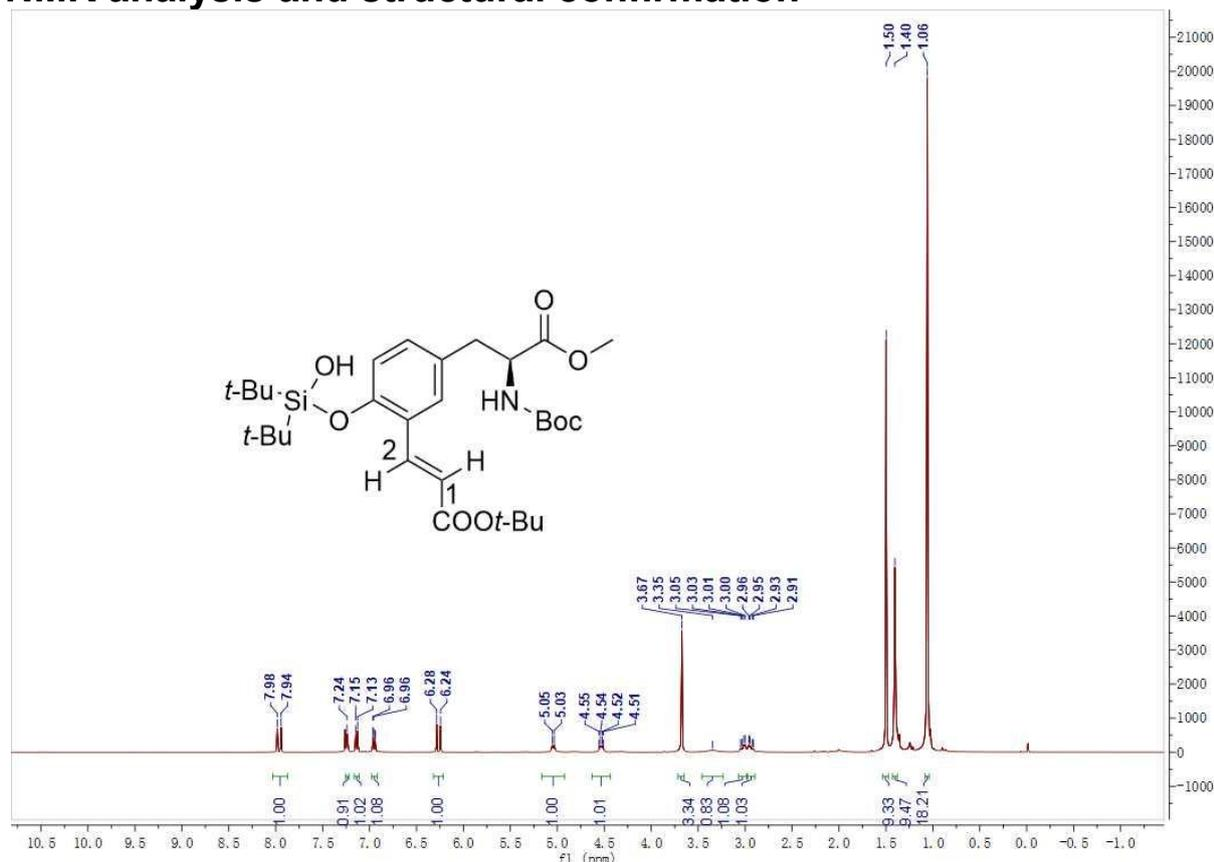
**Figure S5.** Determination of the configuration of exocyclic double bond in product **3aa** by  $^1\text{H}$  NMR (400 MHz,  $\text{CDCl}_3$ ). The coupling constant was  $J_{\text{H}_1, \text{H}_2} = 16.0$  Hz, and therefore the double bond is in *E*-configuration.
