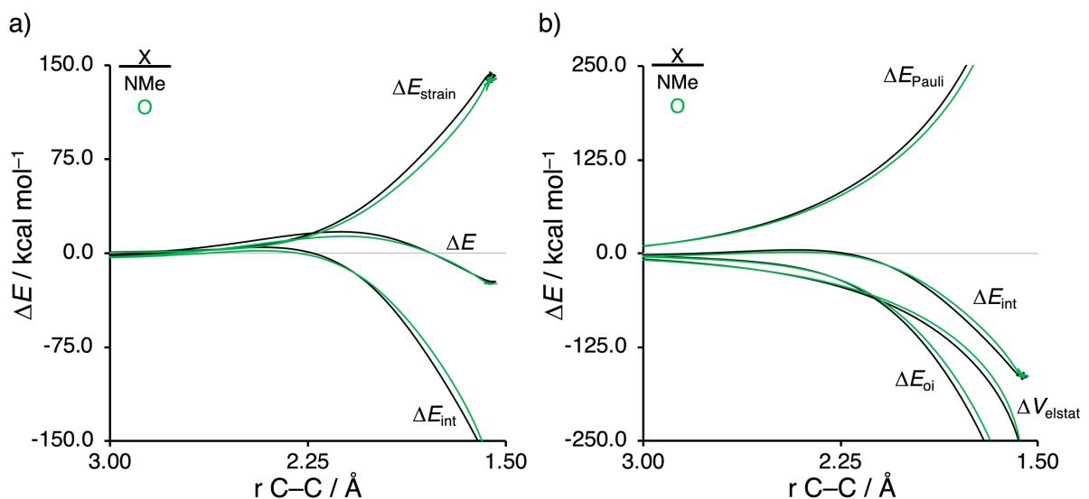
**Figure S5.** a) Activation strain analyses and b) energy decomposition analyses of the Diels-Alder reactions between the **CP** and **O** and **NMe** going from the reactants to the products, where the energy values are projected onto the shorter newly forming  $\text{C}_{\text{CP}}^{\bullet\bullet\bullet}\text{C}_\beta$  bond between **CP** and the dienophile, computed at ZORA-M06-2X/TZ2P//M06-2X/def2-TZVP.
