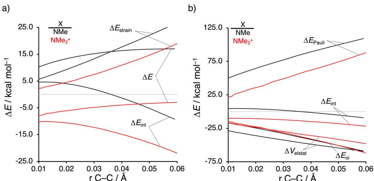
**Figure S4.** a) Activation strain analyses and b) energy decomposition analyses of the Diels-Alder reactions between the **CP** and **NMe** and **NMe<sub>2</sub><sup>+</sup>** going from the reactants to the transition states, where the energy values are projected onto the stretch of the C<sub>α</sub>•••C<sub>β</sub> bond of the dienophile, computed at ZORA-M06-2X/TZ2P//M06-2X/def2-TZVP.
