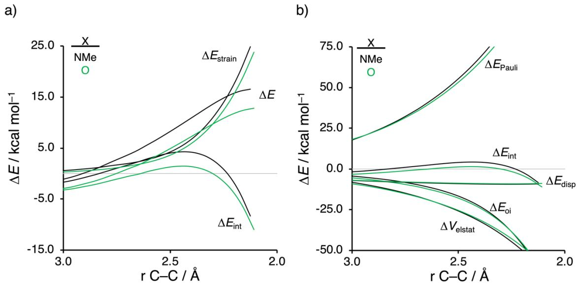
**Figure S8.** a) Activation strain analyses and b) energy decomposition analyses of the Diels-Alder reactions between the **CP** and **O** and **NMe** going from the reactants to the transition states, where the energy values are projected onto the shorter newly forming  $\text{C}_{\text{CP}} \cdots \text{C}_\beta$  bond between the **CP** and the dienophile, computed at ZORA-B3LYP-D3(BJ)/TZ2P//M06-2X/def2-TZVP.
