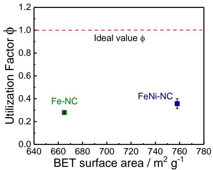
**Figure S4.** The active-site utilization factor  $\phi_{SD \text{ surfac/bulk}}$  as a function of Brunauer-Emmett-Teller (BET) surface area.
