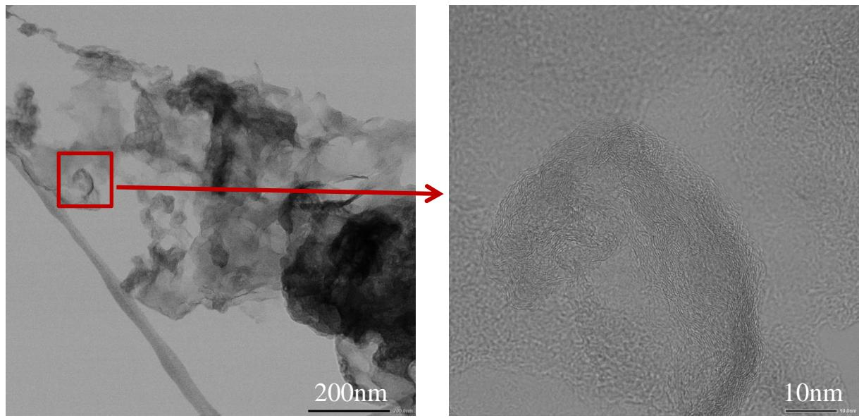
**Figure S2.** STEM-BF image images of the carbon phase of FeNi-NC catalyst.
