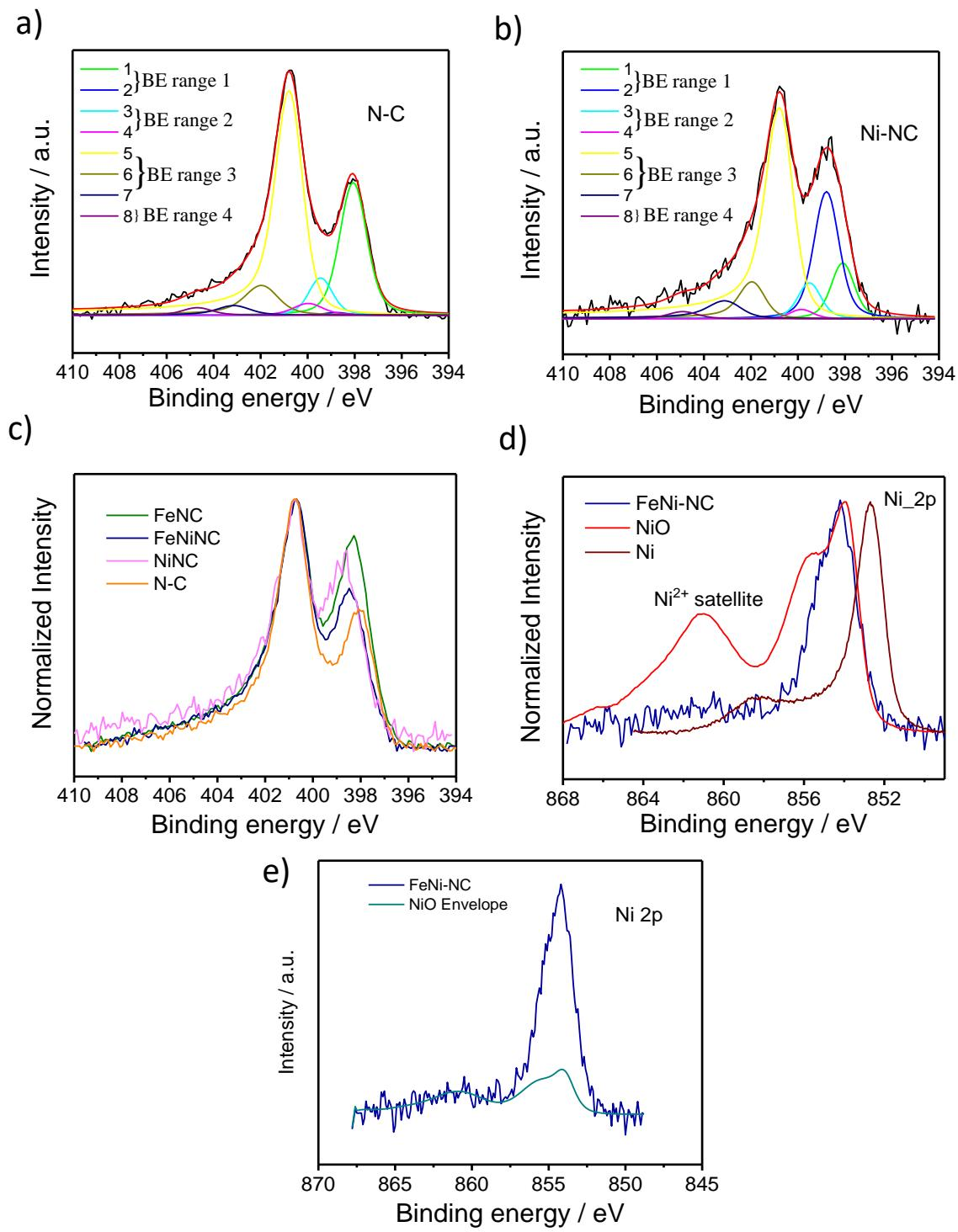
**Figure S1.** XPS analyses of N-C and Ni-NC catalysts. XPS-N<sub>1s</sub> spectrum of (a) N-C and (b) Ni-NC, (c) The comparison of high-resolution N 1s XPS for all the catalyst, (d) XPS-Ni<sub>2p</sub> spectra of FeNi-NC, NiO and Pure Ni, (e) The comparison of experimental Ni2p spectra of FeNi-NC and expected Ni2p spectra of NiO envelope.
