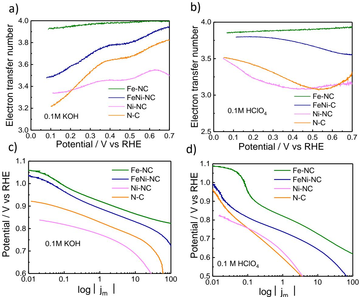
**Figure S3.** Electron transfer for Fe-NC, FeNi-NC, Ni-NC and N-C in (a) alkaline and (b) acidic electrolyte. Electrochemical Tafel curves of MNC catalysts (applied E versus  $\log|j_m|$  ( $j_m$ : kinetic mass activity / mA mg<sup>-1</sup>)) in (c) alkaline and (d) acid electrolyte.
