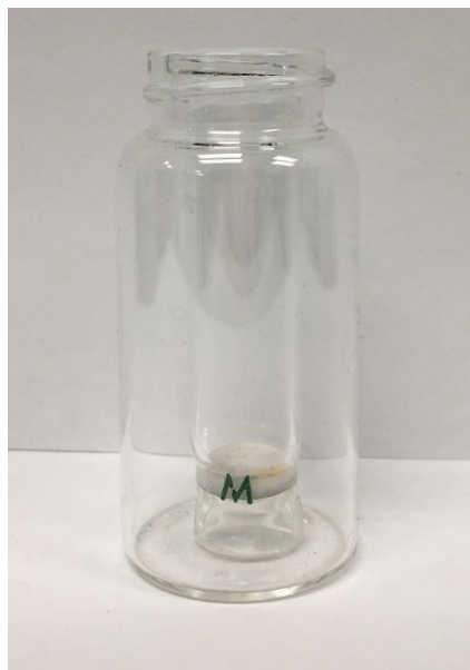
Figure S2. Image of the custom-made frit used to house single crystals of \text{Fe}_2(\text{bdp})_3 for stoichiometric reduction with lithium naphthalenide.
