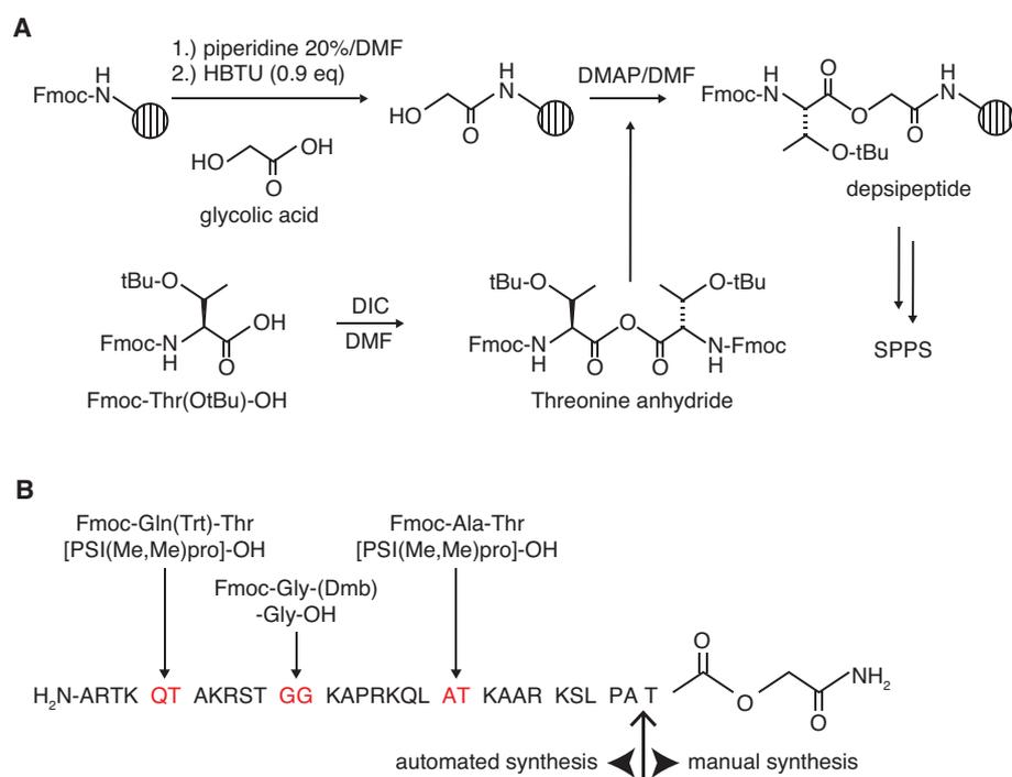
**Fig. S12:** Formation of depsipeptide bond and H3 depsipeptides. **(A)** Depsipeptide bonds between glycolic acid and Threonine were formed by coupling glycolic acid to the solid support followed by coupling of Fmoc-Thr(otBu)-OH as symmetric anhydride under 4-dimethylaminopyridine (DMAP) catalysis. **(B)** H3 depsipeptide synthesis was facilitated by installation of pseudoproline and Dmb dipeptide building blocks during synthesis at the indicated positions.
