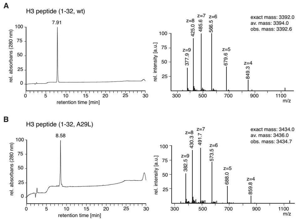
**Fig. S15: LC-MS analysis of H3 peptides used in this study.** The peptides were used for establishing nucleosomal ligations in solution (see Fig. S1). The H3 depsipeptide (1-32, A29L) is identical to pep19 (Fig. S9 P).
