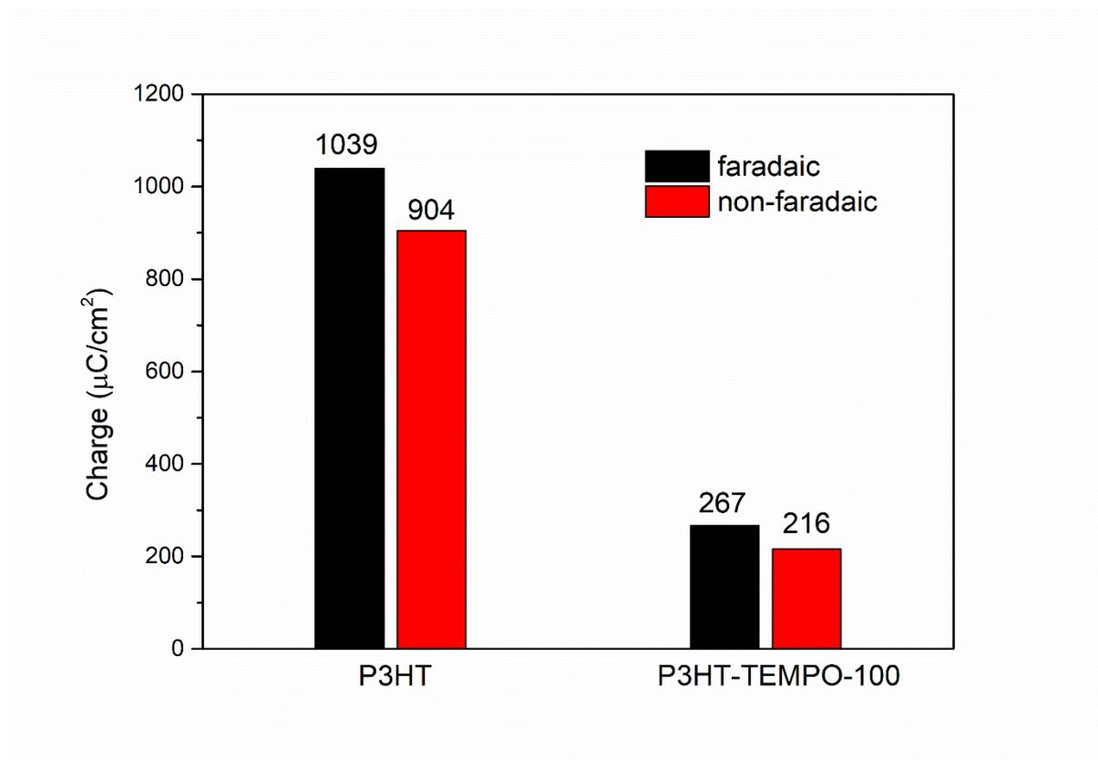
**Figure S2.** Faradaic vs. non-faradaic contributions to charge transfer for P3HT and P3HT-TEMPO-100 thin film electrodes.
