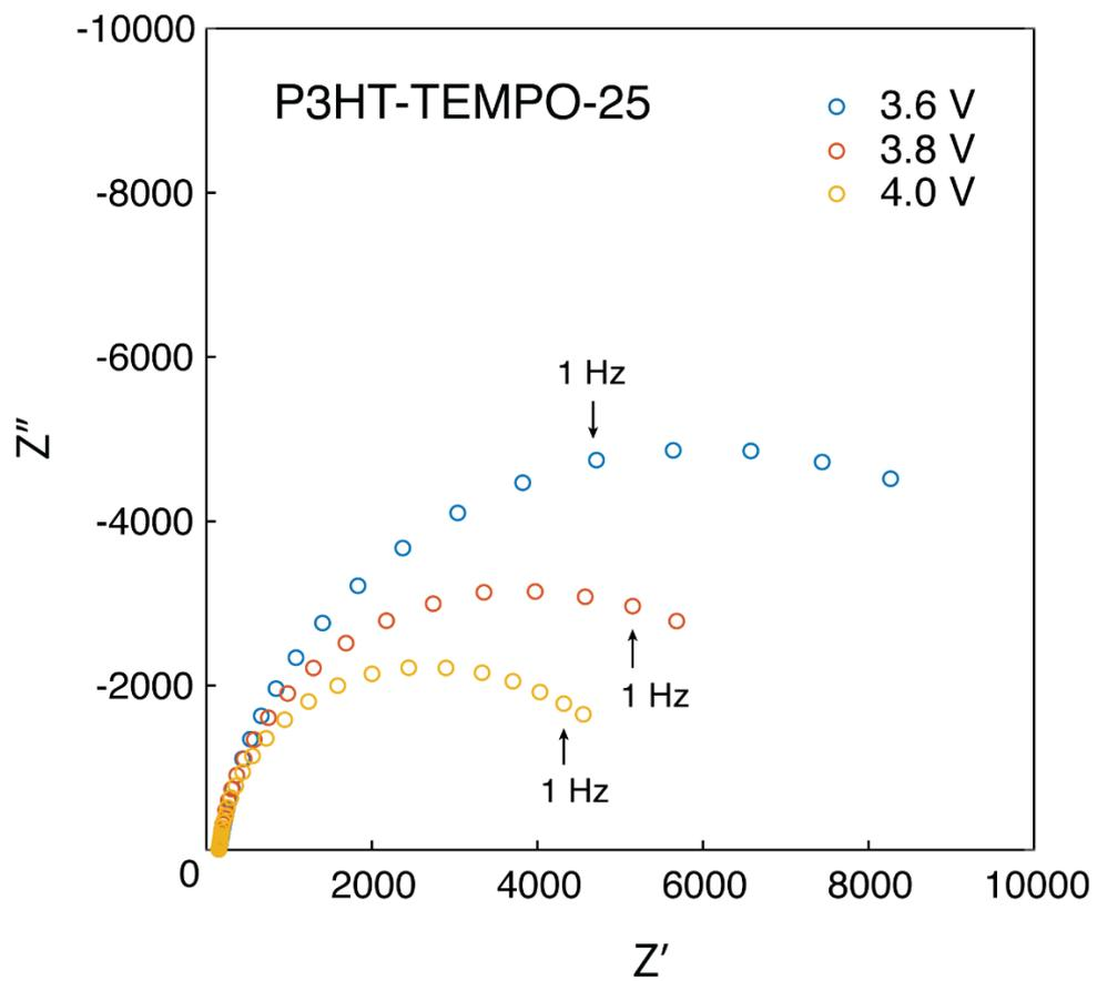
**Figure S4.** Electron impedance spectroscopy of P3HT-TEMPO-25.
