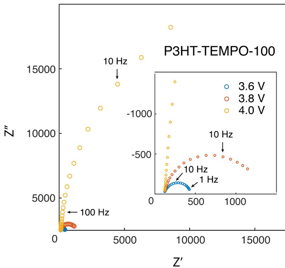
**Figure S5.** Electron impedance spectroscopy of P3HT-TEMPO-100.
