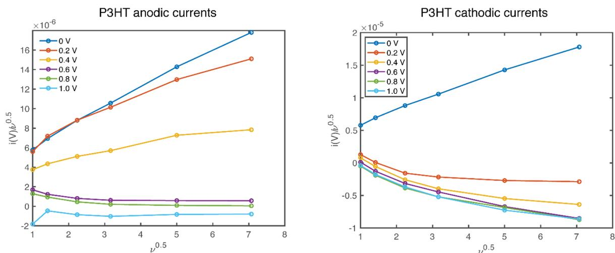
**Figure S1.** Example of deconvolution for the faradic and non-faradic current response.
