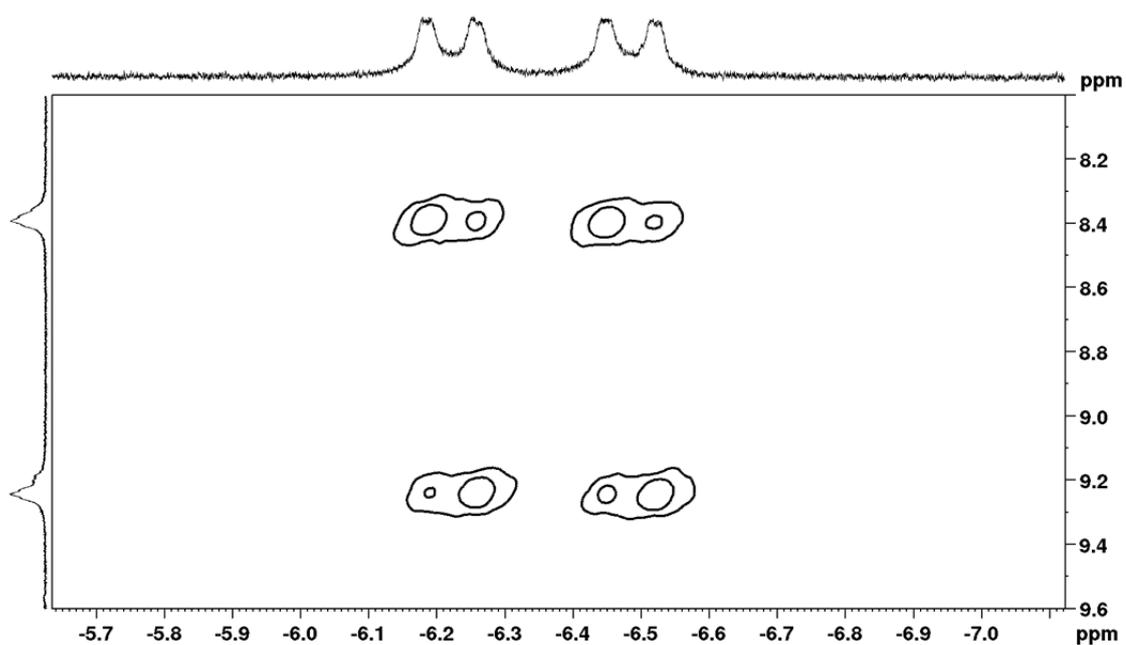
Figure S24. Expansion of the  $^1\text{H}$ -EXSY NMR spectrum of **2** in  $\text{C}_6\text{D}_6$  showing the exchange cross-peak between PH and CrH signals.
