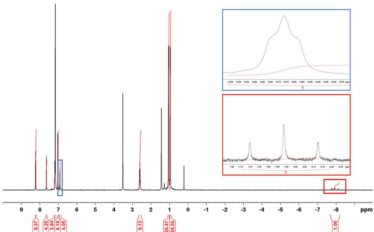
Figure S31.  $^1\text{H}$  NMR spectrum of **5**[ $\text{BAr}_4^f$ ] in  $\text{C}_6\text{D}_6/\text{THF-D}_8$  5:1 with expansions showing the regions of the CrH and NCH signals.
