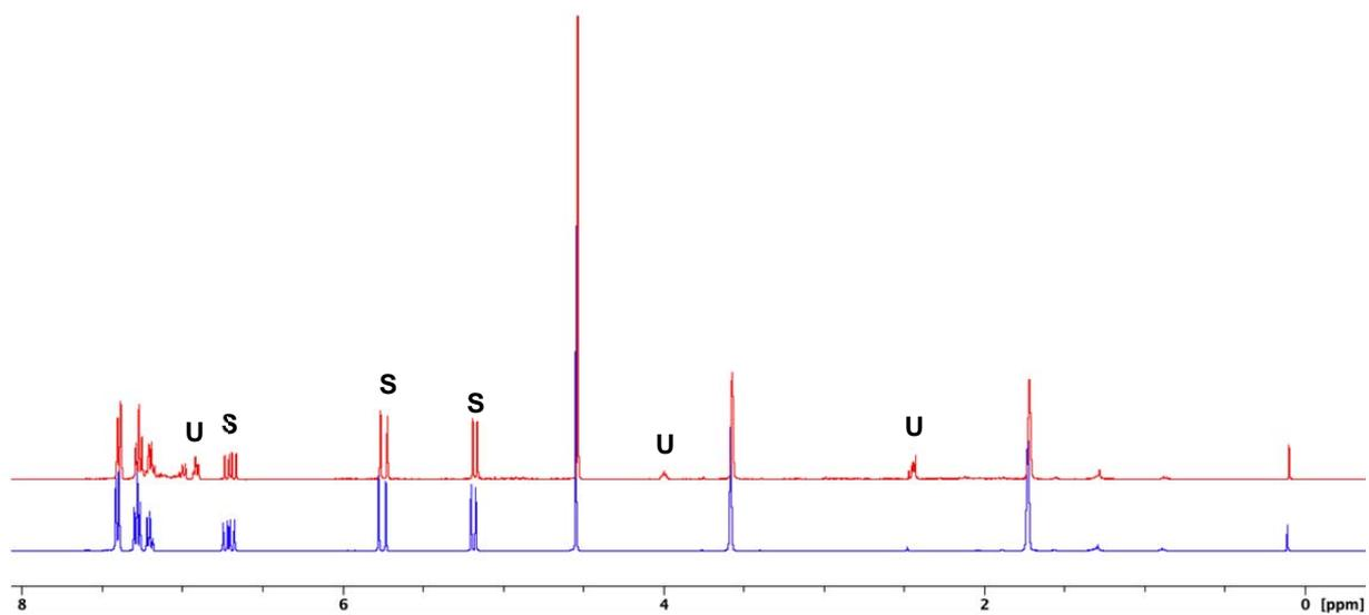
**Figure S22.**  $^1\text{H}$  NMR spectra of a solution of styrene in  $\text{THF-D}_8$  under 8 atm of  $\text{H}_2$  before (blue trace) and after 17 h of irradiation with a medium pressure Hg lamp (red trace). Labelled signals are attributable to styrene (S) and an unidentified by-product (U).
