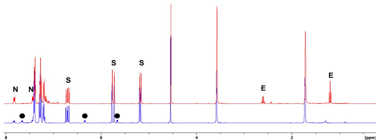
**Figure S20.**  $^1\text{H}$  NMR spectra of a solution of styrene and  $[\text{Cr}(\text{CO})_3(\text{naphthalene})]$  in  $\text{THF-D}_8$  under 8 atm of  $\text{H}_2$  before irradiation (blue trace) and after 17h of irradiation with a medium pressure Hg lamp (red trace). Labelled signals are attributable to styrene (S), ethylbenzene (E),  $[\text{Cr}(\text{CO})_3(\text{naphthalene})]$  (circle) and naphthalene (N).
