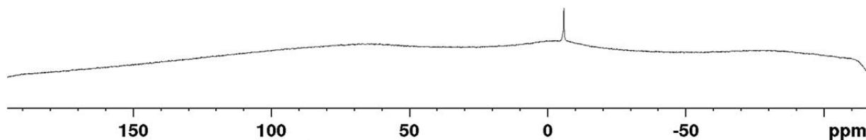
Figure S34.  $^{11}\text{B}\{^1\text{H}\}$  NMR spectrum of  $5[\text{BAr}_4^f]$  in  $\text{C}_6\text{D}_6/\text{THF-D}_8$  5:1.
