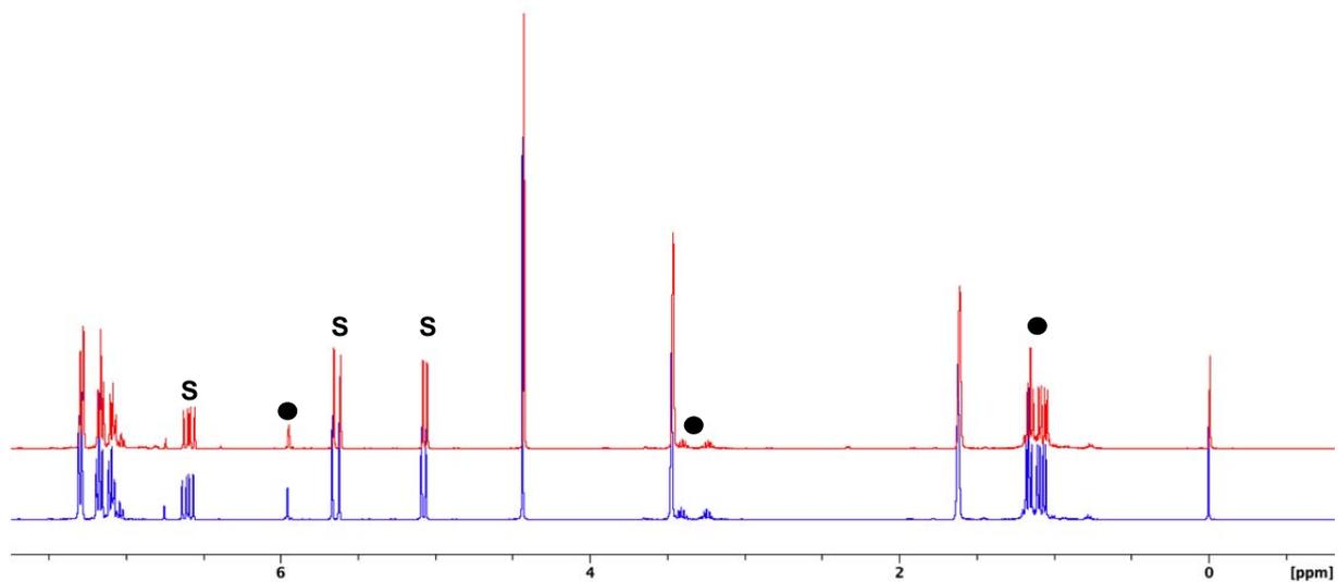
**Figure S21**  $^1\text{H}$  NMR spectra of a solution of styrene and **1** in  $\text{THF-D}_8$  under 8 atm of  $\text{H}_2$  before (blue trace) and after 17h of irradiation with a medium pressure Hg lamp (red trace). Labelled signals are attributable to styrene (S) and **1** (circle).
