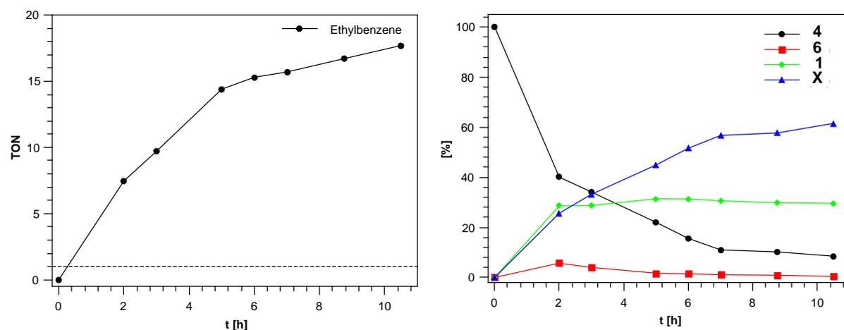
**Figure S17.** Kinetic plot showing the time evolution of ethylbenzene (left) and phosphorus-containing species (right) during photohydrogenation of styrene in the presence of 4 mol-% of **4** (TON =  $n(\text{Ethylbenzene})/n(\mathbf{4})_{t=0}$ ).
