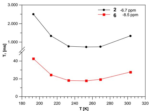
**Figure S36.**  $T_1$  relaxation times for the hydride signals of **2** and **6** determined by the inversion-recovery method at different temperatures. Minimum values (at 253 K):  $T_{1,\min} = 18$  ms (**6**), 739 ms (**2**).
