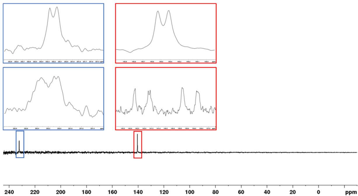
**Figure S25.**  $^{31}\text{P}\{^1\text{H}\}$  NMR spectrum of **2** in  $\text{C}_6\text{D}_6$  (bottom trace). Framed inserts display expansions of the two signals in the  $^{31}\text{P}\{^1\text{H}\}$  (top row) and  $^{31}\text{P}$  (bottom row) NMR spectrum.
