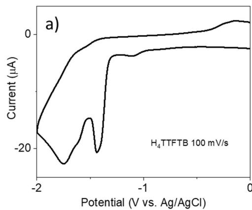
**Figure S6.** CV data collected on the reduction side for  $\text{H}_4\text{TTFTB}$  in  $\text{N}_2$  purged 0.1M  $\text{TBAPF}_6$  at 100 mV/s. The working electrode is glassy carbon.
