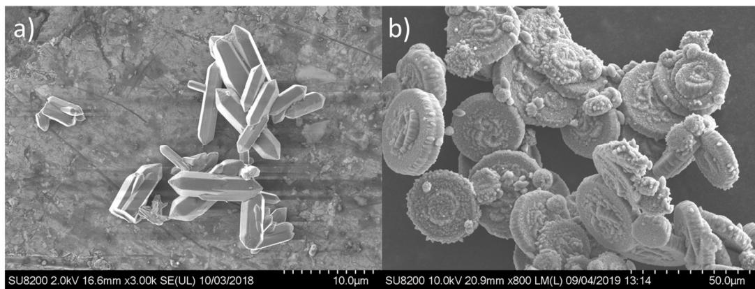
**Figure S4.** SEM images of (a)  $\text{Zn}_2\text{TTFTB}$  powder synthesized under the standard synthesis conditions containing added  $\text{H}_2\text{O}$  and (b)  $\text{Zn}_2\text{TTFTB}$  powder synthesized under the film conditions without added  $\text{H}_2\text{O}$  and also with a larger  $\text{Zn:TTFTB}$  ratio than the standard synthesis.
