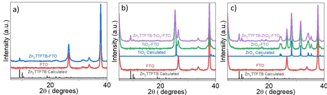
**Figure S1.** pXRD patterns comparing the calculated Zn<sub>2</sub>TTFTB film samples to the patterns for the substrate(s) for Zn<sub>2</sub>TTFTB-FTO (a), Zn<sub>2</sub>TTFTB-TiO<sub>2</sub> (b), and Zn<sub>2</sub>TTFTB-ZrO<sub>2</sub> (c).
