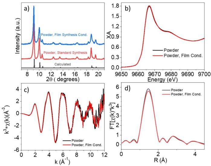
**Figure S2.** (a) pXRD patterns comparing the polycrystalline powder sample obtained from the standard published synthesis to the powder synthesized under the film synthesis condition. (b) Zn K-edge XANES spectra comparing the two synthesis conditions. (c) K-space and (d) R-space comparisons of the two synthesis methods.
