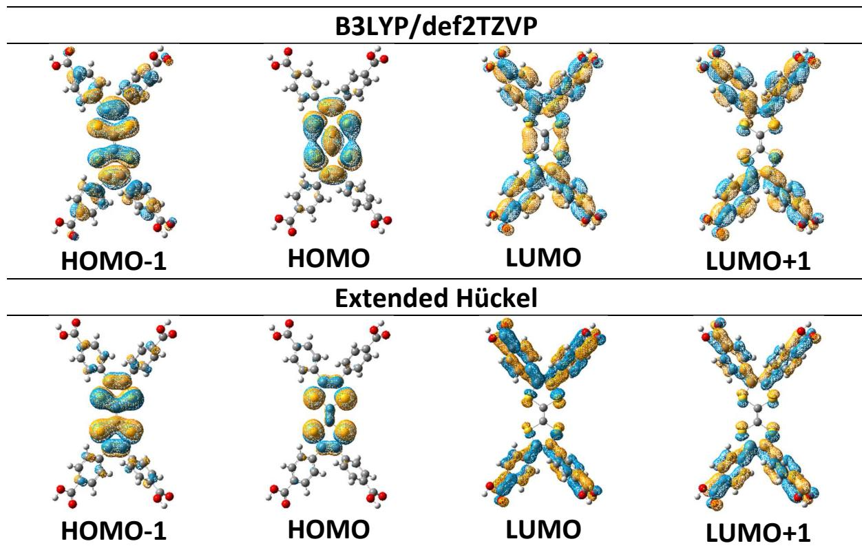
**Figure S20.** Comparison of the molecular orbital topologies at the DFT (B3LYP/def2TZVP) and Extended Hückel (EH) levels for the H<sub>4</sub>TTFTB ligand. The parameters of the EH Hamiltonian were optimized to closely reproduce the symmetries and HOMO-LUMO gap of the DFT orbitals. The HOMO-LUMO gap at the DFT and EH levels are 2.56 and 3.15 eV, respectively.
