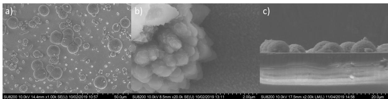
**Figure S5.** SEM results for  $\text{Zn}_2\text{TTFTB-FTO}$ . Top-view images (a,b) and cross-section image (c) show the formation of a monolayer of hemispherical flower-like MOF structures.
