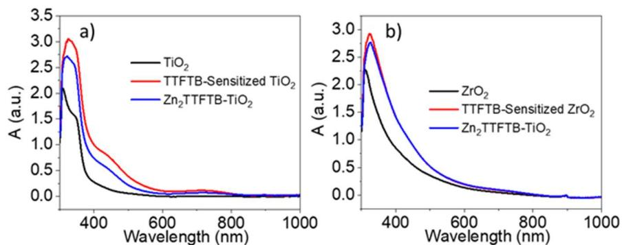
**Figure S14.** Transmission mode UV-Visible spectra for TiO<sub>2</sub> samples (a), ZrO<sub>2</sub> samples (b). The cation radical band is observed clearly in the TTFTB-Sensitized TiO<sub>2</sub> sample (a). Additionally, it is observed in the diffuse reflectance spectrum of H4TTFTB powder (c). Evidently, oxidation occurs when the ligands are aggregated in either the solid powder, on a sensitized film, or in the MOF structure.
