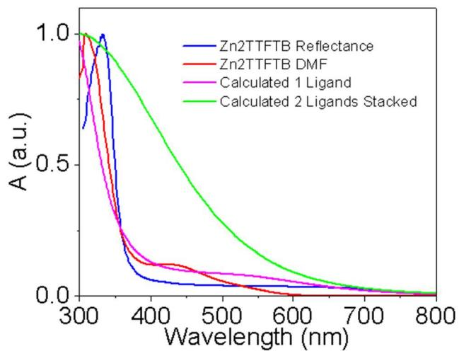
**Figure S12.** Comparison of 2 ligand stacked model to experimental and theoretically calculated single ligand UV-Visible spectra. The 2 ligand shows absorption broadening between the 400–600 nm region but does not show a prominent feature in the 600 – 800nm region seen in the MOF and cation structures.
