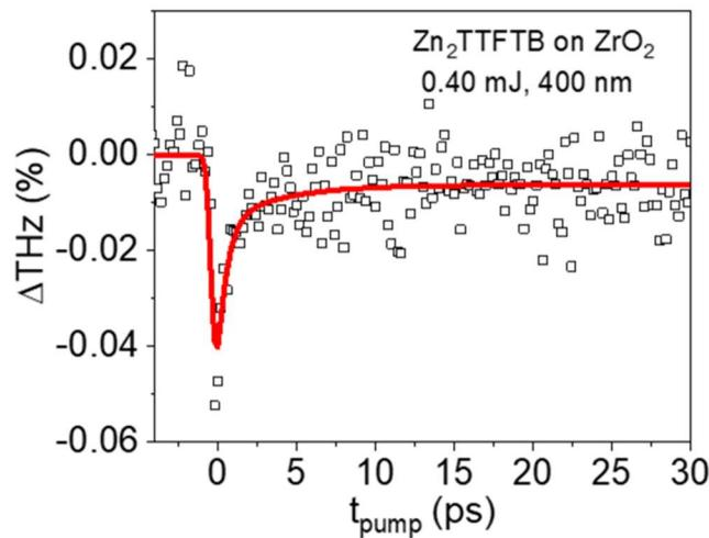
**Figure S16.** Control experiment for  $\text{Zn}_2\text{TTFTB}$  on  $\text{ZrO}_2$  under 400nm excitation. The intrinsic photoconductivity of the MOF is over an order of magnitude weaker than the observed injection signal and is therefore disregarded in modelling.
