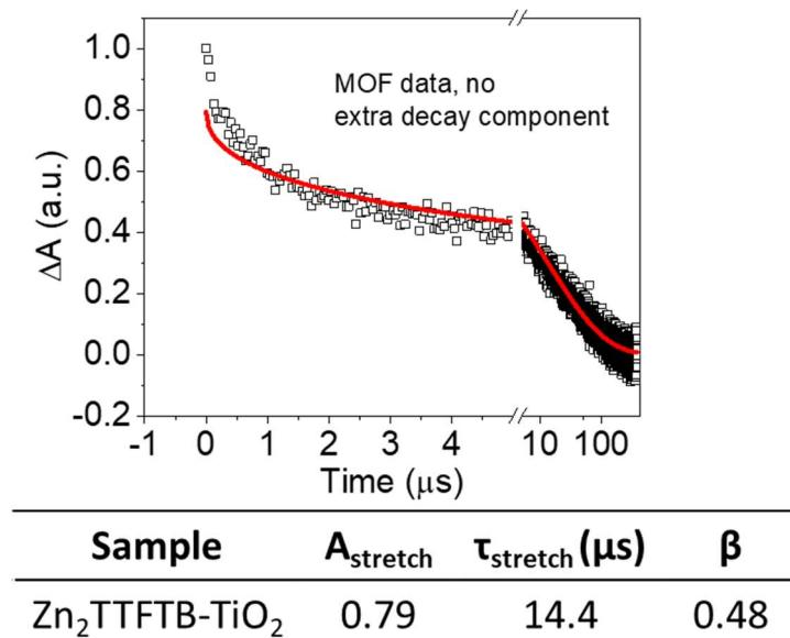
**Figure S18.** Fitting of  $\text{Zn}_2\text{TTFTB-TiO}_2$  ns-TA data with a single stretched exponential.
