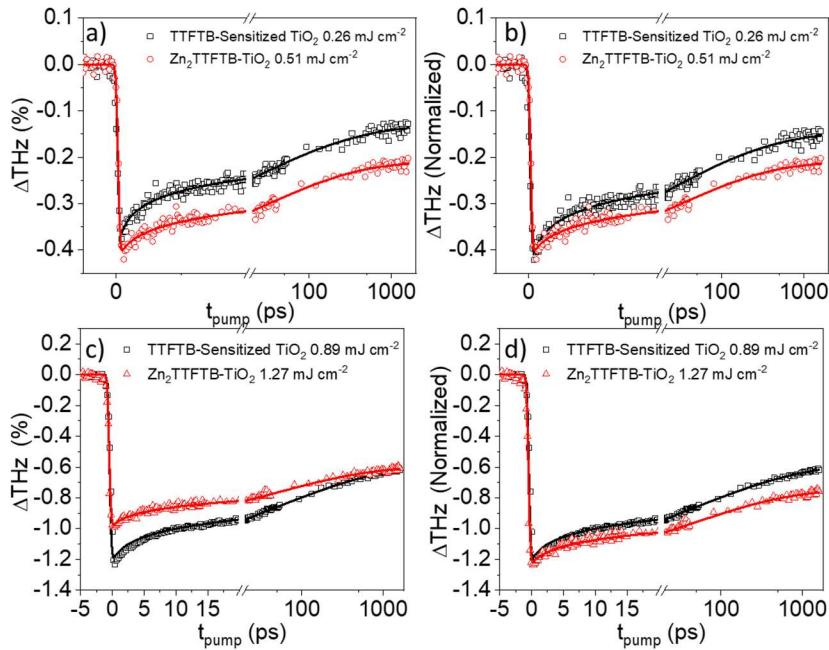
**Figure S17.** OPTP comparisons of TTFTB-Sensitized  $\text{TiO}_2$  to  $\text{Zn}_2\text{TTFTB-TiO}_2$  at similar  $\Delta\text{THz}$  attenuation magnitudes. Unnormalized (a) and normalized (b) comparisons at  $0.26 \text{ mJ cm}^{-2}$  and  $0.51 \text{ mJ cm}^{-2}$ , respectively. Unnormalized (c) and normalized (d) comparisons at  $0.89 \text{ mJ cm}^{-2}$  and  $1.27 \text{ mJ cm}^{-2}$ , respectively.
