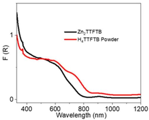
**Figure S8.** Diffuse reflectance UV-Visible-NIR spectra for  $Zn_2$ TTFTB powder and  $H_4$ TTFTB powder. Both display absorption in the region between 600-nm corresponding to TTF cation radical absorption.
