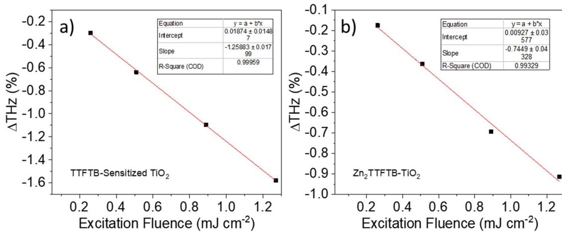
**Figure S15.** Linear dependence of the THz attenuation amplitude on the 400 nm pump fluence.
