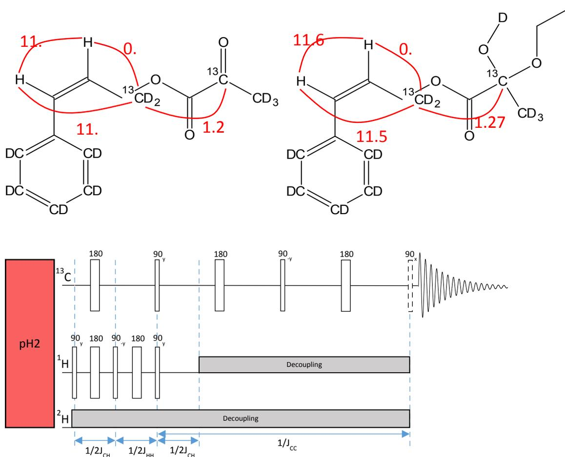
Figure S4. Top:  $J$ -coupling network of two structures (oxo form on the left and semiketal on the right) present after para-hydrogenation and during the polarization transfer.  $J$ -couplings relevant for the polarization transfer are  $J_{HH}=11.6$  Hz,  $J_{CH}=11.53$  Hz and  $J_{CC}=1.27$  Hz.
