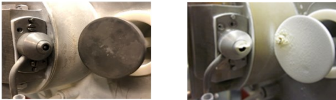
Figure S1. Baffle cone (left) before and (right) after running methylalumoxane.
