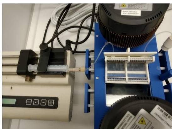
10) Set-up with opened lid before usage, with syringe pump (left) connected to the flow reactor (right).
