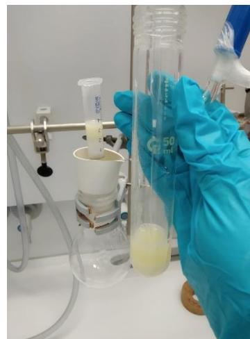
15) The reaction was filtered through a short pad of silica, washing thoroughly with ethyl acetate.
