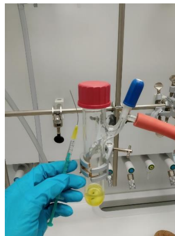
9) The bromide 1a is transferred to the vessel under argon counterflow.
