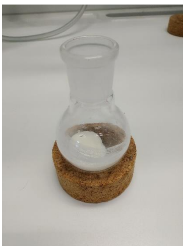
16) The solvent was removed in vacuo by rotary evaporation (40 °C) and loaded on silica.
