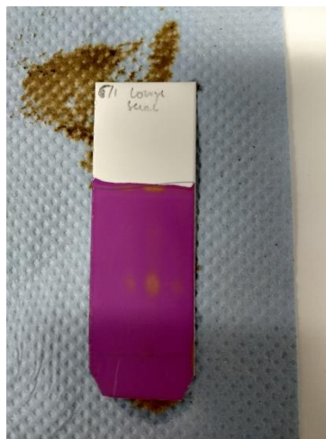
14) Thin layer chromatography ( n -pentane/EtOAc = 5/1) of the crude reaction mixture, stained with basic \text{KMnO}_4 solution.
