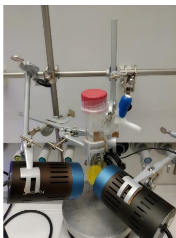
11) The reaction is placed in the photoreactor, stirring set to approximately 1000 rpm.
