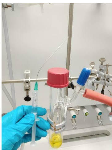
10) The solution of butadiene in THF is transferred to the vessel under argon counterflow, then the vessel is tightly sealed.
