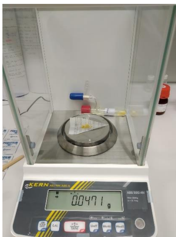
1) Nucleophile sodium p -toluenesulfinate 3a weighted under air.
