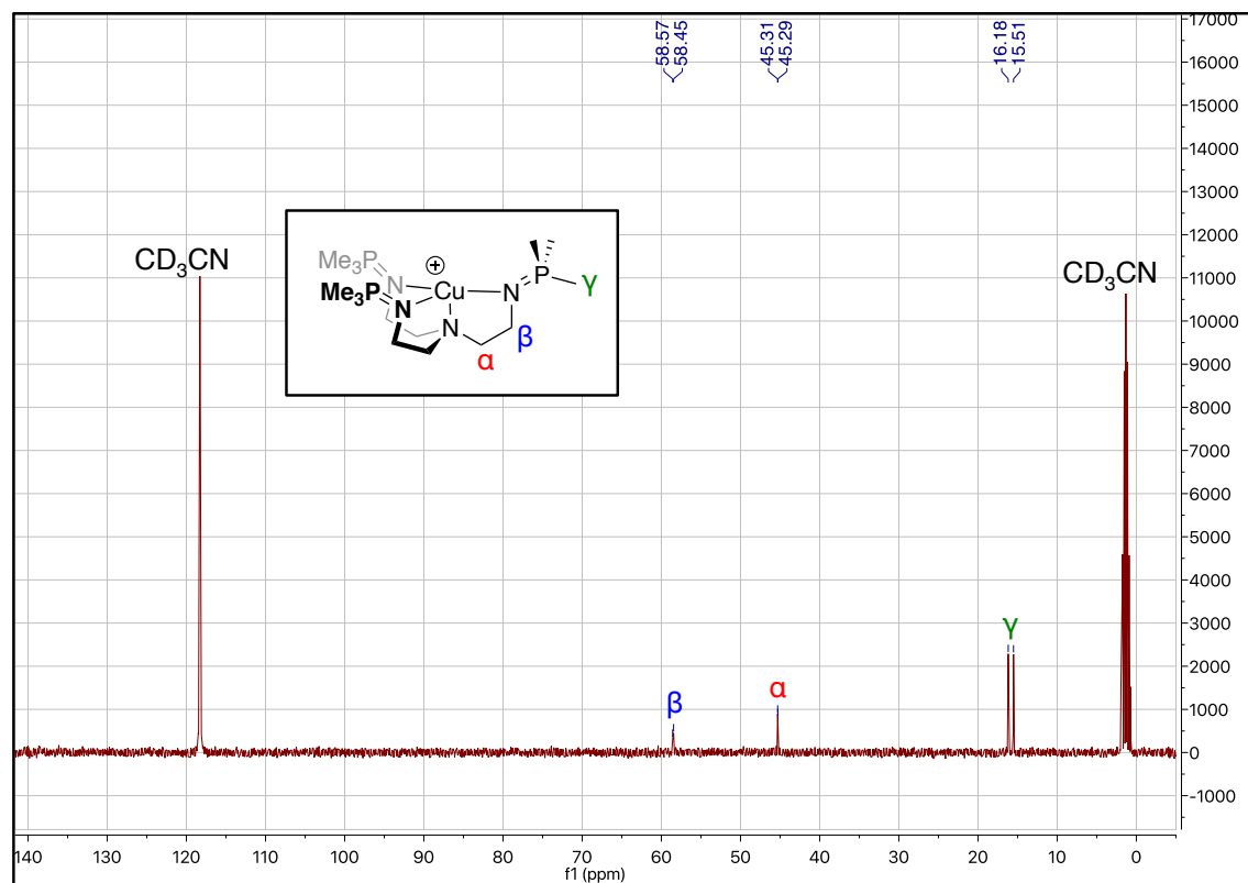
Fig S34. ^{13}\text{C}\{^1\text{H}\} NMR (101 MHz) spectrum of 1 PMe3 in \text{CD}_3\text{CN} (T = 298 K).
