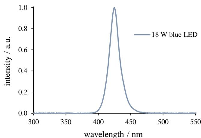
**Figure S15.** Emission spectrum of the blue LED (18 W) for quantum yield determination.
