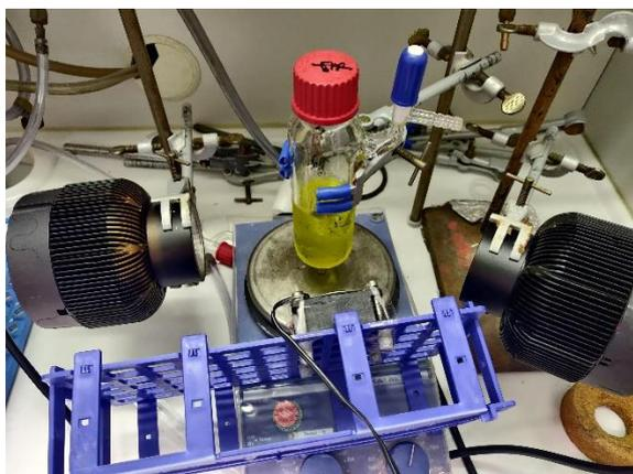
**Figure S4.** Big scale photoreaction set-up ( $d = 8$  cm) with fan cooling (entry 12).
