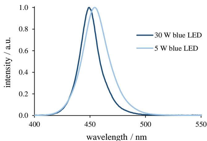
**Figure S1.** Emission spectra of EvoluChem 30 W blue LED and 5 W blue LED.
