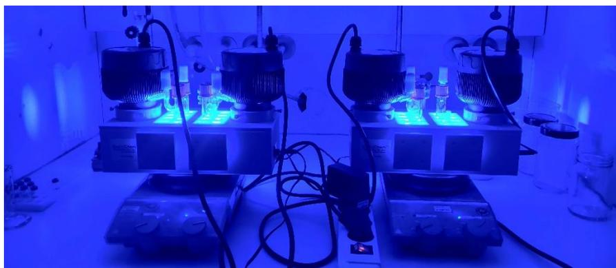
**Figure S3.** Photoreaction set-up for the sensitivity-assessment in a commercial EvoluChem™ PhotoRedOx Duo photobox (entries 1–6).
