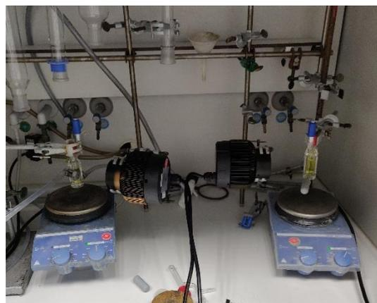
**Figure S5.** Low  $T$  photoreaction set-up with water cooling (entry 8) and control (entry 9, no water flow).
