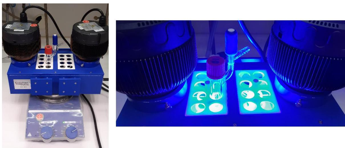
**Figure S2.** Photoreaction set-up. Commercial EvoluChem™ PhotoRedOx Duo photobox with irradiation by EvoluChem HCK1021-01-008 blue LEDs (30 W,  $\lambda_{\text{max}}$  = 450 nm).
