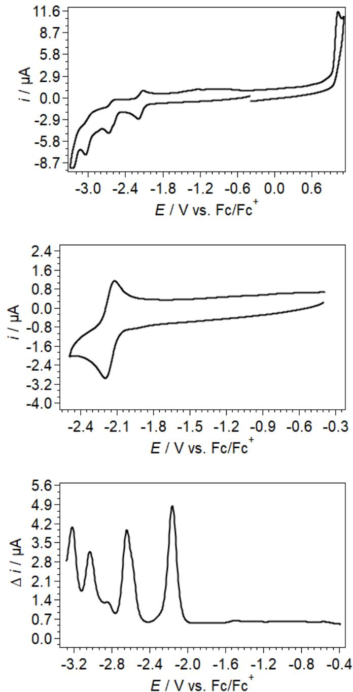
Figure S3. Overall cyclic (upper), first reduction (middle) and square-wave (bottom) voltammograms showing reduction processes of 1 mM compound **12** with 0.1 M  $n\text{Bu}_4\text{NPF}_6$ /DMF at  $0.1 \text{ V s}^{-1}$  using 1 mm diameter GC working electrode at  $298 \pm 2 \text{ K}$  in a Faraday cage.
