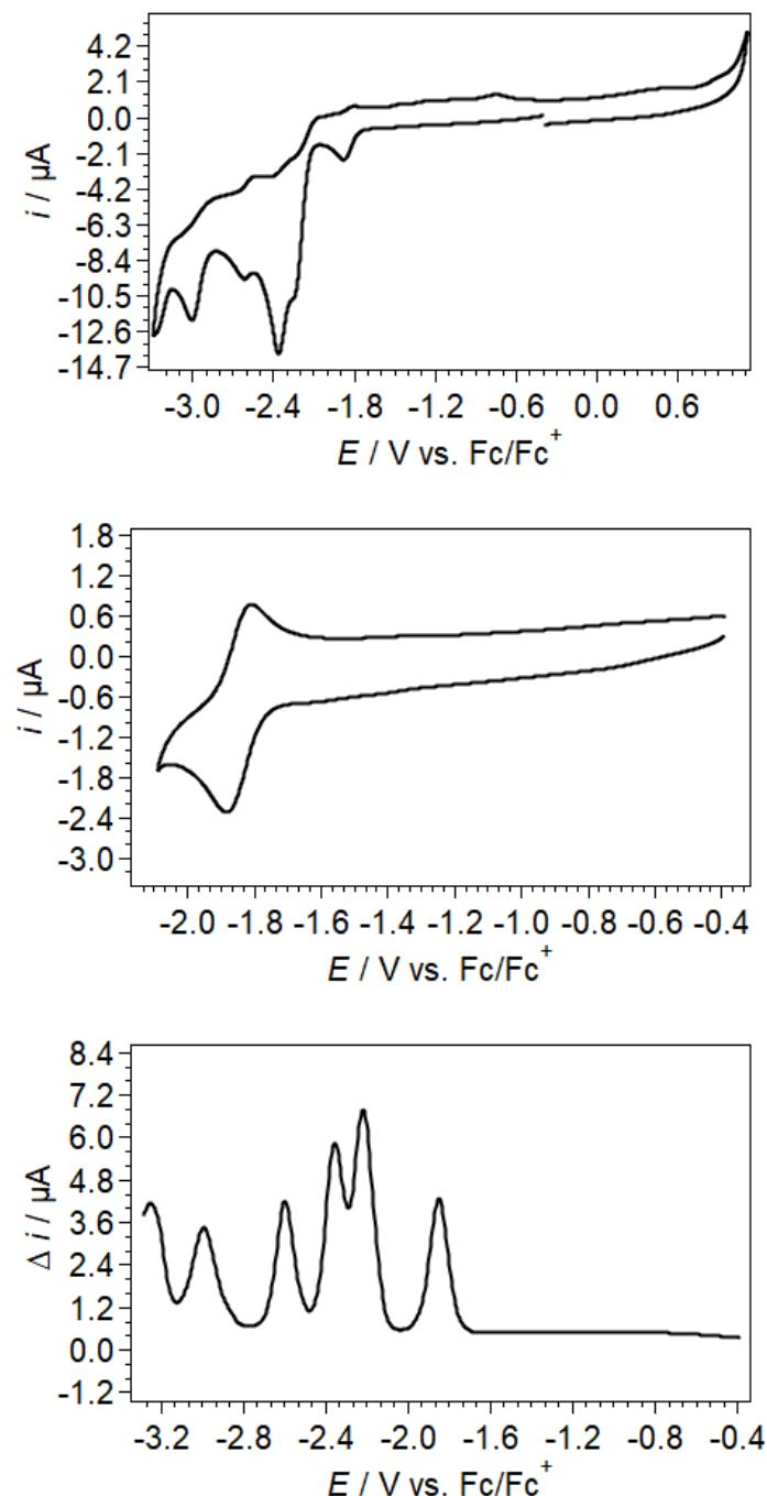
Figure S4. Overall cyclic (upper), first reduction (middle) and square-wave (bottom) voltammograms showing reduction processes of 1 mM compound **14** with 0.1 M  $n\text{Bu}_4\text{NPF}_6$ /DMF at  $0.1 \text{ V s}^{-1}$  using 1 mm diameter GC working electrode at  $298 \pm 2 \text{ K}$  in a Faraday cage.
