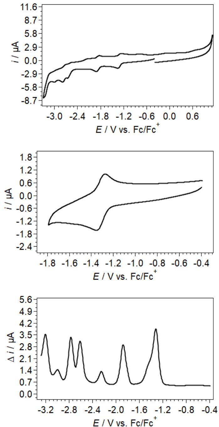
Figure S5. Overall cyclic (upper), first reduction (middle) and square-wave (bottom) voltammograms showing reduction processes of 1 mM compound **17** with 0.1 M  $n\text{Bu}_4\text{NPF}_6$ /DMF at  $0.1 \text{ V s}^{-1}$  using 1 mm diameter GC working electrode at  $298 \pm 2 \text{ K}$  in a Faraday cage.
