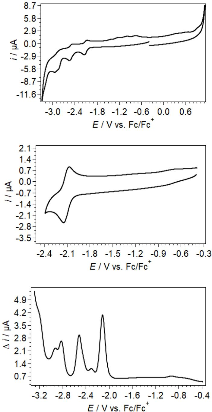
Figure S2. Overall cyclic (upper), first reduction (middle) and square-wave (bottom) voltammograms showing reduction processes of 1 mM compound **10** with 0.1 M  $n\text{Bu}_4\text{NPF}_6$ /DMF at  $0.1 \text{ V s}^{-1}$  using 1 mm diameter GC working electrode at  $298 \pm 2 \text{ K}$  in a Faraday cage.
