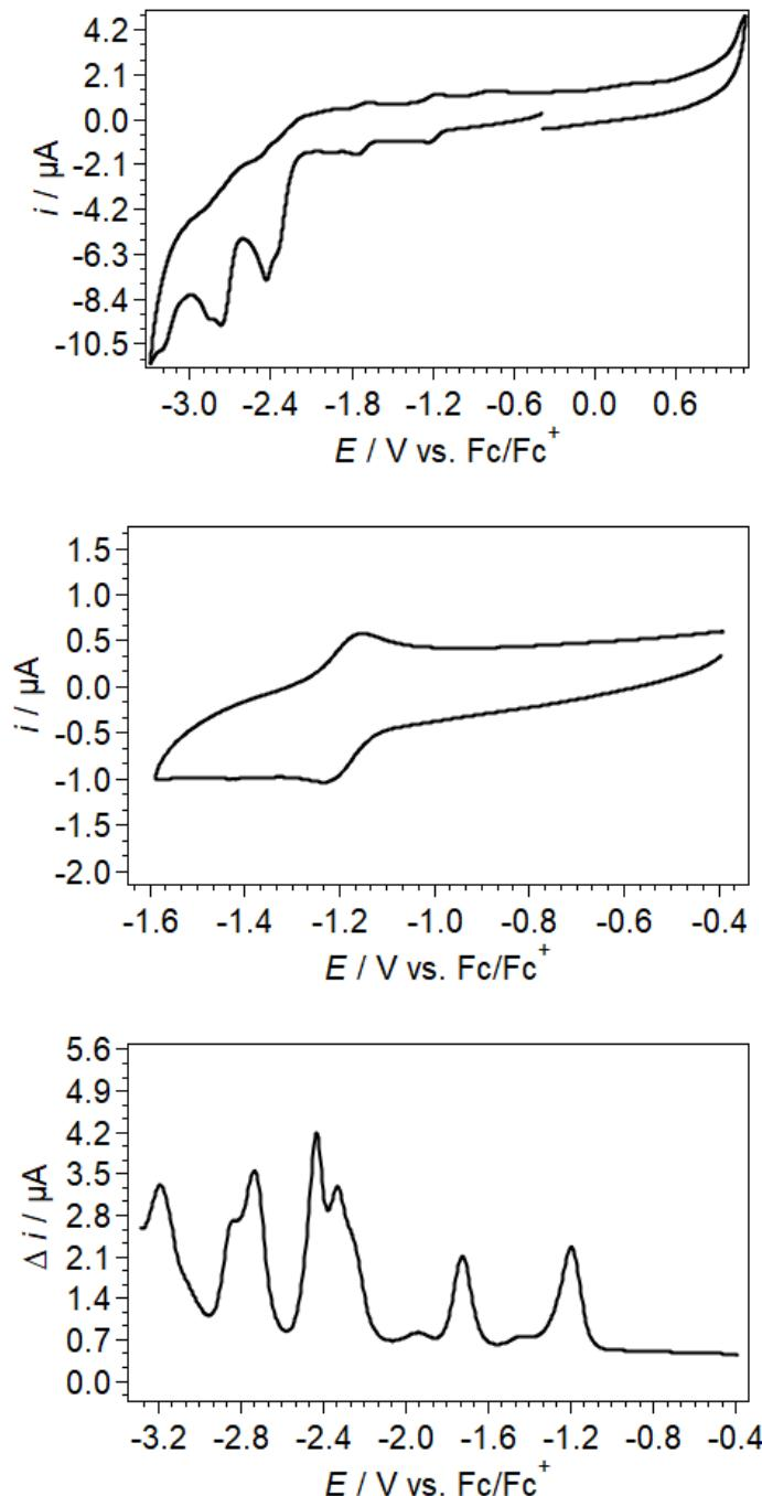
Figure S7. Overall cyclic (upper), first reduction (middle) and square-wave (bottom) voltammograms showing reduction processes of 1 mM compound **21** with 0.1 M  $n\text{Bu}_4\text{NPF}_6/\text{DMF}$  at  $0.1 \text{ V s}^{-1}$  using 1 mm diameter GC working electrode at  $298 \pm 2 \text{ K}$  in a Faraday cage.
