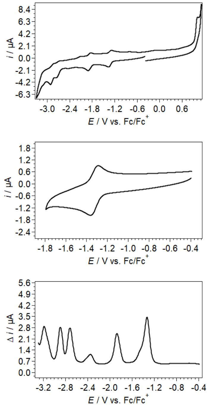
Figure S6. Overall cyclic (upper), first reduction (middle) and square-wave (bottom) voltammograms showing reduction processes of 1 mM compound **19** with 0.1 M  $n\text{Bu}_4\text{NPF}_6$ /DMF at  $0.1 \text{ V s}^{-1}$  using 1 mm diameter GC working electrode at  $298 \pm 2 \text{ K}$  in a Faraday cage.
