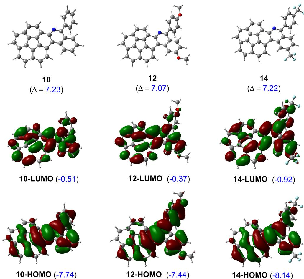
Figure S8. Frontier molecular orbitals of the single azahelienes (isovalue = 0.03). Orbital energies calculated at the  $\omega$ B97X-D/Def2TZVPP level and the HOMO-LUMO energy gaps ( $\Delta$ ) are given in parenthesis (in eV).
