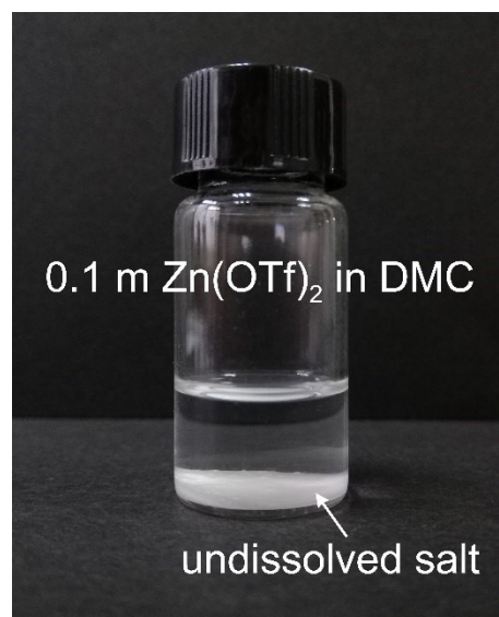
Fig. S2 Photograph of 0.1 m Zn(OTf) 2 in the neat DMC electrolyte. DMC solvent has a low solubility for Zn(OTf) 2 salt (< 0.1 m).
