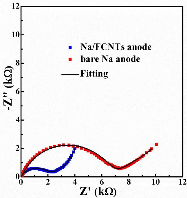
**Fig. S9.** Nyquist plots of the Na–O<sub>2</sub> cells with bare Na and Na/FCNTs anodes.
