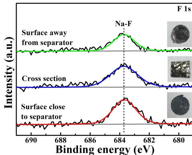
**Fig. S5.** F1s XPS spectra of the Na/FCNTs electrode surface close to separator, the cross section and the surface away from separator of Na/FCNTs electrode after 30% Na stripping at 1 mA cm<sup>-2</sup>.
