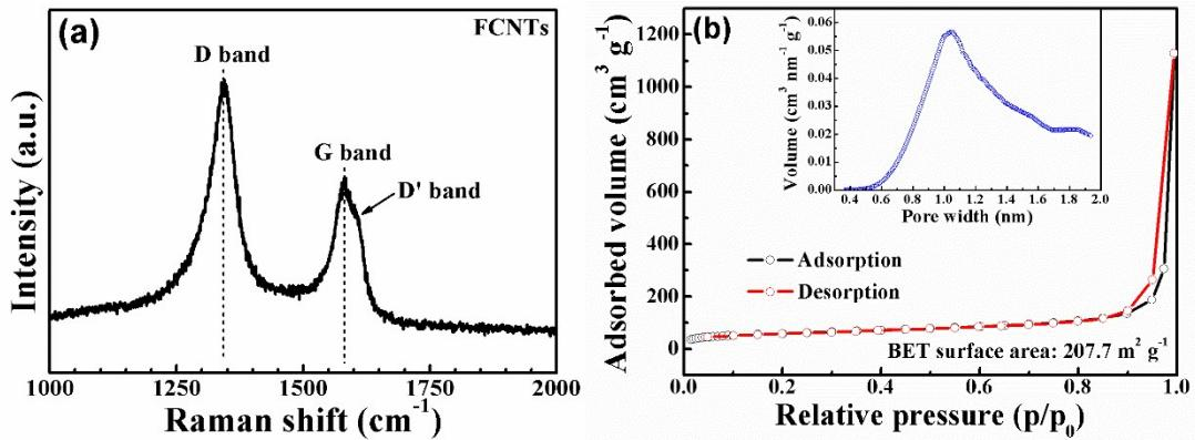
**Fig. S2.** (a) Raman spectrum of FCNTs, and (b) nitrogen adsorption/desorption isotherms and pore size distribution of FCNTs.
