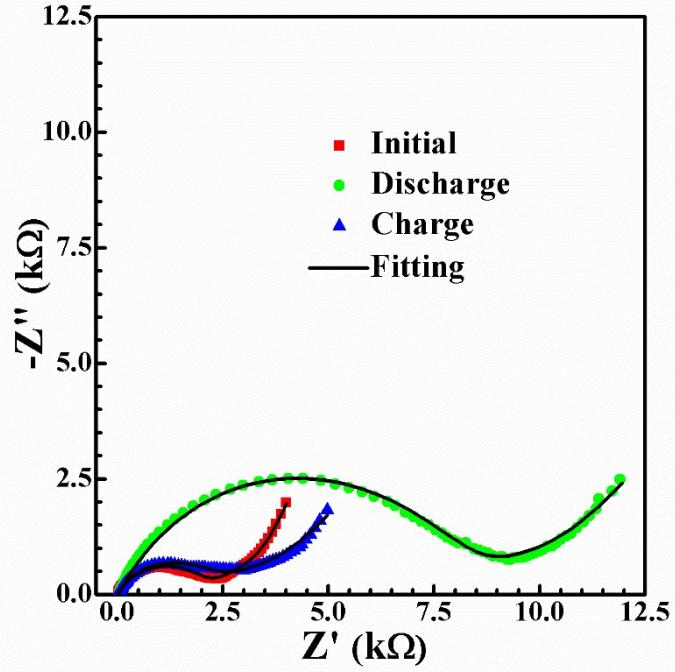
**Fig. S8.** Nyquist plots of the Na–O<sub>2</sub> cells with Na/FCNTs anode at different states.
