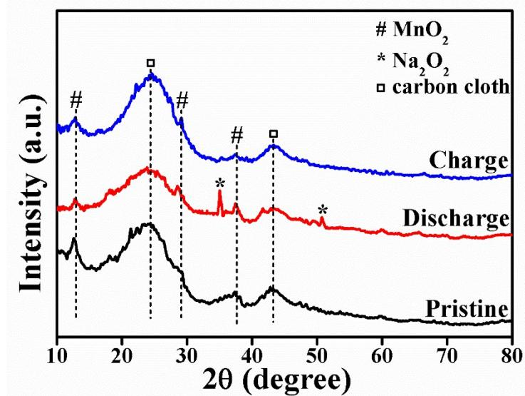
**Fig. S6.** XRD patterns of cathodes of the Na–O<sub>2</sub> cells at different states with Na/FCNTs anode.
