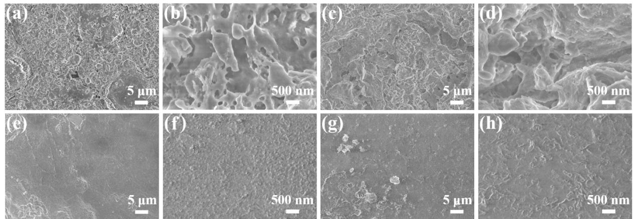
**Fig. S4.** SEM images of bare Na electrodes after (a, b) 30% and (c, d) 50% Na stripping, and SEM images of Na/FCNTs electrodes after (e, f) 30% and (g, h) 50% Na stripping at 1 mA cm<sup>-2</sup>.
