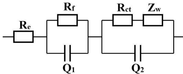
**Fig. S3.** Equivalent circuit for fitting of the Nyquist plots, where  $R_e$  represents ohm resistance of cell components,  $R_f$  and  $Q_1$  correspond to surface film resistance and relaxation capacitance,  $R_{ct}$  and  $Q_2$  represent the charge transfer resistance and double-layer capacitance, and  $Z_w$  is associated with the bulk diffusion of Na ions.
