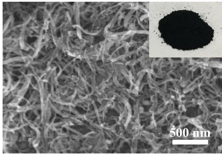
**Fig. S1.** SEM image of the commercial FCNTs.
