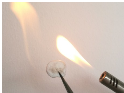
Fig. S7 | Heating experiments of GF separator soaked in TEGDME electrolyte.
